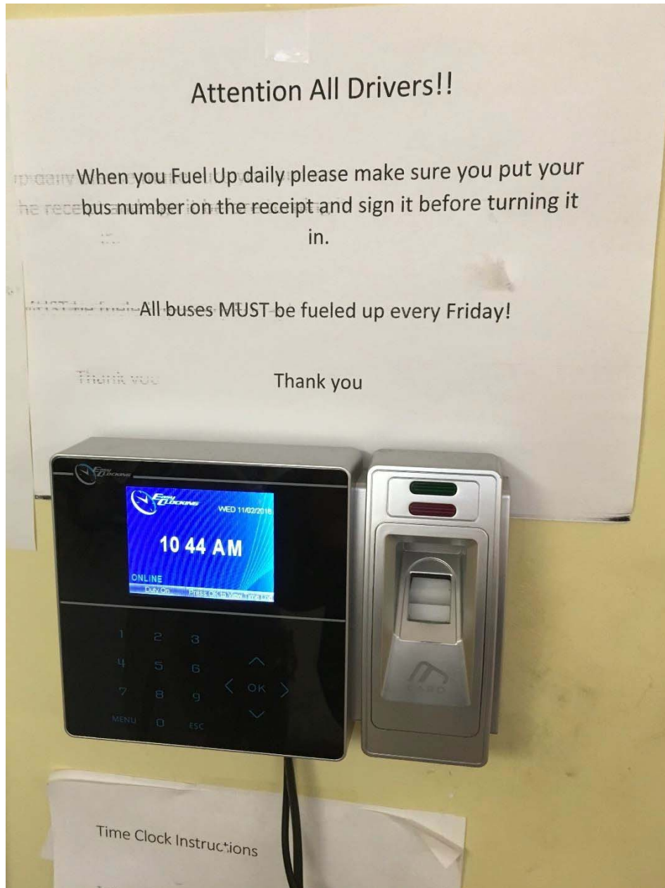
Photo 3. AAAfordable biometric time card station where drivers would use a finger to scan into the time card device to track driver's hours of service.
