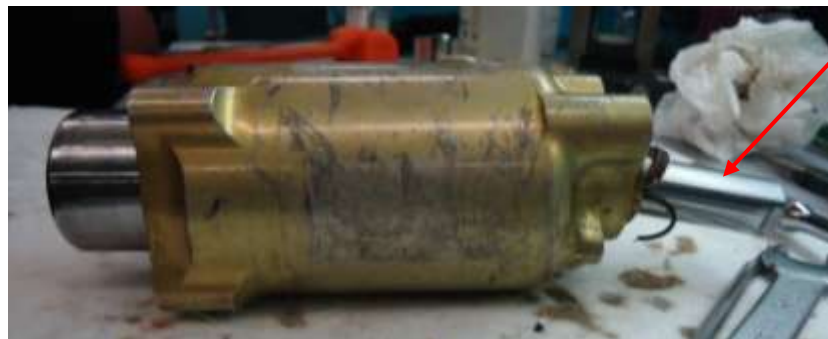
Figure 20. Actuator assembly with hydraulic extend chamber removed
