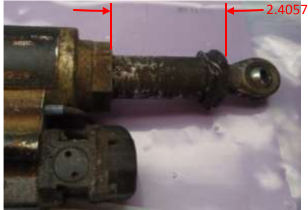
Figure 33. Residue present on actuator piston
