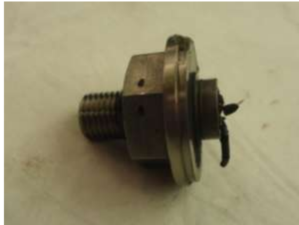
Figure 19. Remainder of nitrogen pressure transducer removed from nitrogen retract chamber
