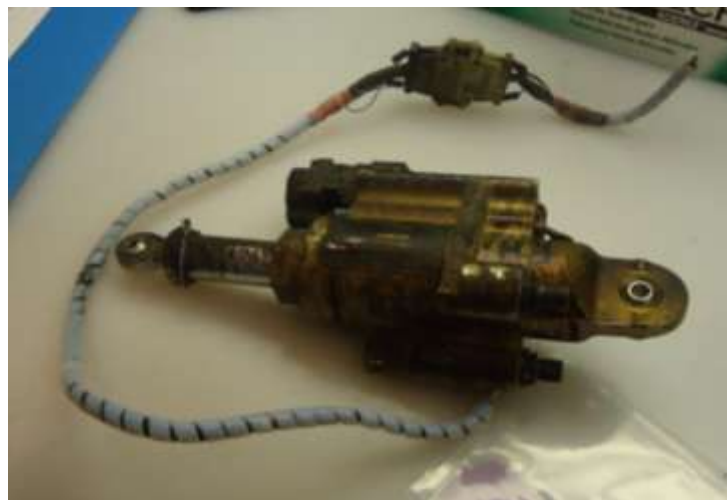
Figure 32. As received Roll Control Actuator S/N: 0469
