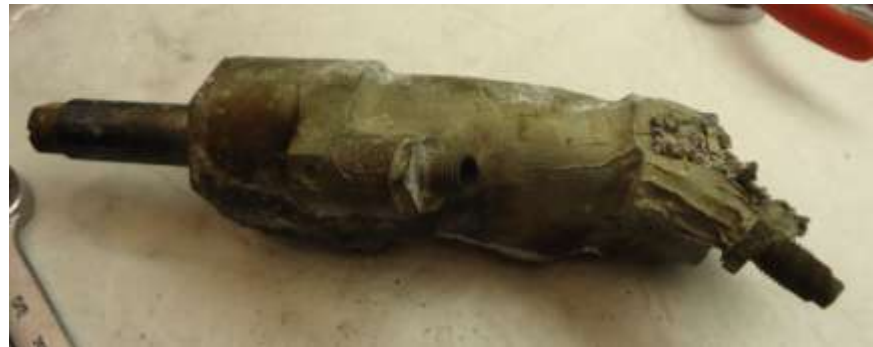
Figure 12. As received Lift Dump Actuator Unknown 2
