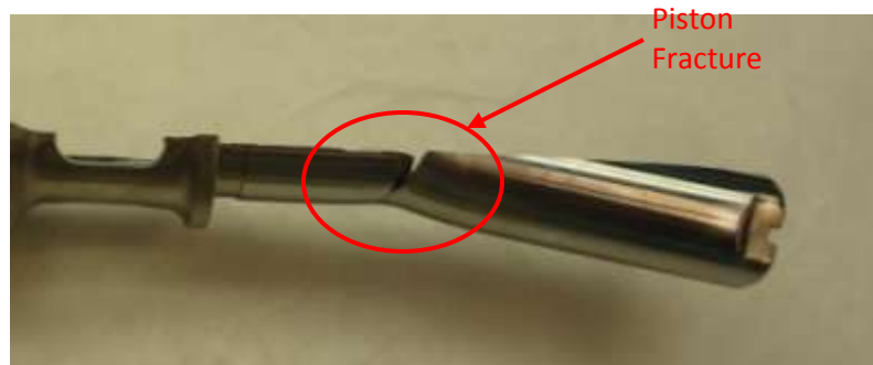
Figure 23. Sectioned actuator piston, rotated to show fracture
