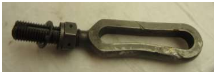
Figure 18a. Deformed clevis removed from end of piston with gouges present
