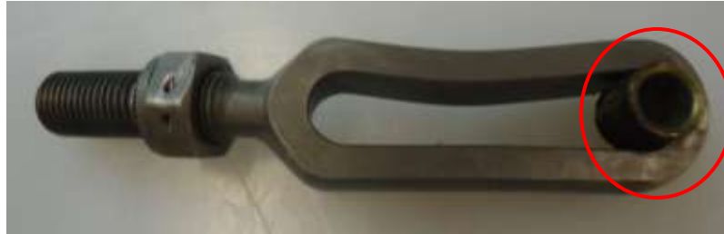
Figure 18b. Deformed clevis with aircraft bushing installed in outboard end.
