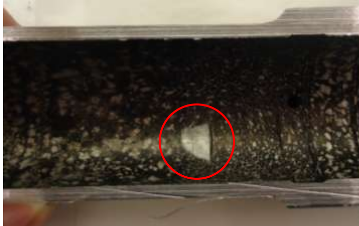
Figure 7. Sectioned manifold – Half 2. Burr and "scuff" mark present.
