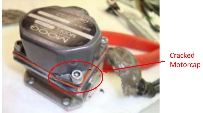
Figure 28. Cracked servovalve motorcap
