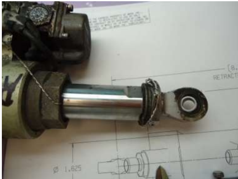
Figure 34. Residue removed from piston prior to evaluation testing
