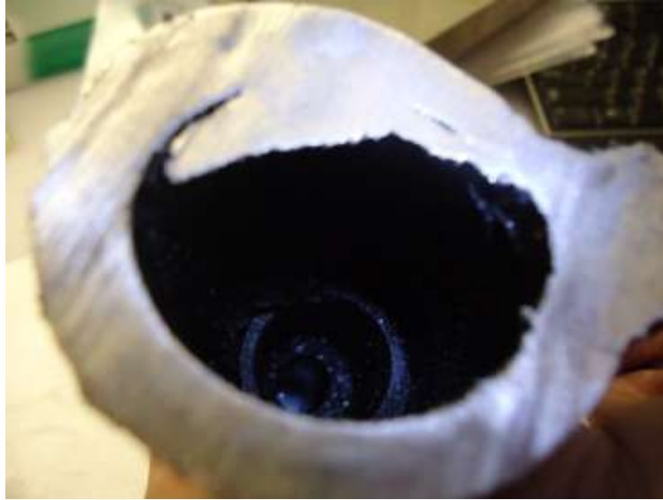
Figure 13. Cylinder bore of manifold after sectioning lug end
