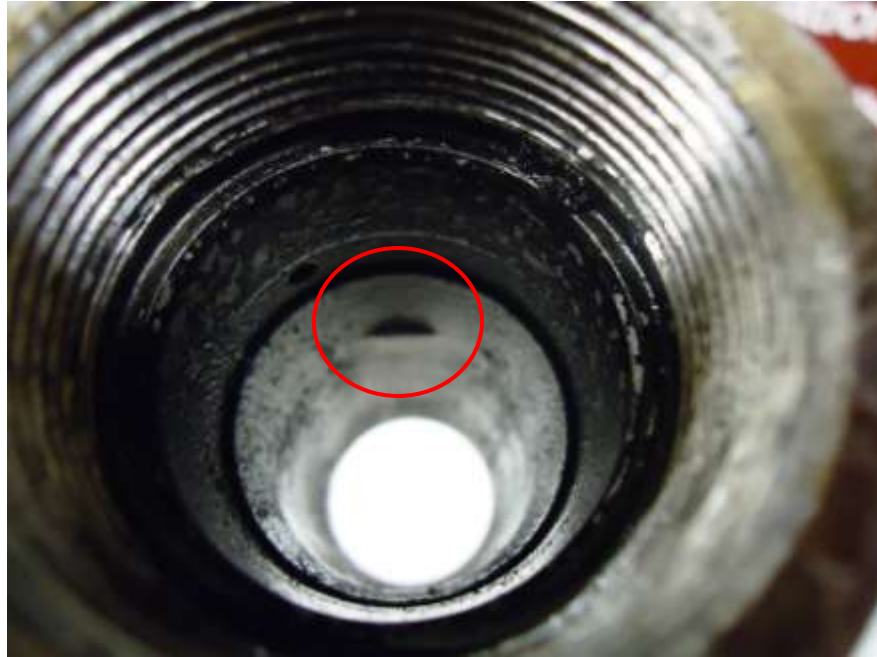
Figure 5. Burr (circled in red) observed preventing piston from being removed through the bore mouth
