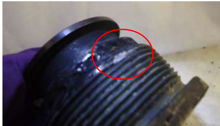
Figure 10. Damaged thread on piston gland (circled in red)
