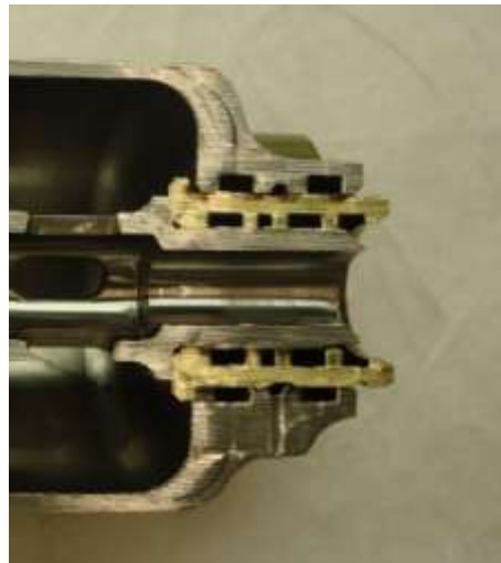
Figure 24. Sectioned actuator assembly in fully extended position
