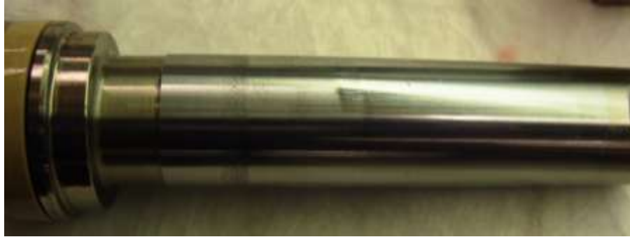
Figure 29. Actuator piston with normal signs of wear
