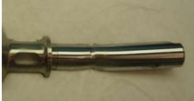
Figure 22. Sectioned actuator piston
