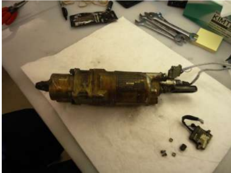
Figure 25. As received Blow Down Actuator S/N: 0459
