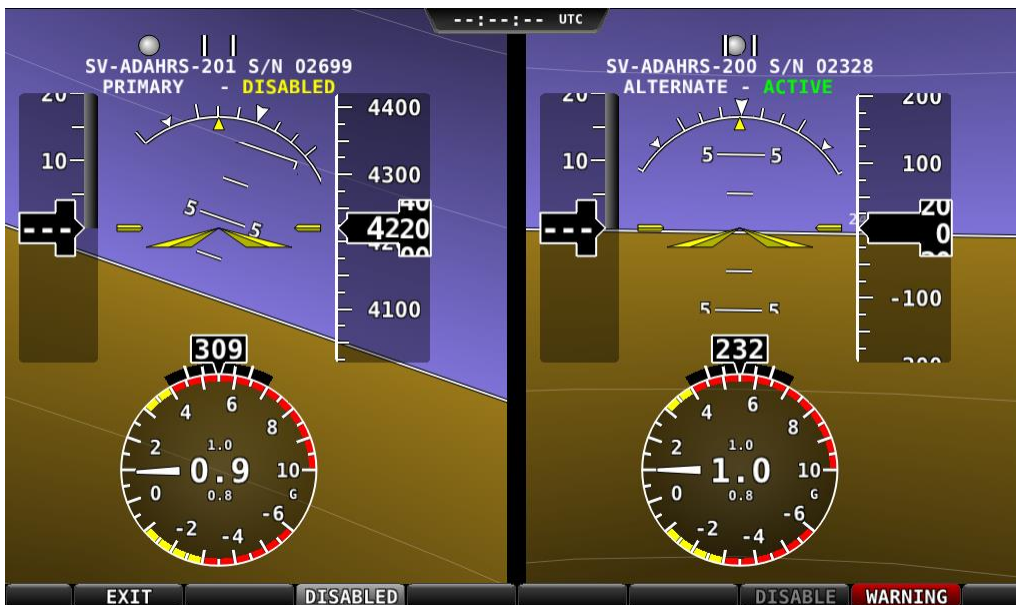
Figure 56 - ADAHRS Cross-Check Comparison (one ADAHRS disabled)
