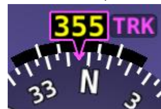
Figure 23 - GPS Track substitute for Magnetic Heading
