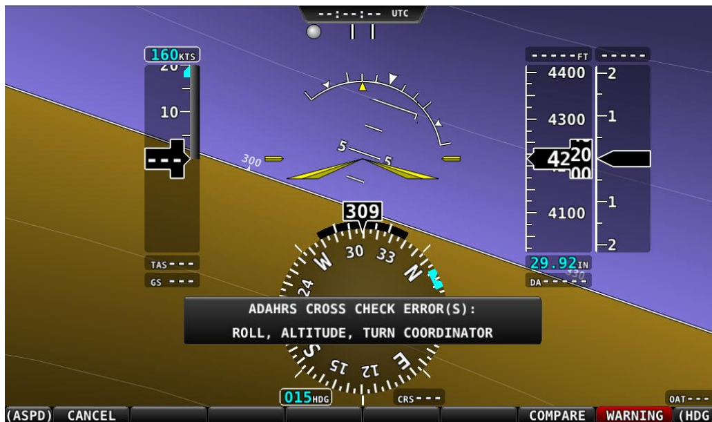
Figure 54 - ADAHRS Cross-Checking Disagreement
