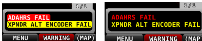
Figure 228–Unacknowledged (left) and Acknowledged (right) Alarms
