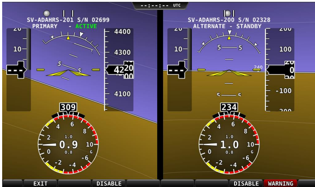
Figure 55 - ADAHRS Cross-Check Comparison
