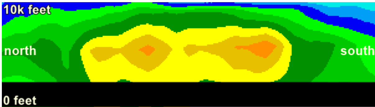
Figure 7 – North-south 0-10,000 feet (approximate) vertical cross-section of the Level-II reflectivity product from the volume scan initiated at 2233:08 AKDT through the cell adjacent to and to the east of the accident site. Color table is as presented in figures 2-6.
