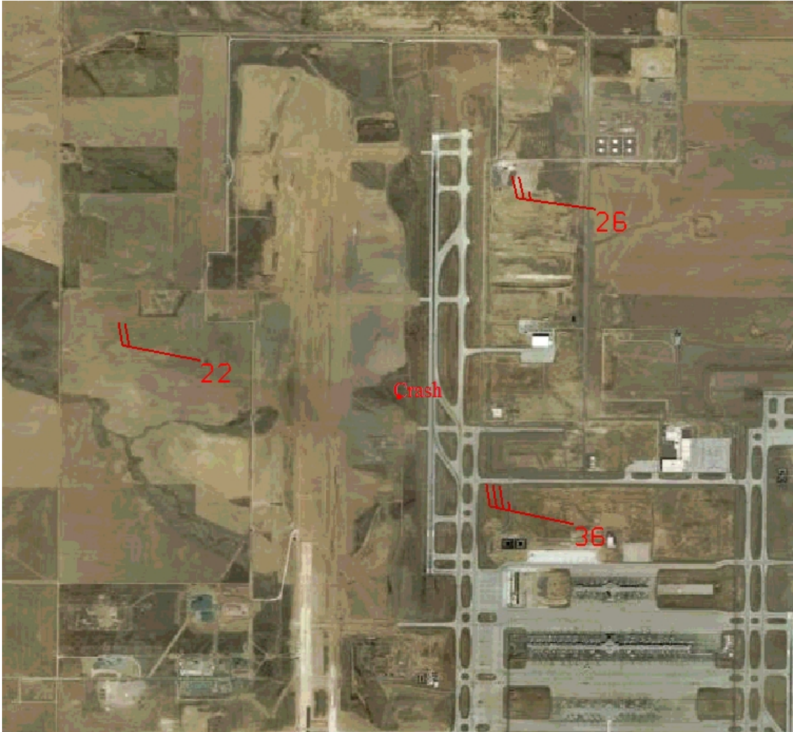
Figure 8: Plot of LLWAS wind sensor data over an image of KDEN showing runway 34R for December 20, 2008, at 1818:32 MST (December 21, 2008, at 0118:32Z). Wind barbs indicate the direction the wind is coming from. Each full barb equals 10 knots and each short barb equals 5 knots. Wind speeds in knots are noted at the head of the wind barbs. The crash site is plotted on the image. True north is to the top of the image. Runway 16R/34L is not shown in the image. The data were plotted using the IDV.
