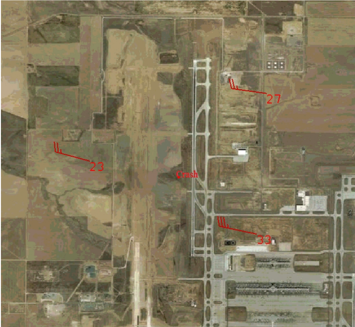
Figure 7: Plot of LLWAS wind sensor data over an image of KDEN showing runway 34R for December 20, 2008, at 1817:32 MST (December 21, 2008, at 0117:32Z). Wind barbs indicate the direction the wind is coming from. Each full barb equals 10 knots and each short barb equals 5 knots. Wind speeds in knots are noted at the head of the wind barbs. The crash site is plotted on the image. True north is to the top of the image. Runway 16R/34L is not shown in the image. The data were plotted using the Integrated Data Viewer (IDV). For information on the IDV see the link: IDV .
