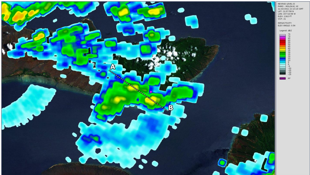
Figure 14 – PHMO 0.54° elevation base reflectivity image from 1213 HST. Pink dot denotes accident location. Dotted line corresponds to section taken for vertical slice in figure 17.
