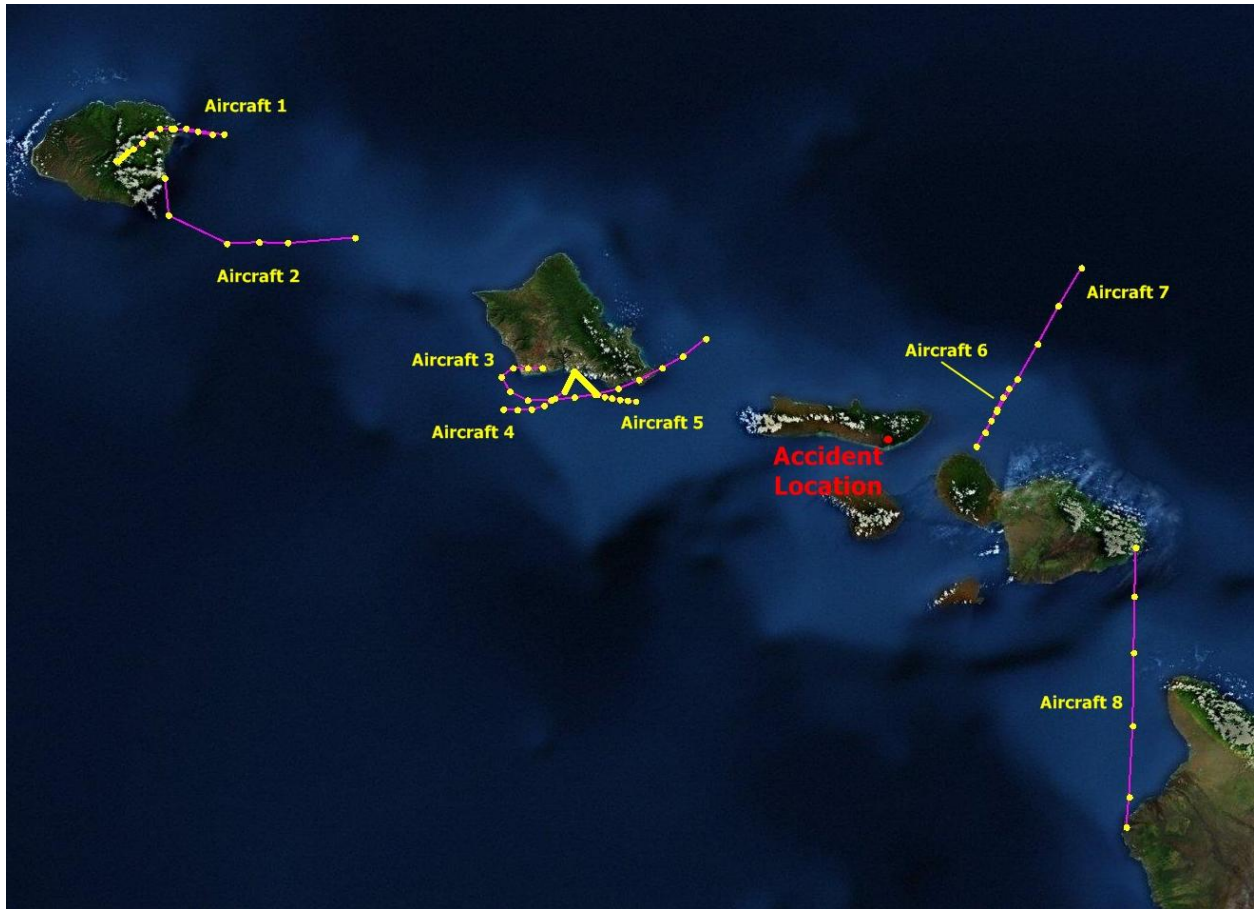
Figure 10 – Flight paths (pink lines) below about 10,000 feet for AMDAR-reporting aircraft. Yellow dots indicate reporting points.
