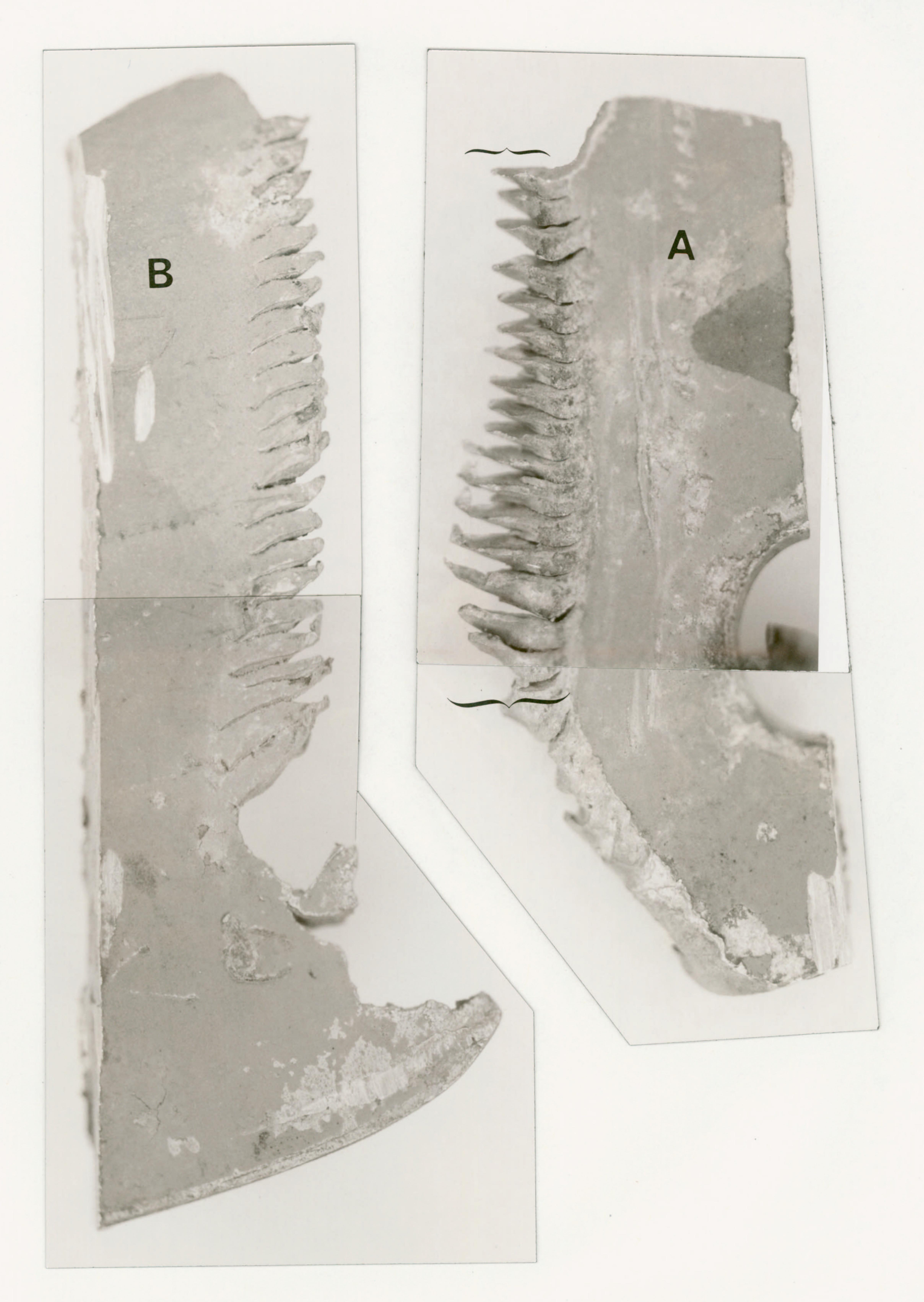
Figure 2b. Exterior surface of the spike tooth area on the landing light surround structure. The brackets indicate the extent of the rubbing damage area. (5X)
