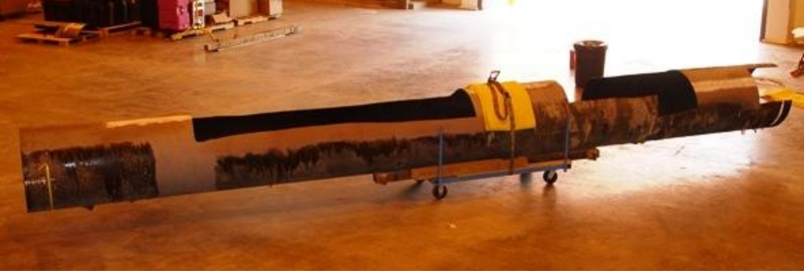
Metallurgical Group-Picture 19 Ruptured pipe piece showing areas where samples have been cut at the NTSB Ashburn, Virginia Facility
