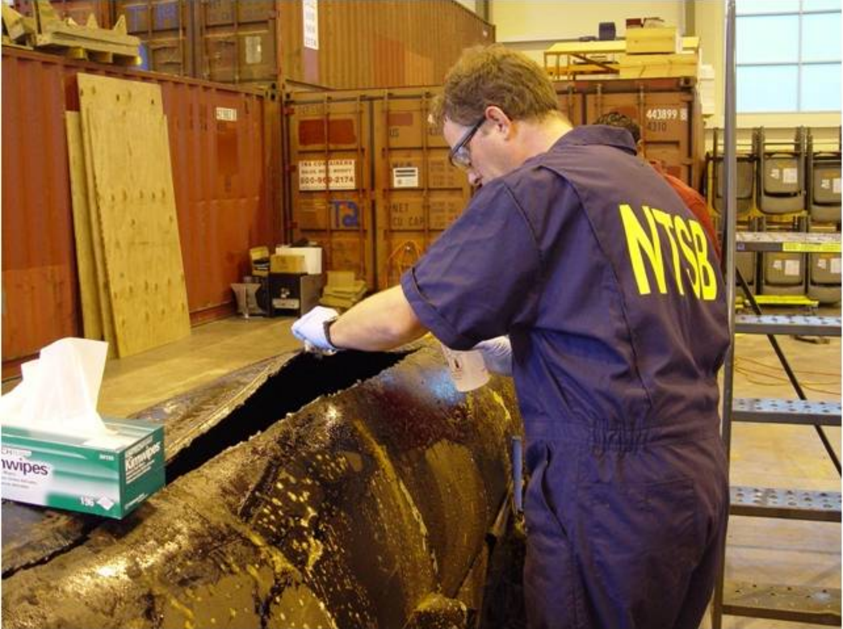
Metallurgical Group-Picture 14 Cleaning the Fracture Faces of the Ruptured Section of pipe (piece B) at the NTSB Ashburn, Virginia Facility.
