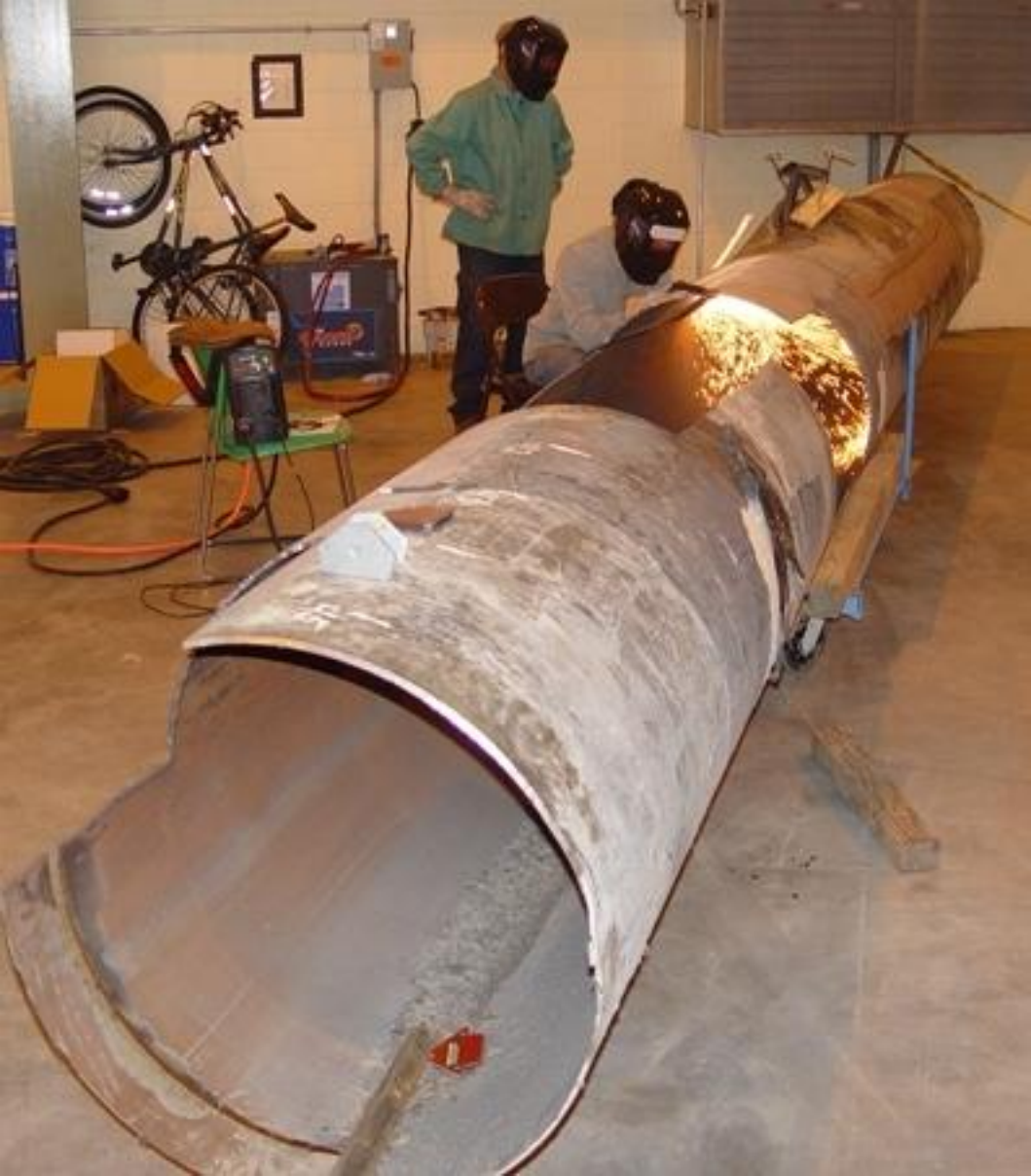
Metallurgical Group--Picture 18 Sample sections are cut from the ruptured pipe piece at the NTSB Ashburn, Virginia Facility
