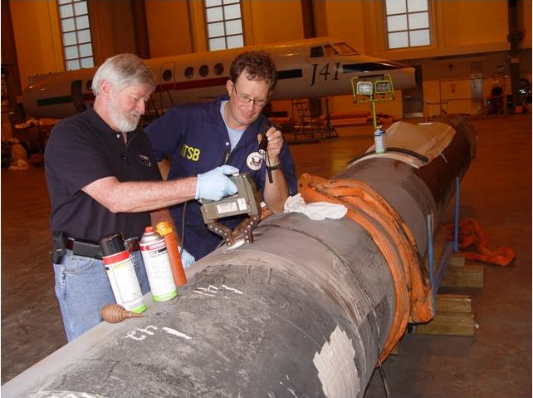
Metallurgical Group- Picture 17 Magnetic Particle Inspection (MPI) testing is performed by a qualified technician on (piece b) after grit blasting of the external surfaces at the NTSB Ashburn, Virginia facility.
