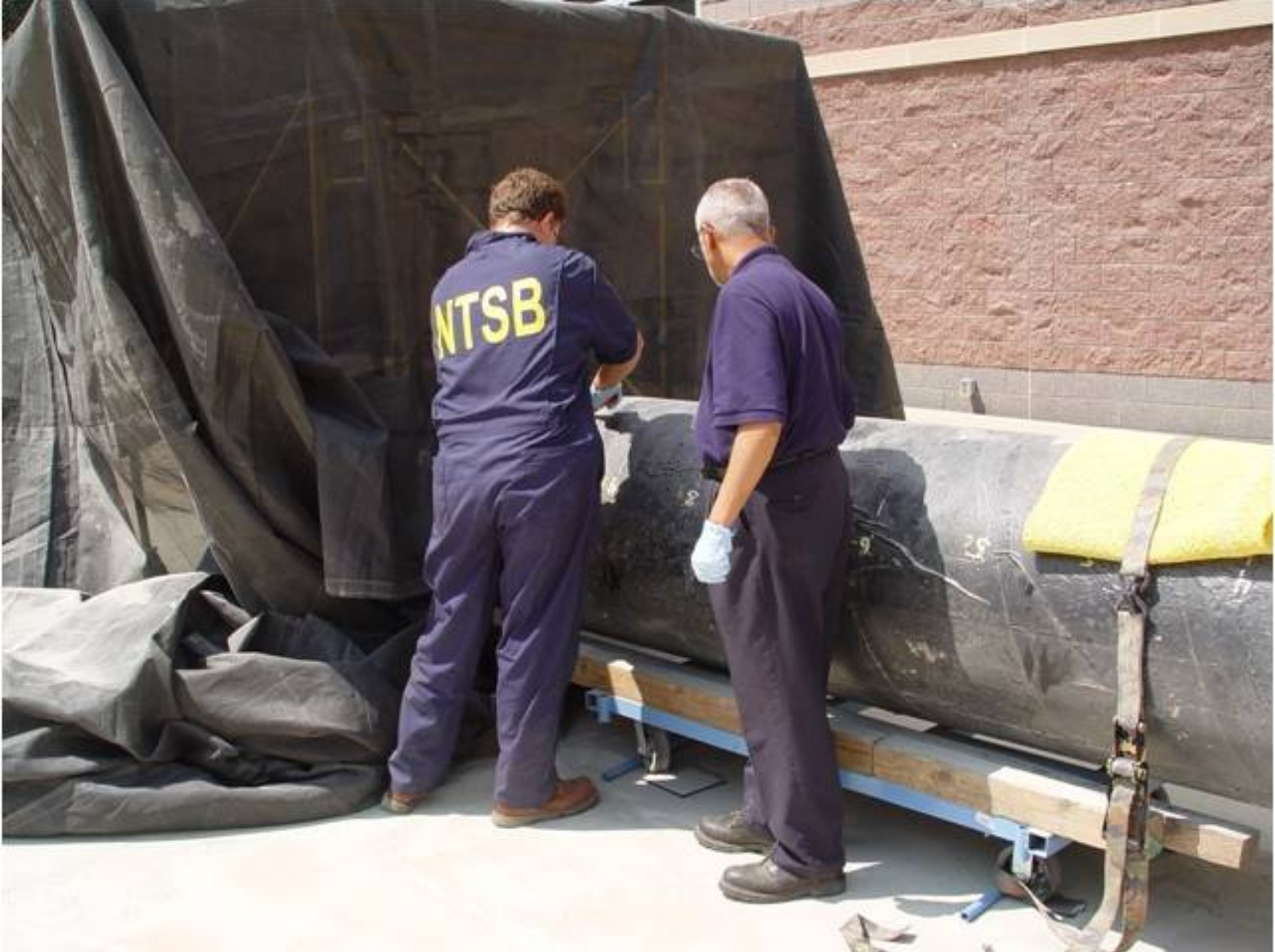
Metallurgical Group- Picture 16 Metallurgical team members inspect the finish from early grit blasting of the ruptured pipe (piece b) at the NTSB Ashburn, Virginia facility.
