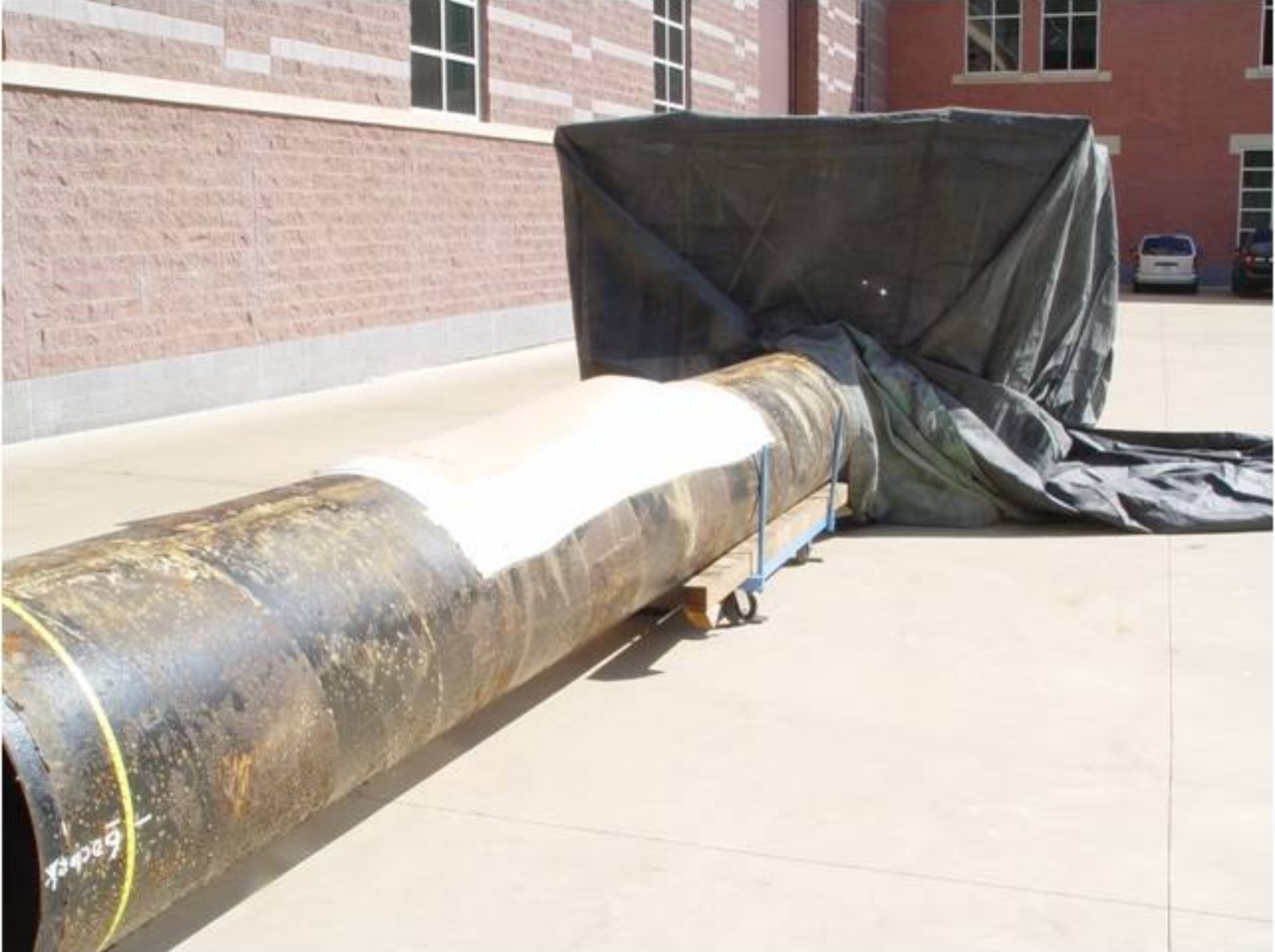
Metallurgical Group- Picture 15 Masked fracture faces and adjacent surfaces during grit blasting at the NTSB Ashburn, Virginia facility.
