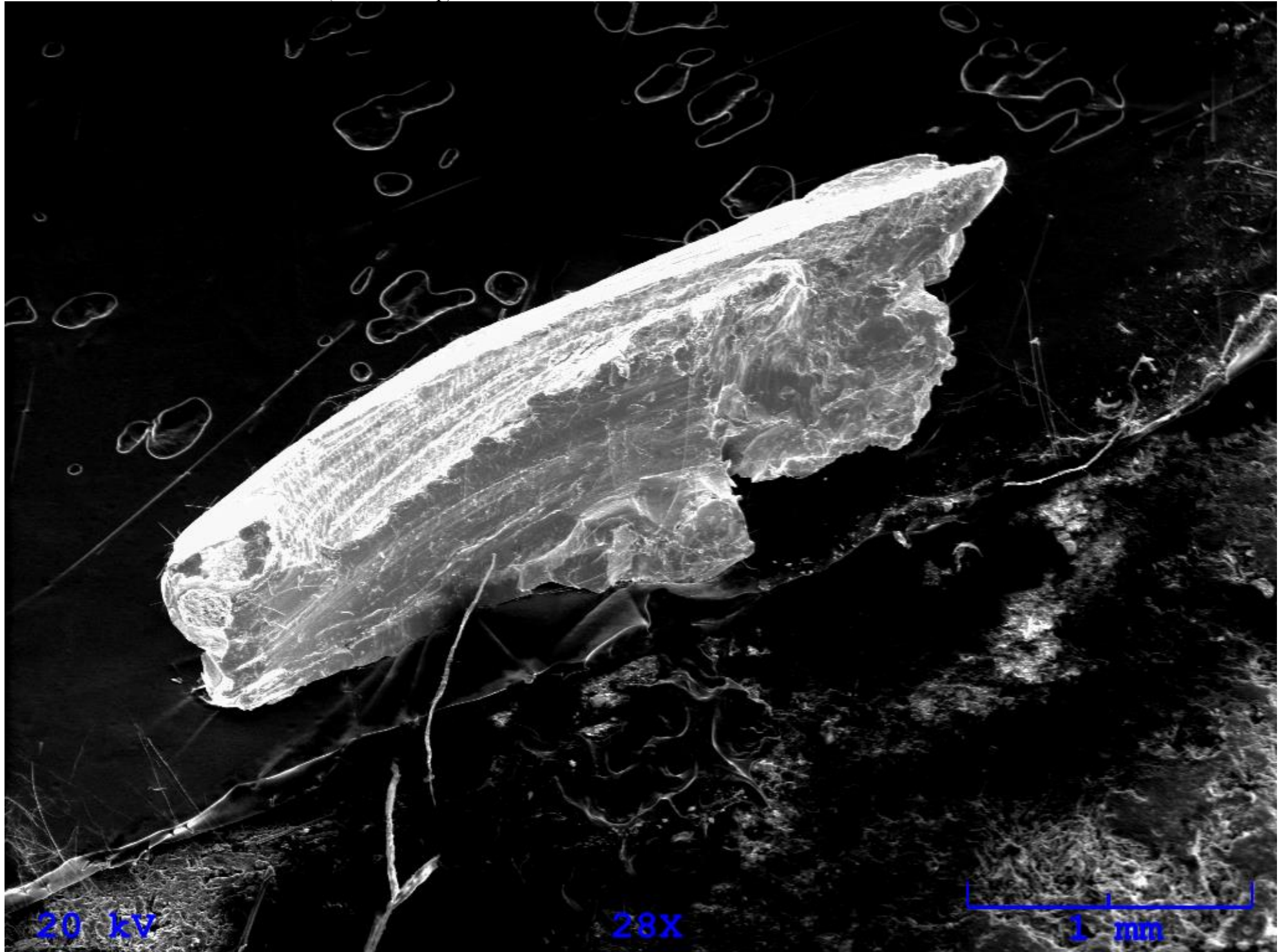
DIRECTIONAL CONTROL VALVE (Metallic Chip)
