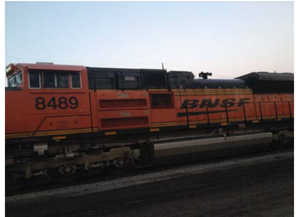
Photo #4 Locomotive BNSF 8489 Side view of locomotive indicating horn position mid-vehicle
