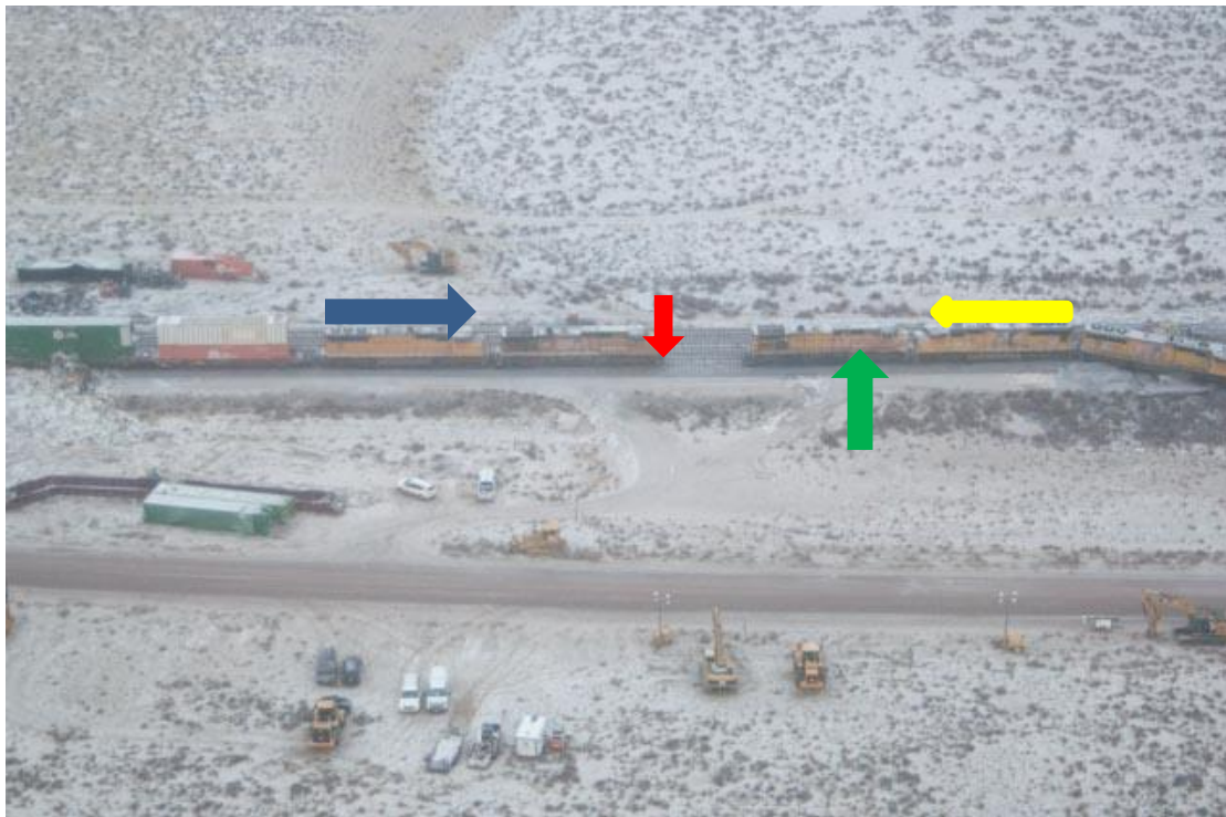
26 27 Figure 1. This is an aerial view on March 15, 2016, looking south at the derailment area. The red downward arrow 28 identifies the point of collision (impact); the yellow arrow shows the position and EB direction of travel of the stopped 29 local train, LCK41; the blue arrow identifies the WB direction of travel of the striking train; the green upward arrow 30 identifies the “as found” position of the locomotives. Note: the striking moved the stopped train about 118’ west.
