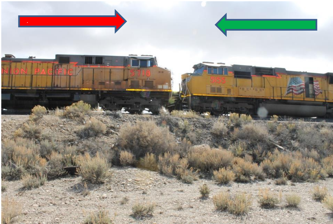
1 2 Figure 3. Collision/impact of lead locomotives. The intermodal train lead locomotive is shown below the 3 red arrow indicating the eastbound direction of travel. The lead locomotive for the coal train is shown below 4 the green arrow indicating the westbound direction of travel. 5 6
