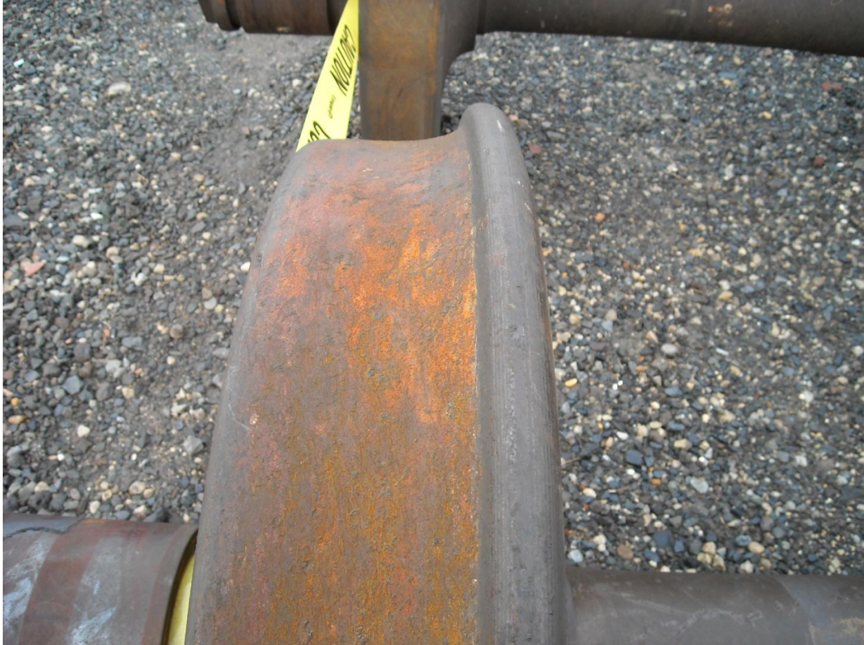
Figure 8 Typical recovered wheel profile.
