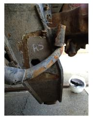
Figure 6 Cab car right side pilot assembly attachment.
