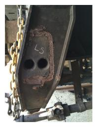
Figure 4 Cab car left side pilot assembly attachment.
