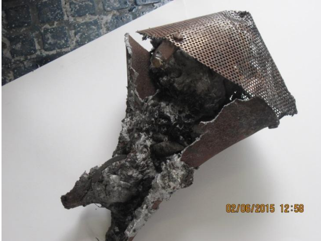
Figure 1 Horn from lead car 4333 destroyed in the fire.
