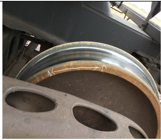
Figure 4-TCBX 198115 wheel damage. (Photo FRA)
