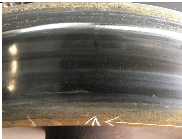
Figure 6- TCBX 198115 wheel damage (Photo FRA)
