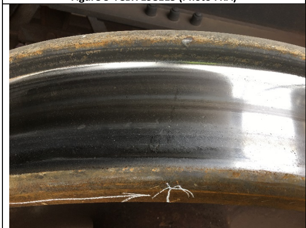
Figure 5- TCBX 198115 wheel damage (Photo FRA)
