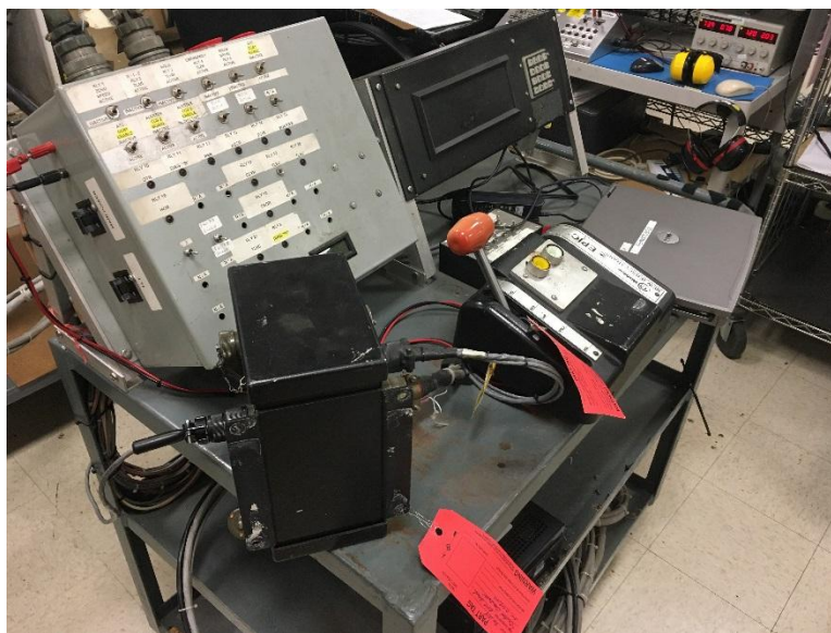
Figure 3-Photograph of test set up of the EPIC II brake components
