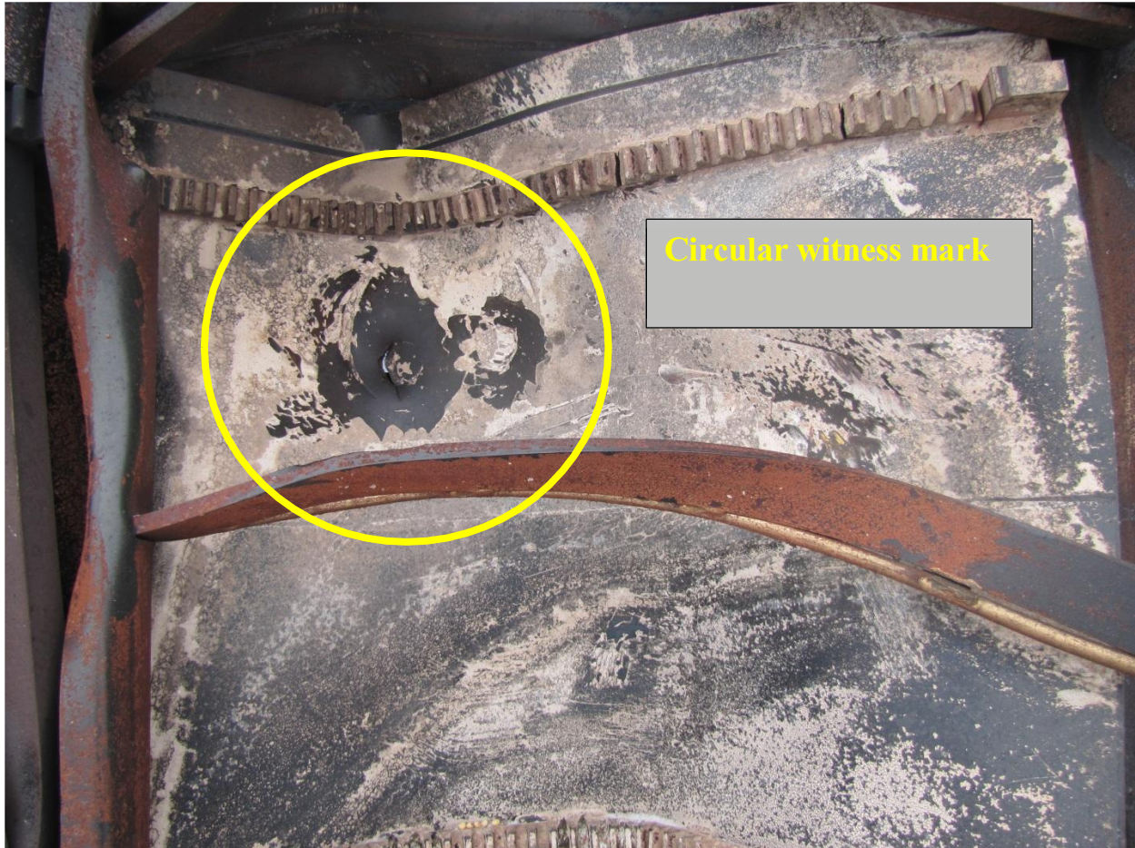
Figure 7-BNSF 486653, the 45th Car With 8-Inch Diameter Circular Witness Mark
