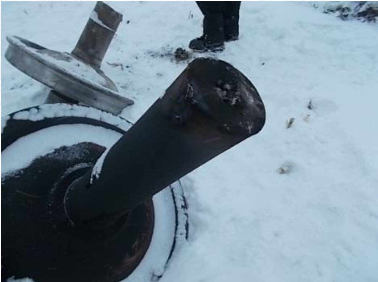
Figure 12-Broken Axle Assembly; Serial number SSD 1102 7A1 E 0912 F
