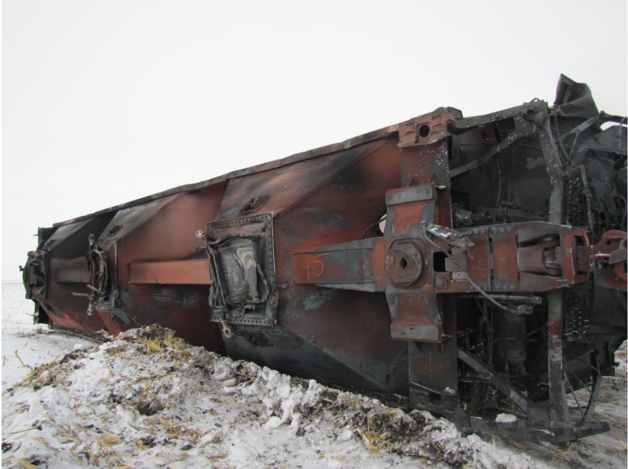
Figure 6-BNSF 486653, the 45th Car With bottom Outlet Gate Damage
