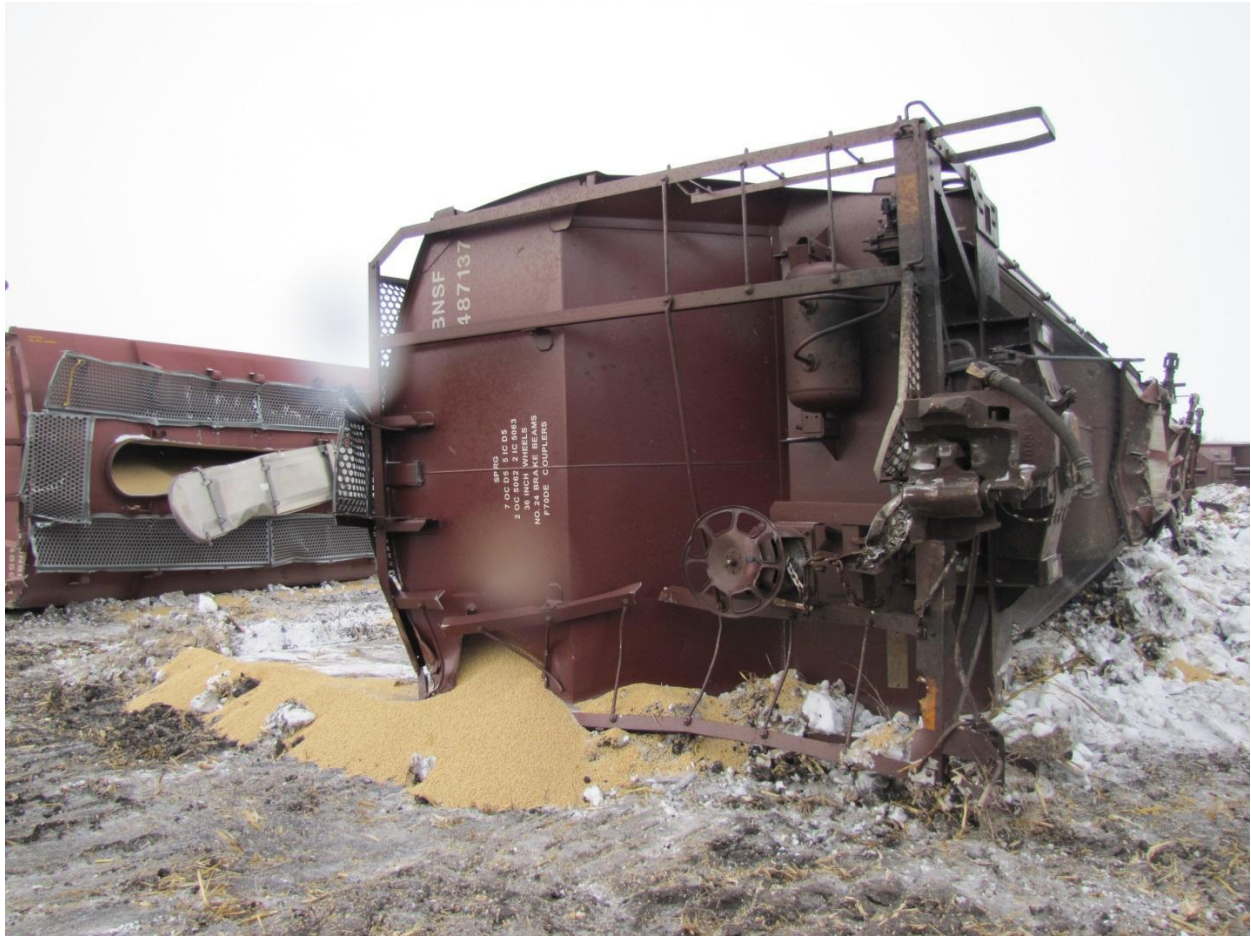
Figure 9-BNSF 487137, the 46th Car Showing the Leading End Relatively Undamaged
