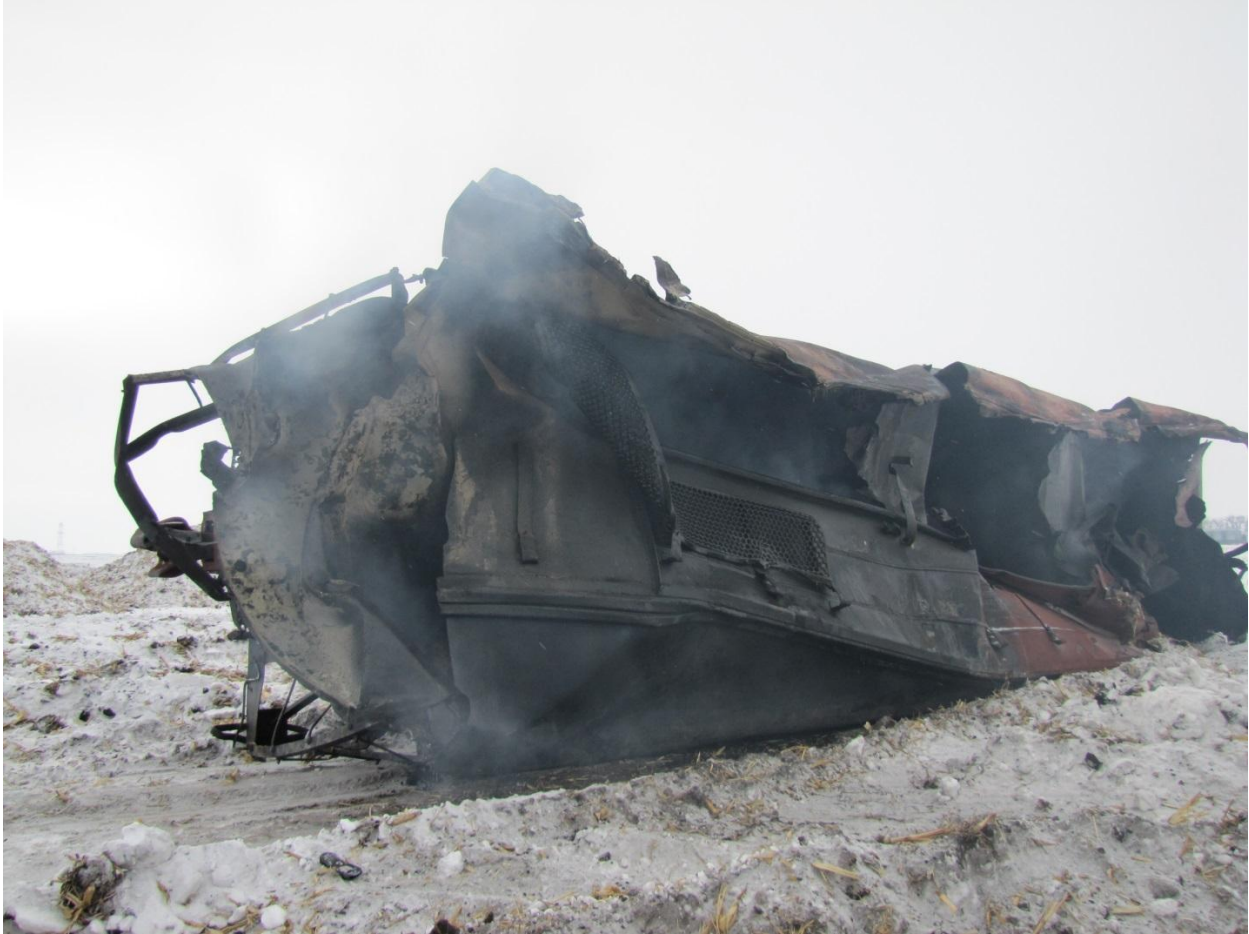
Figure 8-Figure 6-BNSF 486653, the 45th Car Showing Car Damage on the Top of the Car
