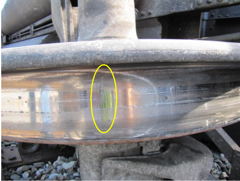
Figure 3-Photograph of Witness Mark on CSXT 398511, Wheel R4
