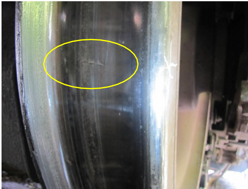
Figure 2-Photograph of Witness Mark on CSXT 4579, Wheel R1
