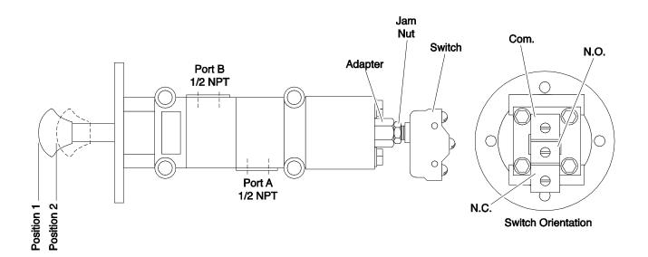
Figure 1 - "D" PILOTAIR Valve Assembly View
