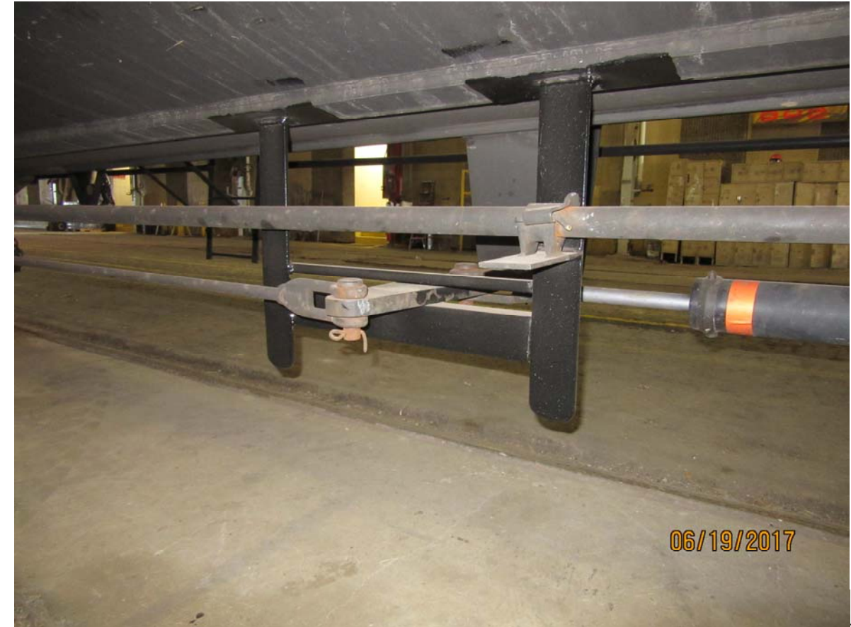
Figure 4263: TILX 198364, slack adjuster and mechanical linkages
