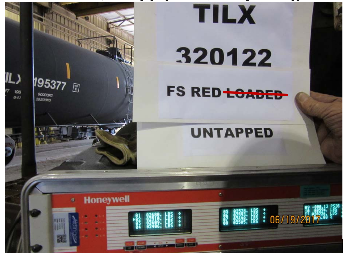
Figure 4334: TILX 320122, full service BPP reduction, car empty/loaded brake shoe forces, brake pins untapped
