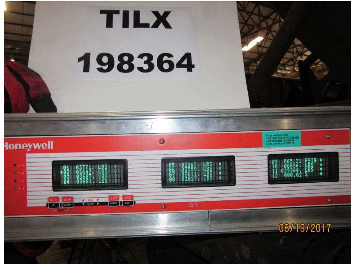
Figure 4305: TILX 198364, full service BPP reduction, loaded car, brake shoe forces, brake pins tapped (Figure 4304 backup)
