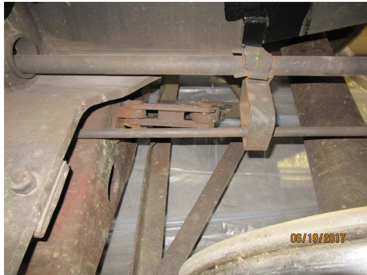
Figure 4268: TILX 198364, brake beam, pins, and mechanical linkages
