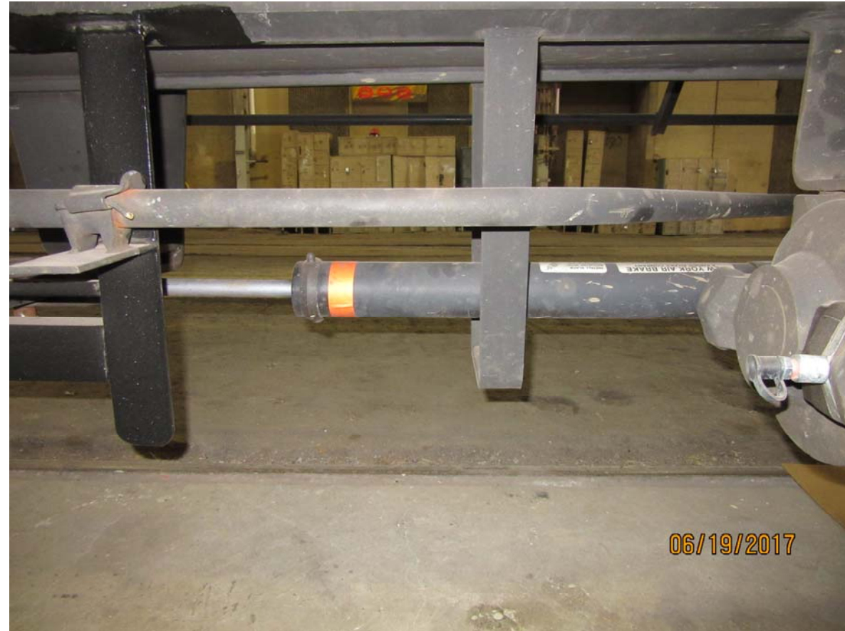
Figure 4262: TILX 198364, slack adjuster
