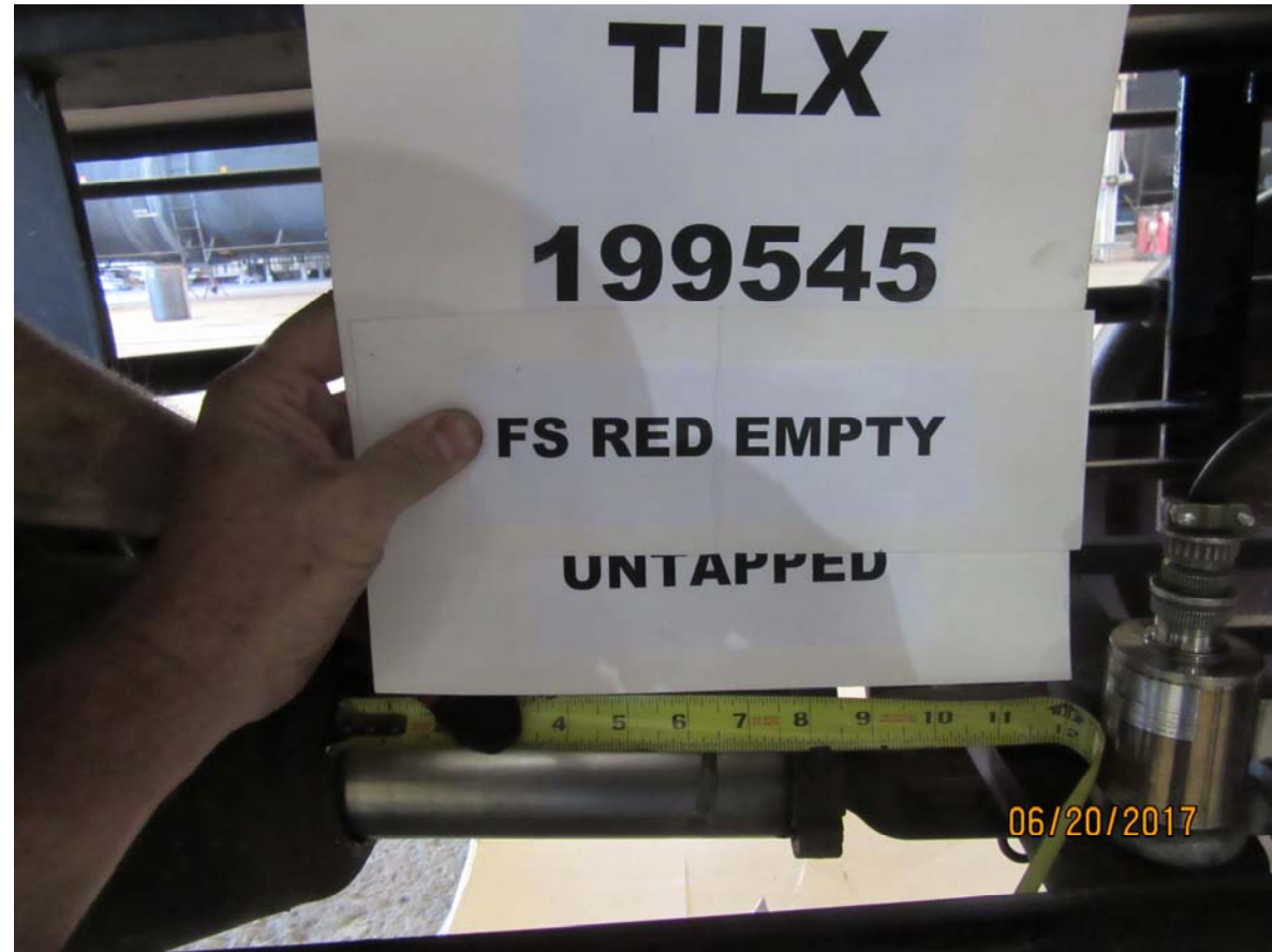
Figure 4362: TILX 199545, full service BPP reduction, empty car, BC piston length, brake pins untapped (Figure 4361 backup)
