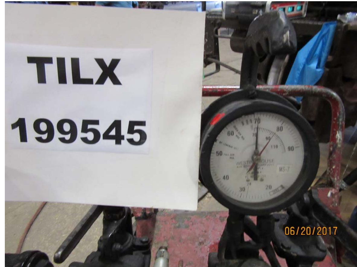
Figure 4338: TILX 199545, 20 pound brake pipe pressure (BPP) reduction, loaded car, brake pipe pressure
