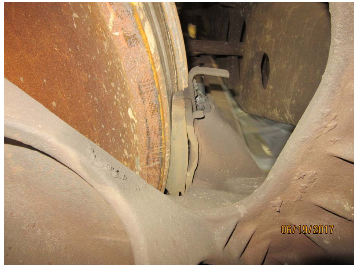
Figure 4248: TILX 320122, brake shoe and wheel tread
