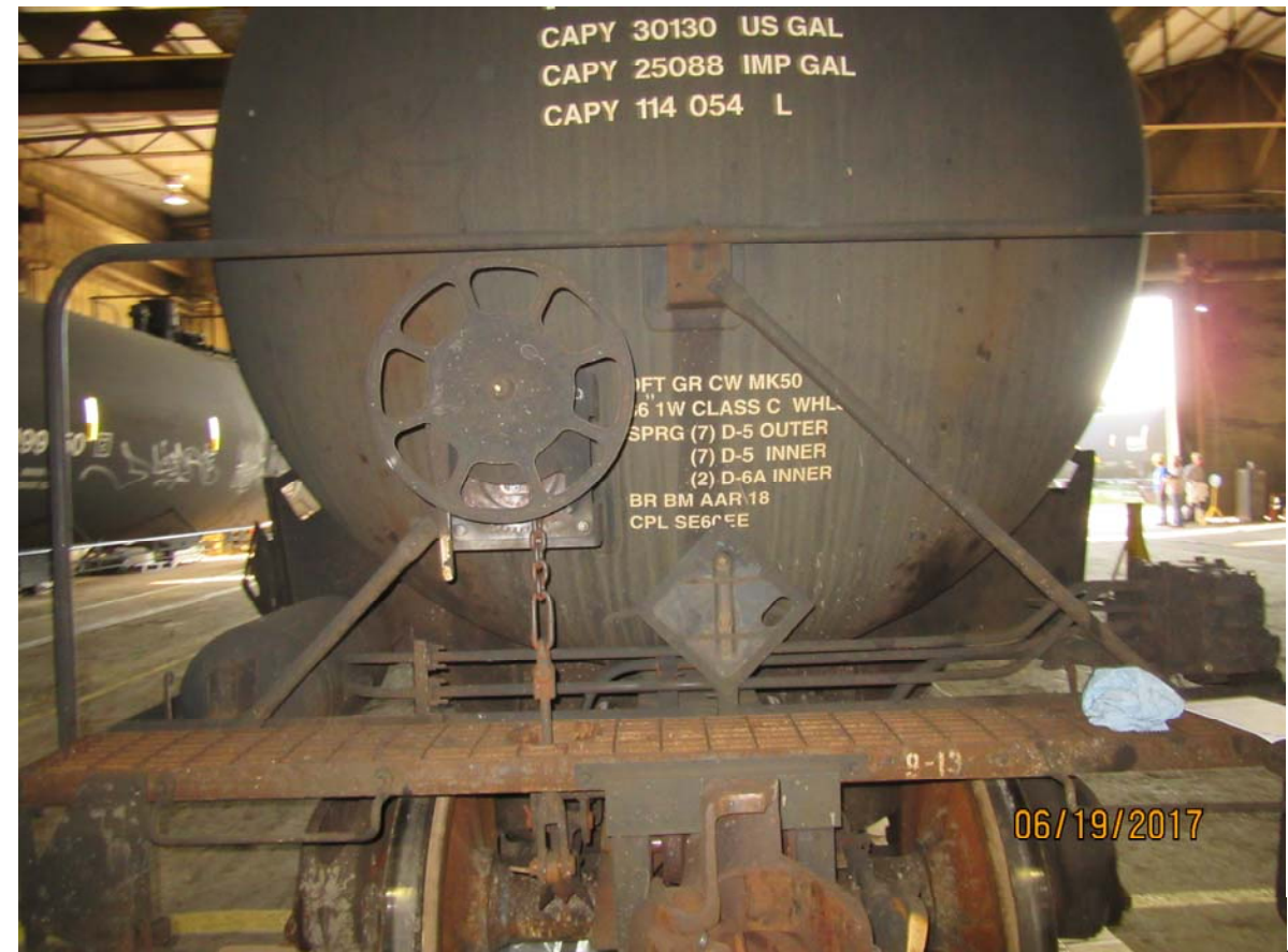
Figure 4241: TILX 320122, handbrake arrangement
