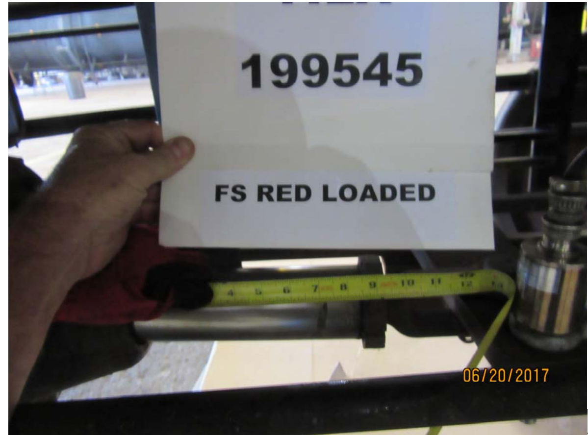
Figure 4343: TILX 199545, full service BPP reduction, loaded car, BC piston length
