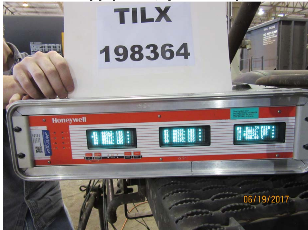
Figure 4299: TILX 198364, minimum service BPP reduction, loaded car, brake shoe forces, brake pins untapped
