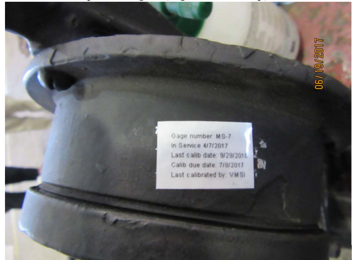
Figure 4284: TILX 198364, single car brake test stand, pressure gauge calibration data
