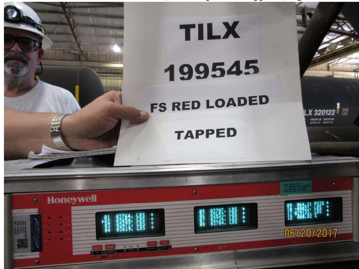
Figure 4356: TILX 199545, full service BPP reduction, loaded car, brake shoe forces, brake pins tapped (Figure 4355 backup)
