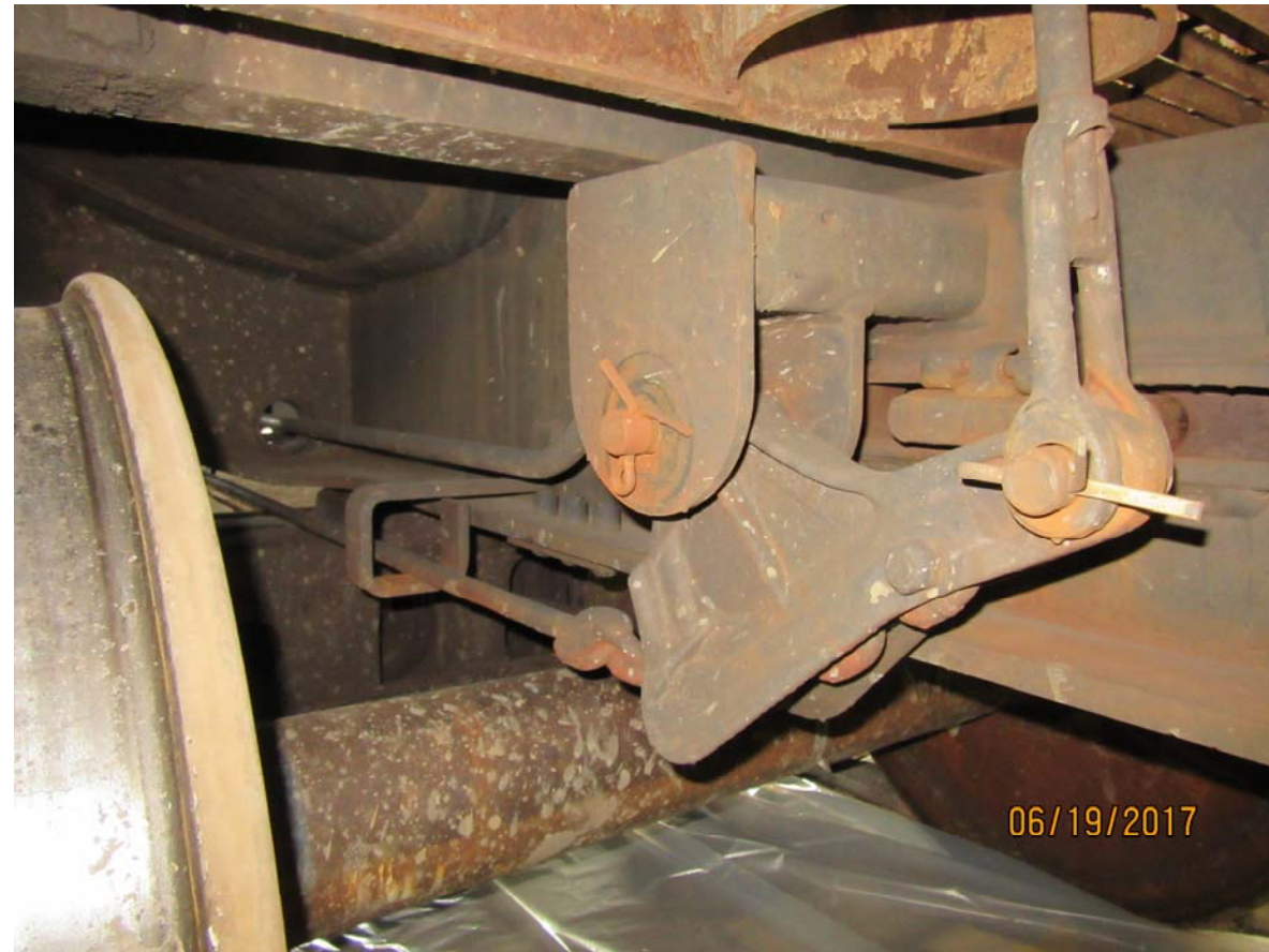
Figure 4242: TILX 320122, handbrake control input connections
