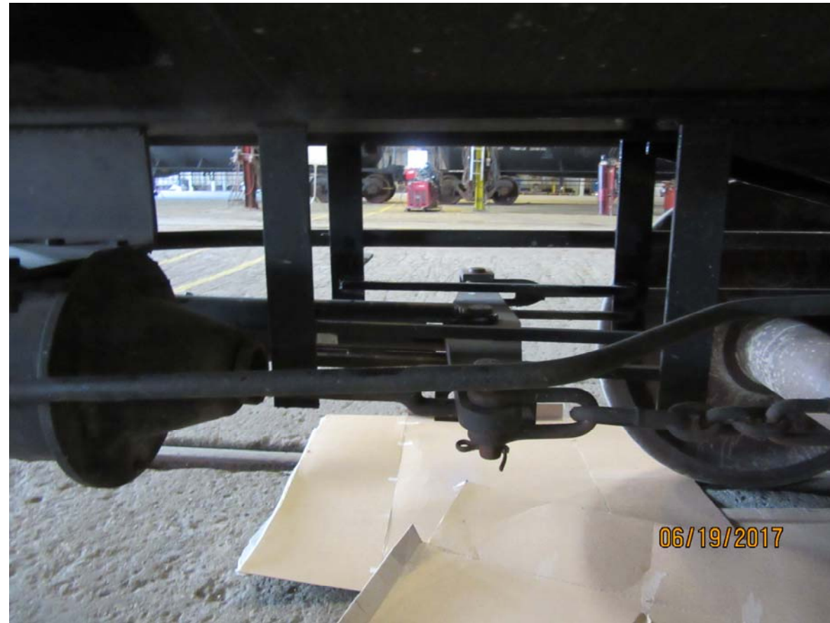
Figure 4230: TILX 199545, brake cylinder and handbrake pin connection
