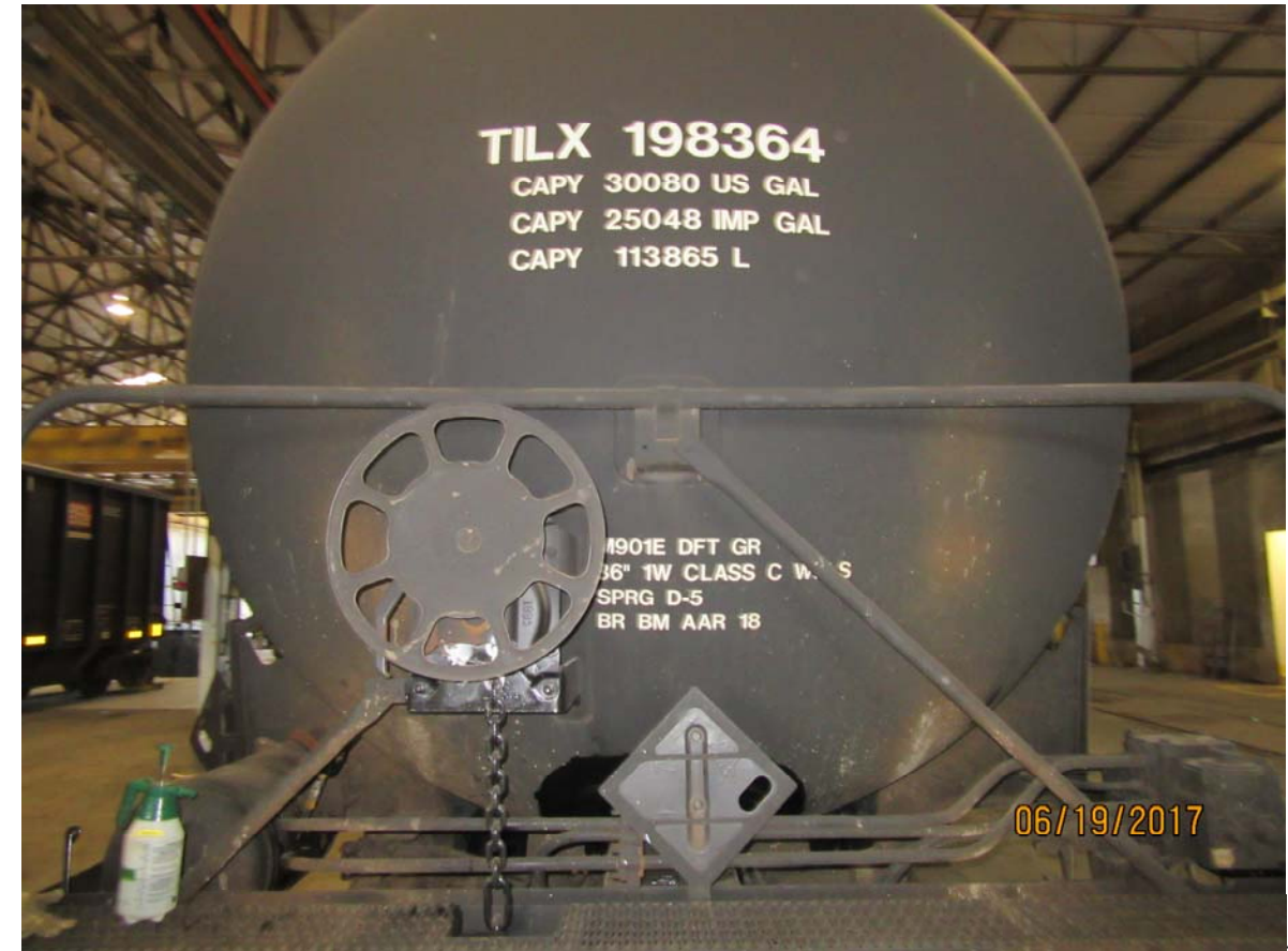
Figure 4255: TILX 198364, handbrake arrangement and chain
