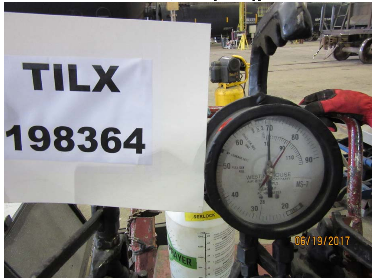
Figure 4311: TILX 198364, 20 pound BPP reduction, empty car, brake pipe pressure
