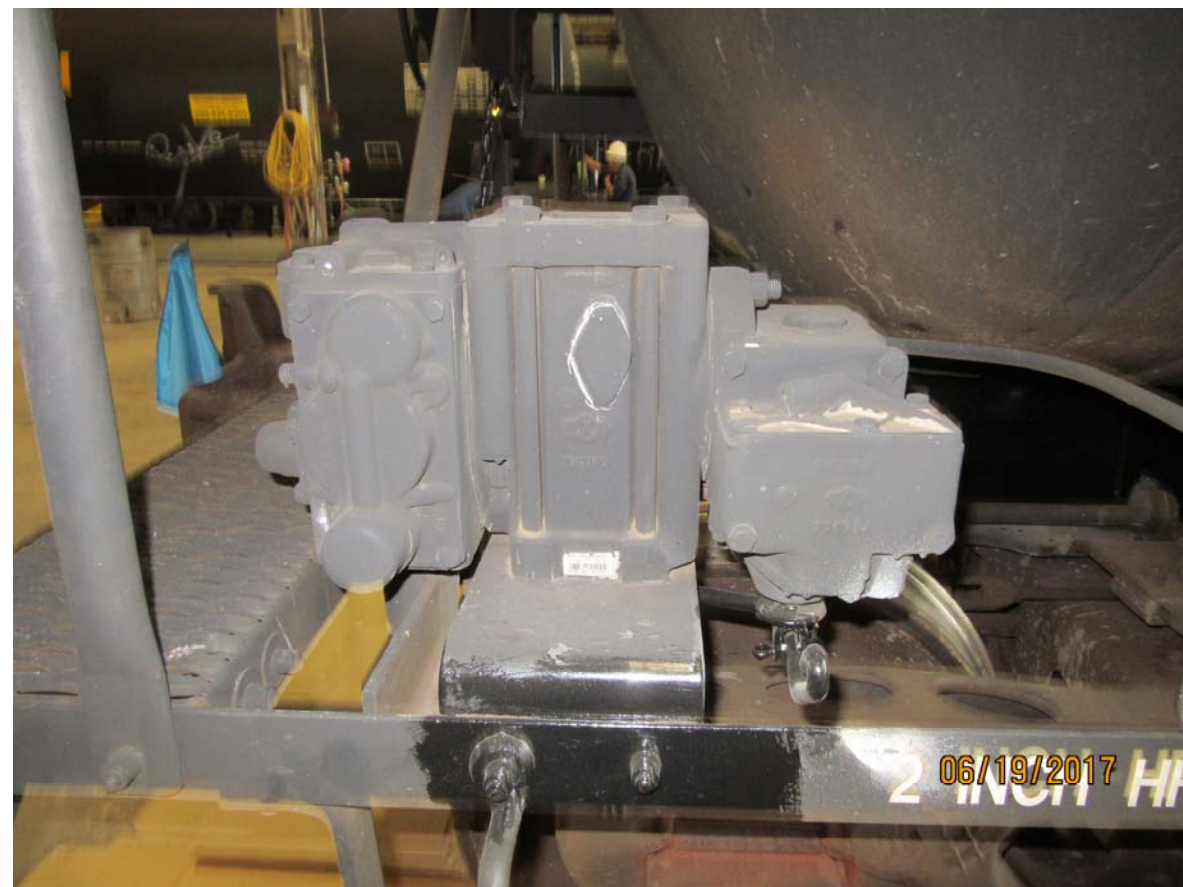
Figure 4236: TILX 199545, brake control valve
