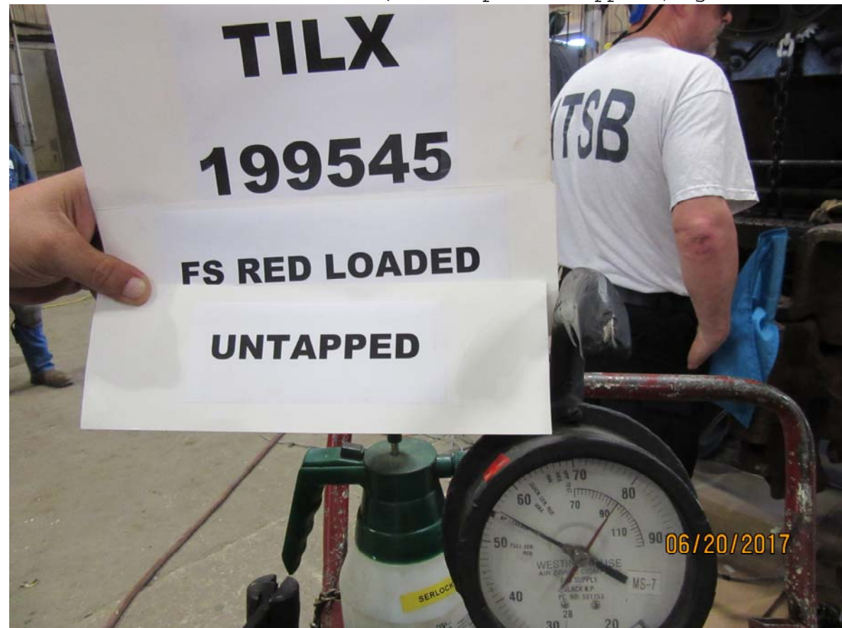
Figure 4352: TILX 199545, full service BPP reduction, loaded car, brake pipe pressure, brake pins untapped
