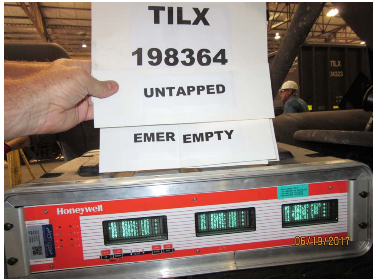
Figure 4321: TILX 198364, emergency BPP reduction, empty car, brake shoe forces, brake pins untapped
