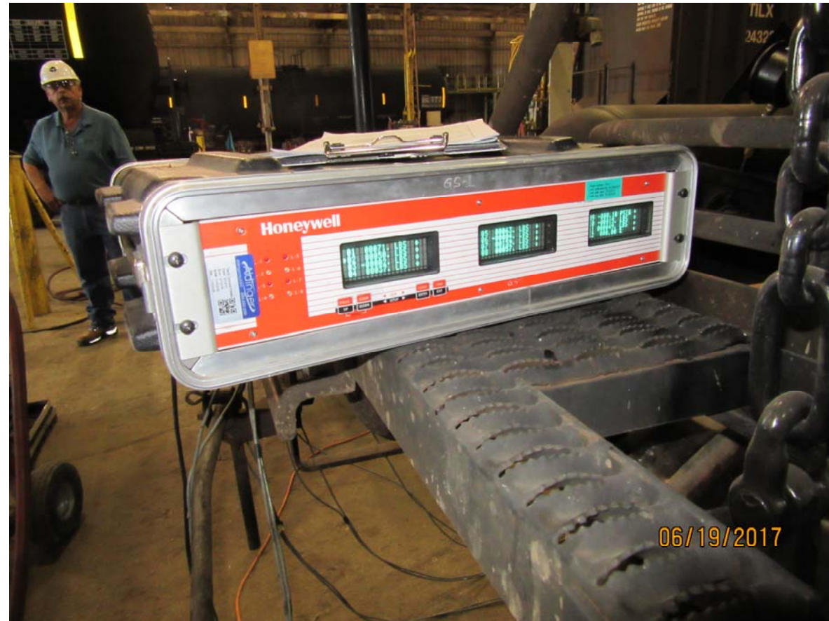
Figure 4285: TILX 198364, force and pressure data acquisition unit, brake shoe forces on channels 1-8, BC pressure on channel 9
