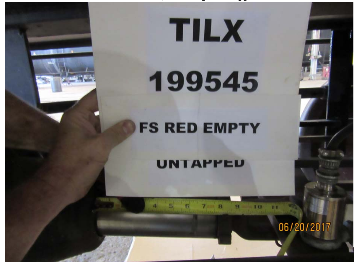
Figure 4361: TILX 199545, full service BPP reduction, empty car, BC piston length, brake pins untapped
