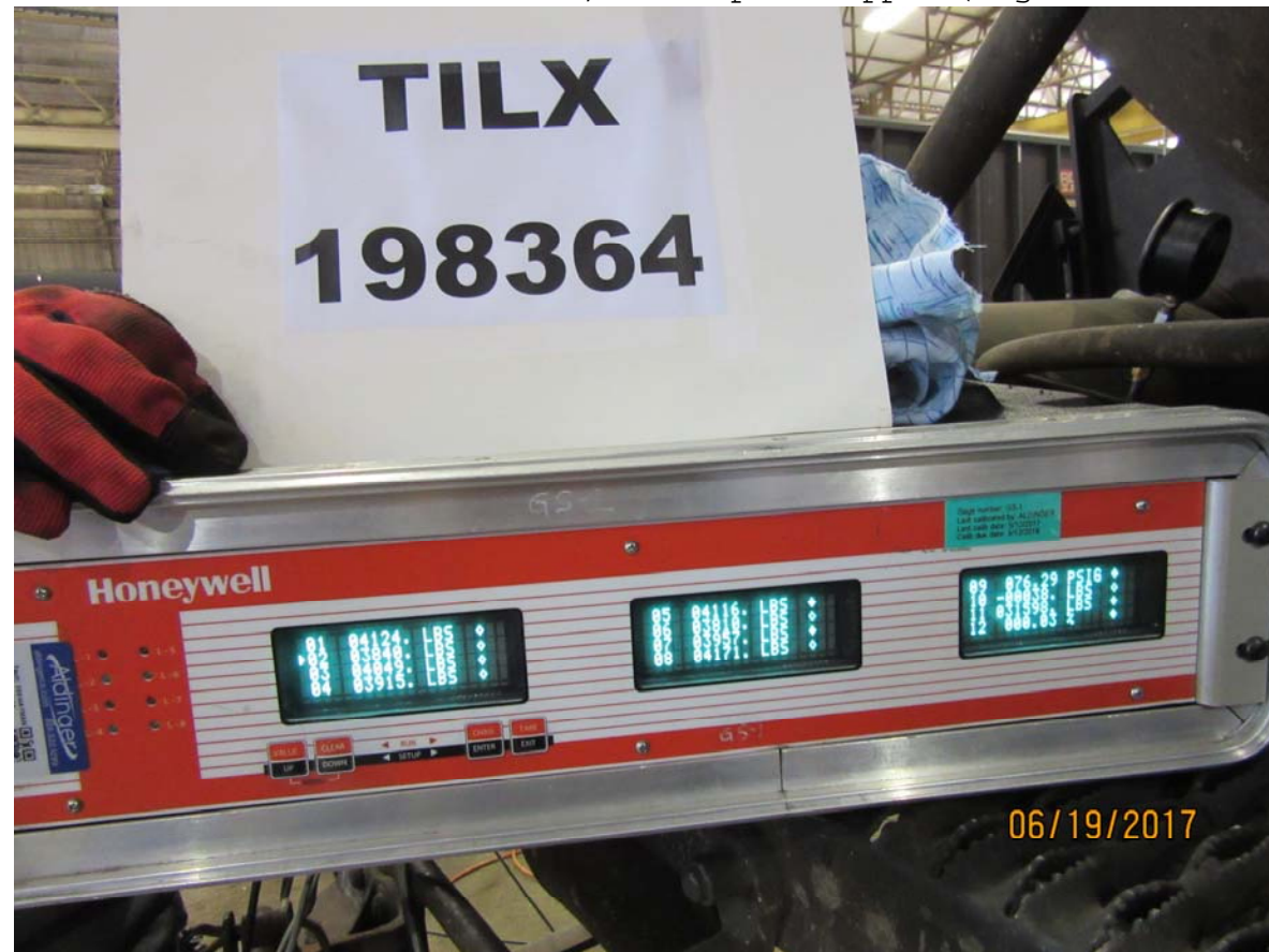
Figure 4307: TILX 198364, emergency BPP reduction, loaded car, brake shoe forces, brake pins untapped
