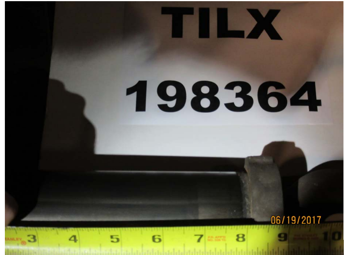
Figure 4278: TILX 198364, 20 pound BPP reduction, loaded car, BC piston length (Figure 4277 backup)
