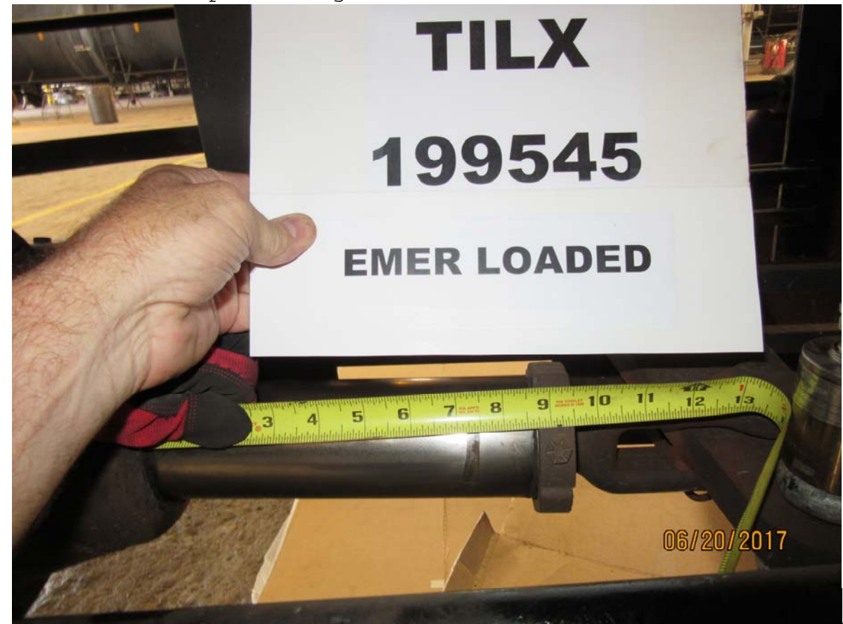
Figure 4345: TILX 199545, emergency BPP reduction, loaded car, BC piston length
