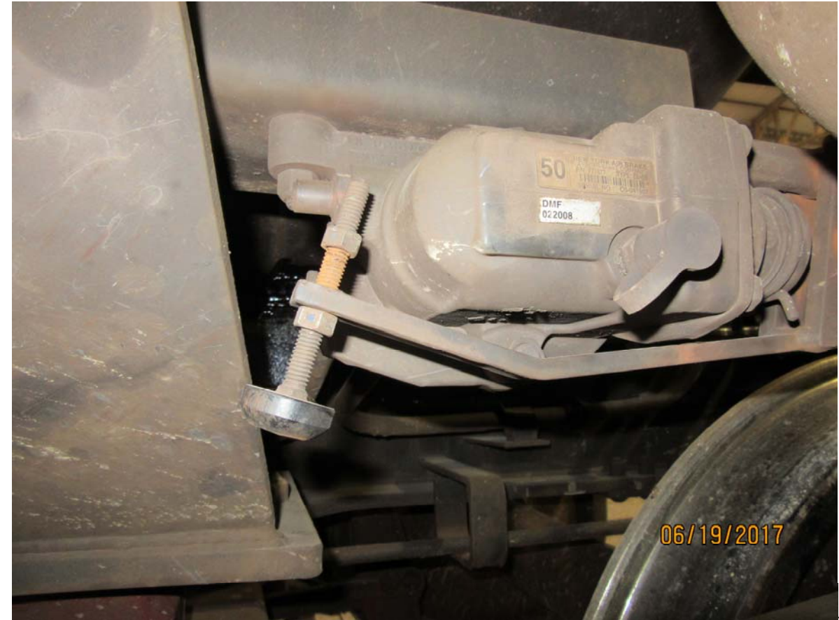
Figure 4239: TILX 199545, empty load device
