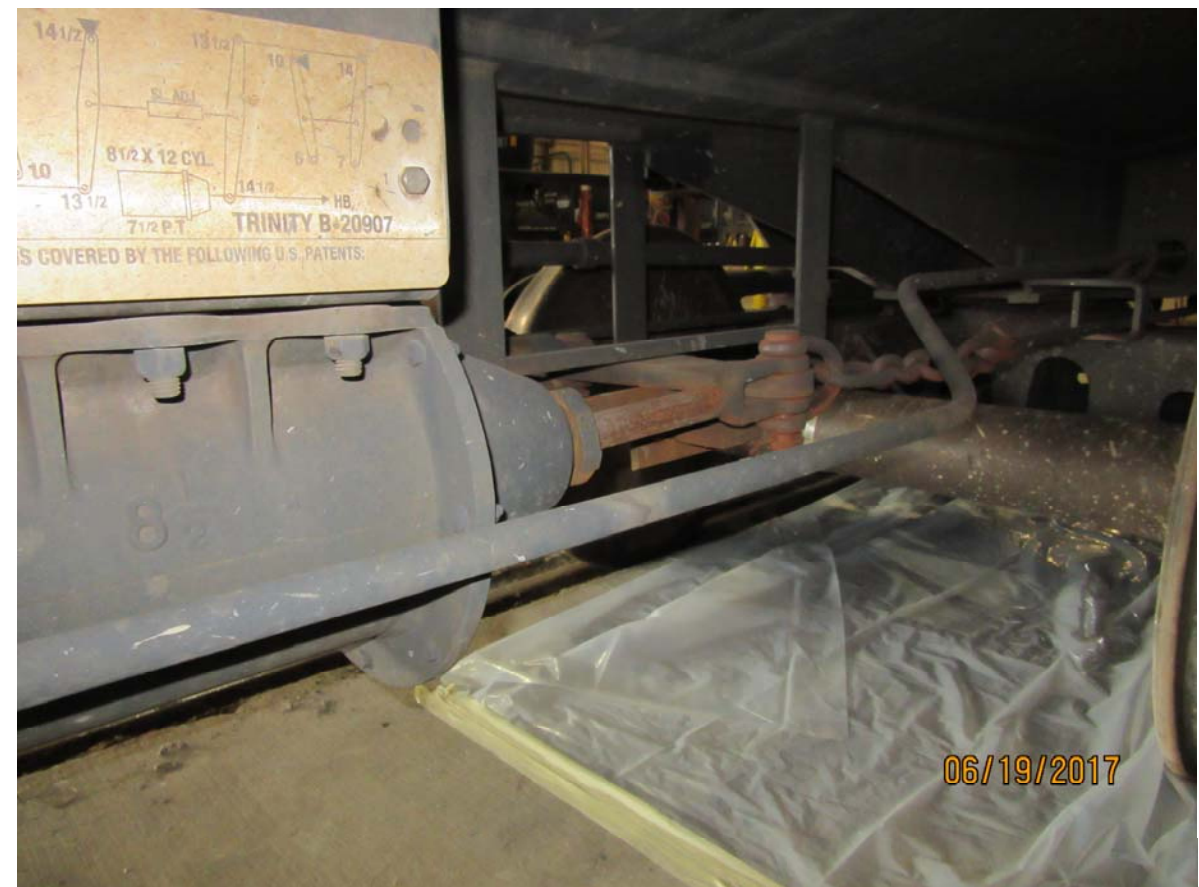
Figure 4253: TILX 320122, brake cylinder and mechanical linkages
