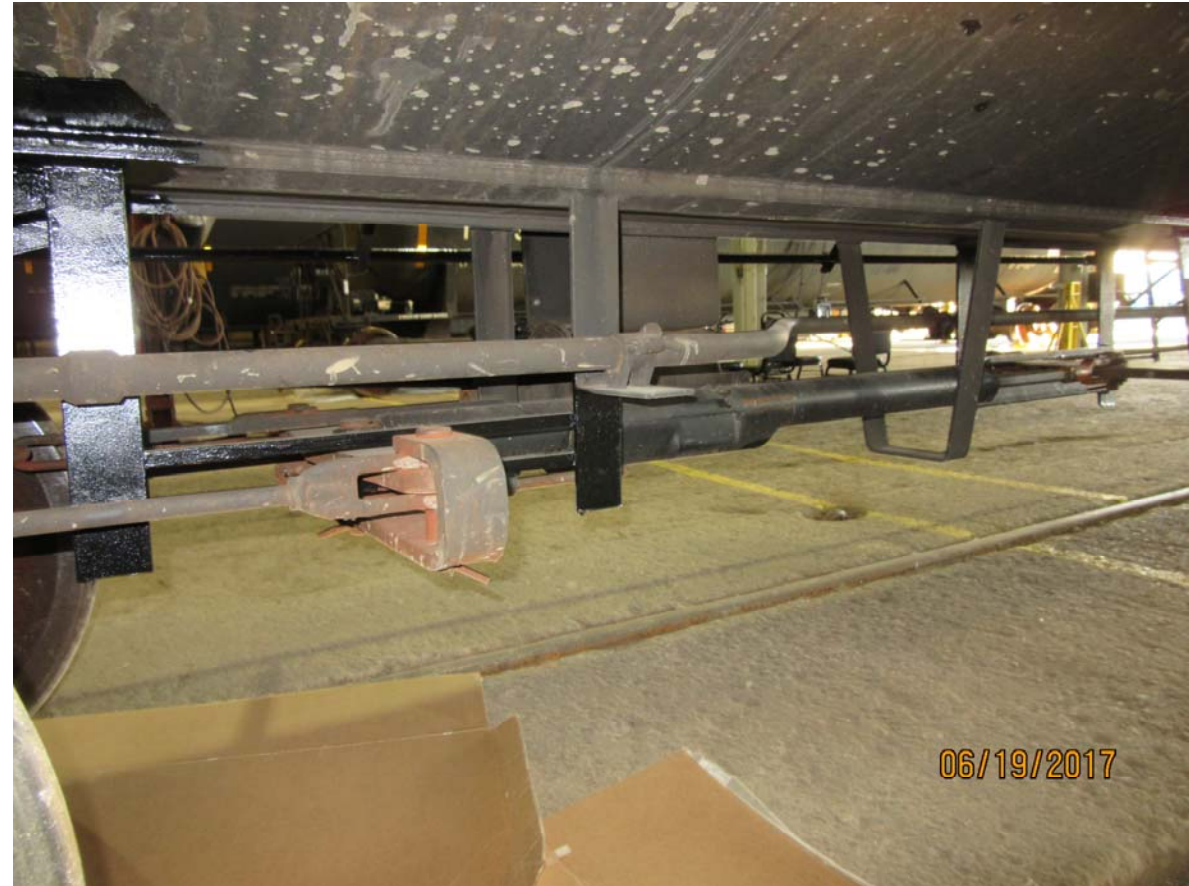
Figure 4238: TILX 199545, slack adjuster and mechanical linkages
