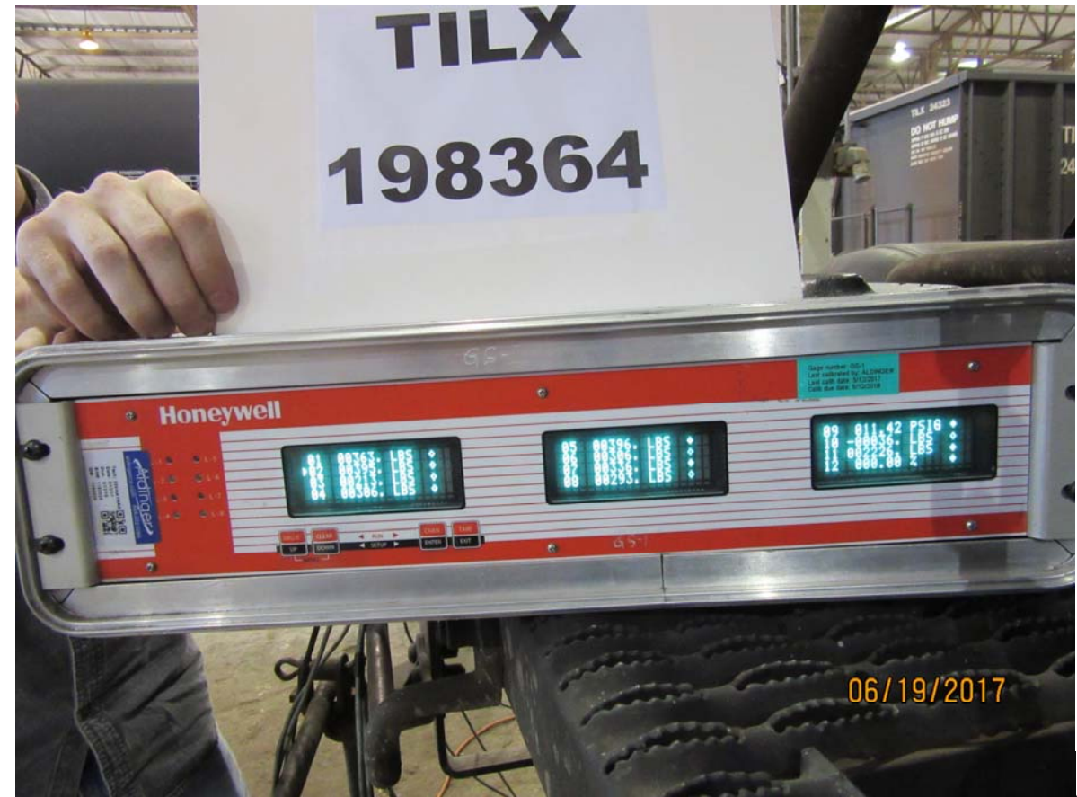
Figure 4300: TILX 198364, minimum service BPP reduction, loaded car, brake shoe forces, brake pins untapped (Figure 4299 backup)
