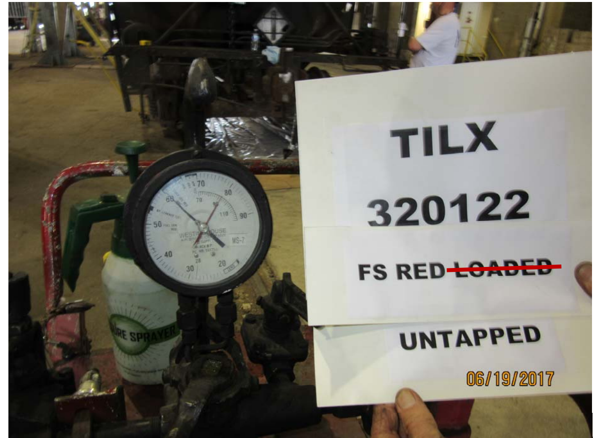
Figure 4332: TILX 320122, full service BPP reduction, car empty/loaded, brake pipe pressure, brake pins untapped
