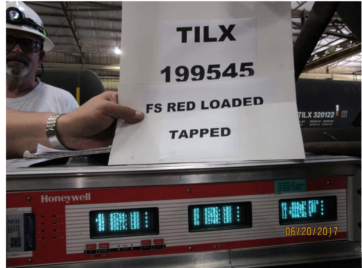
Figure 4355: TILX 199545, full service BPP reduction, loaded car, brake shoe forces, brake pins tapped
