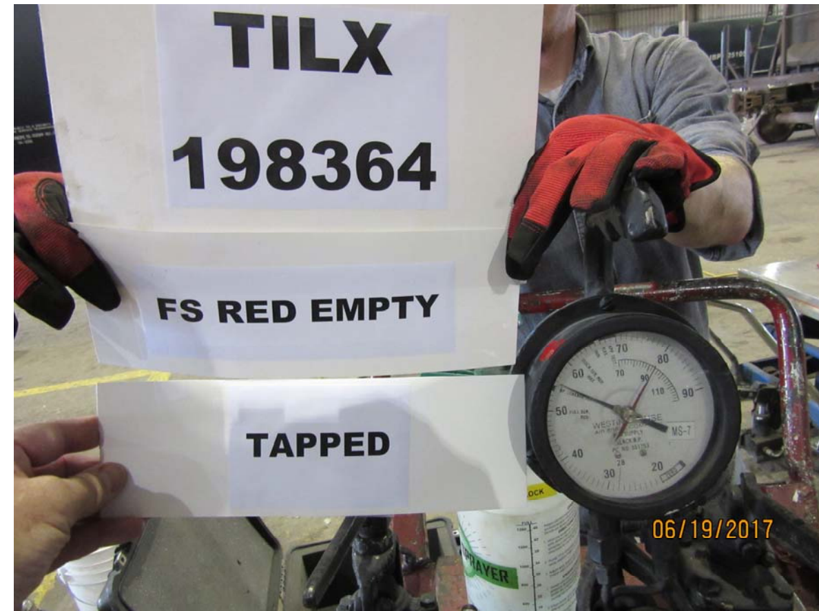
Figure 4320: TILX 198364, full service BPP reduction, empty car, brake pipe pressure, brake pins tapped
