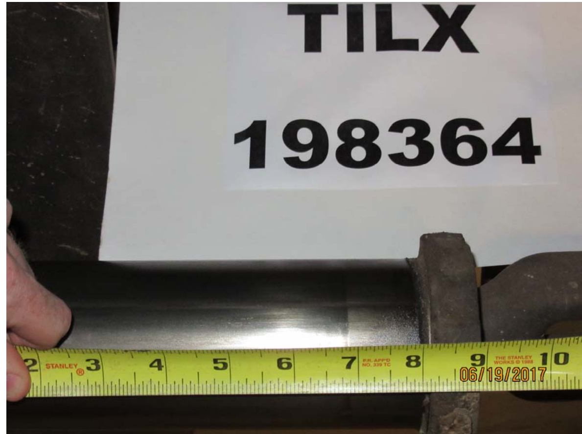
Figure 4277: TILX 198364, 20 pound brake pipe pressure (BPP) reduction, loaded car, brake cylinder (BC) piston length
