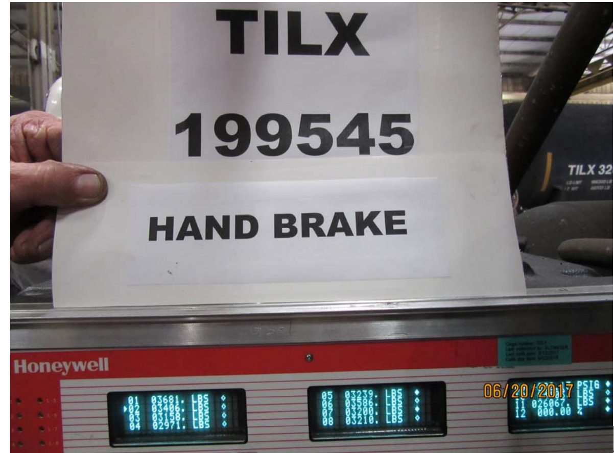
Figure 4347: TILX 199545, handbrake application, brake shoe forces (Figure 4346 backup)
