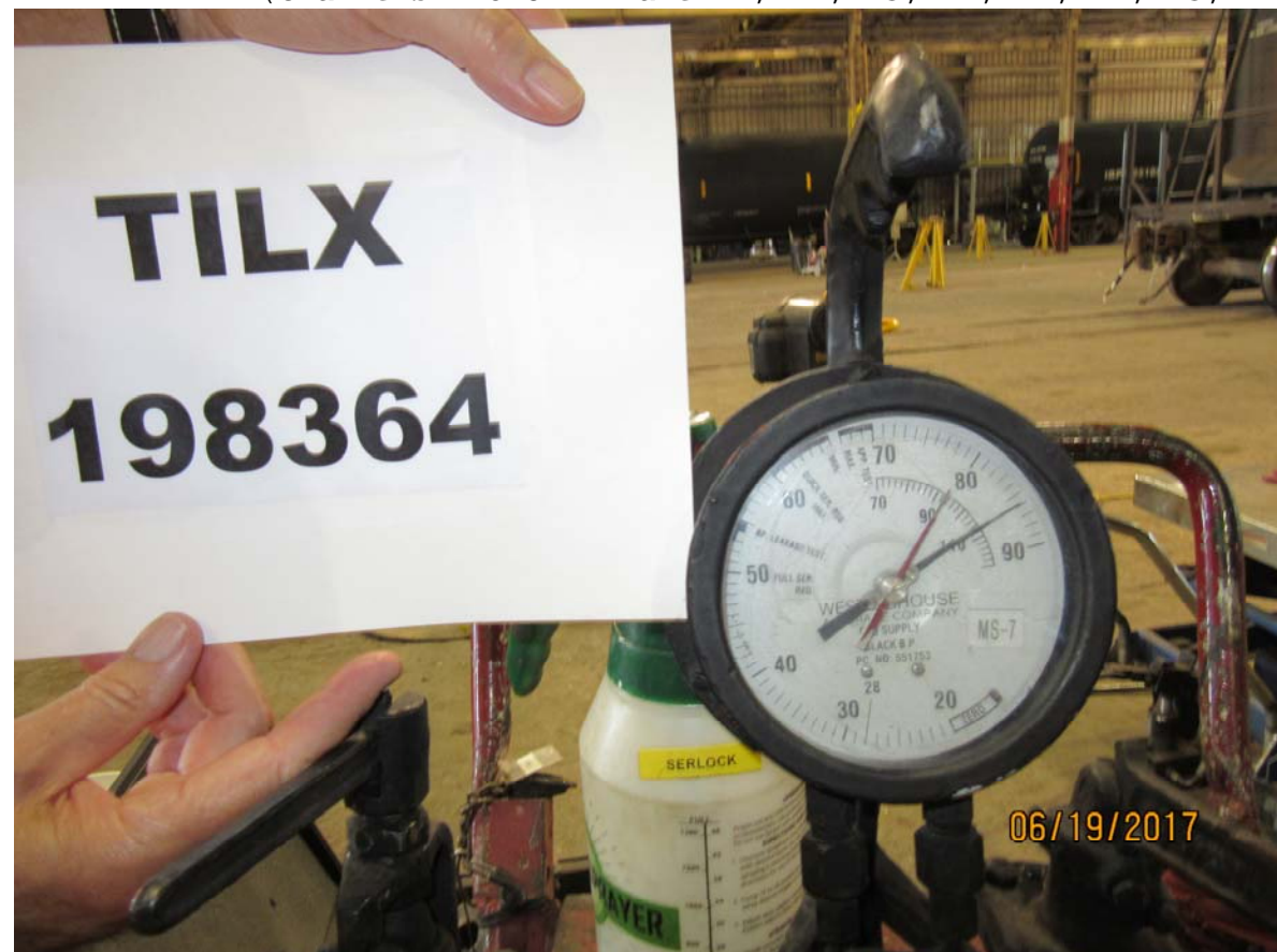
Figure 4295: TILX 198364, minimum service BPP reduction, loaded car, brake pipe pressure
