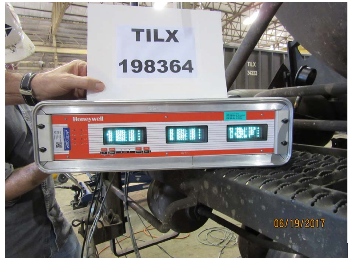
Figure 4294: TILX 198364, handbrake application, brake shoe forces (Figure 4293 backup)
