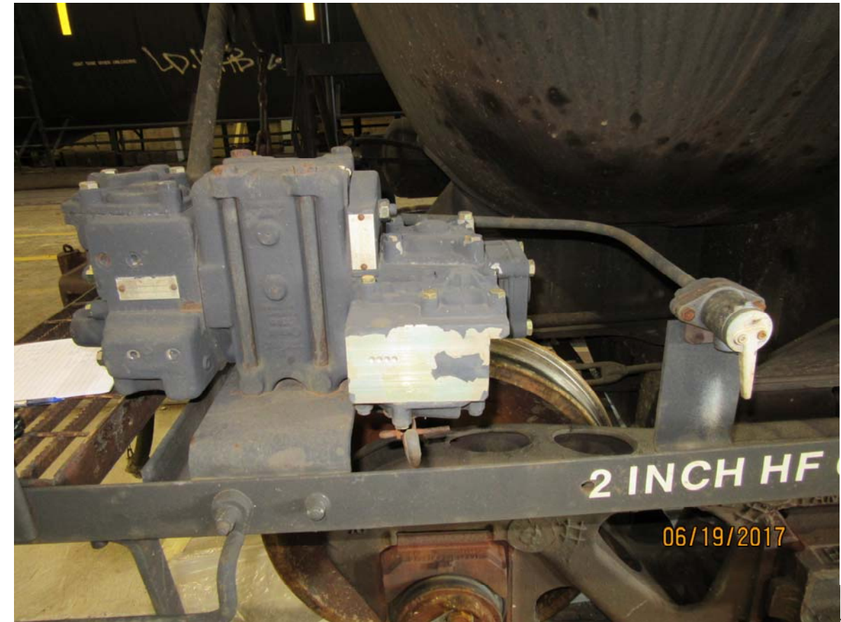
Figure 4247: TILX 320122, retainer valve
