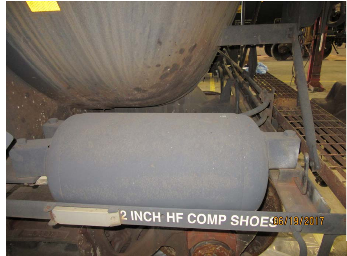
Figure 4243: TILX 320122, air reservoir (auxiliary and emergency)
