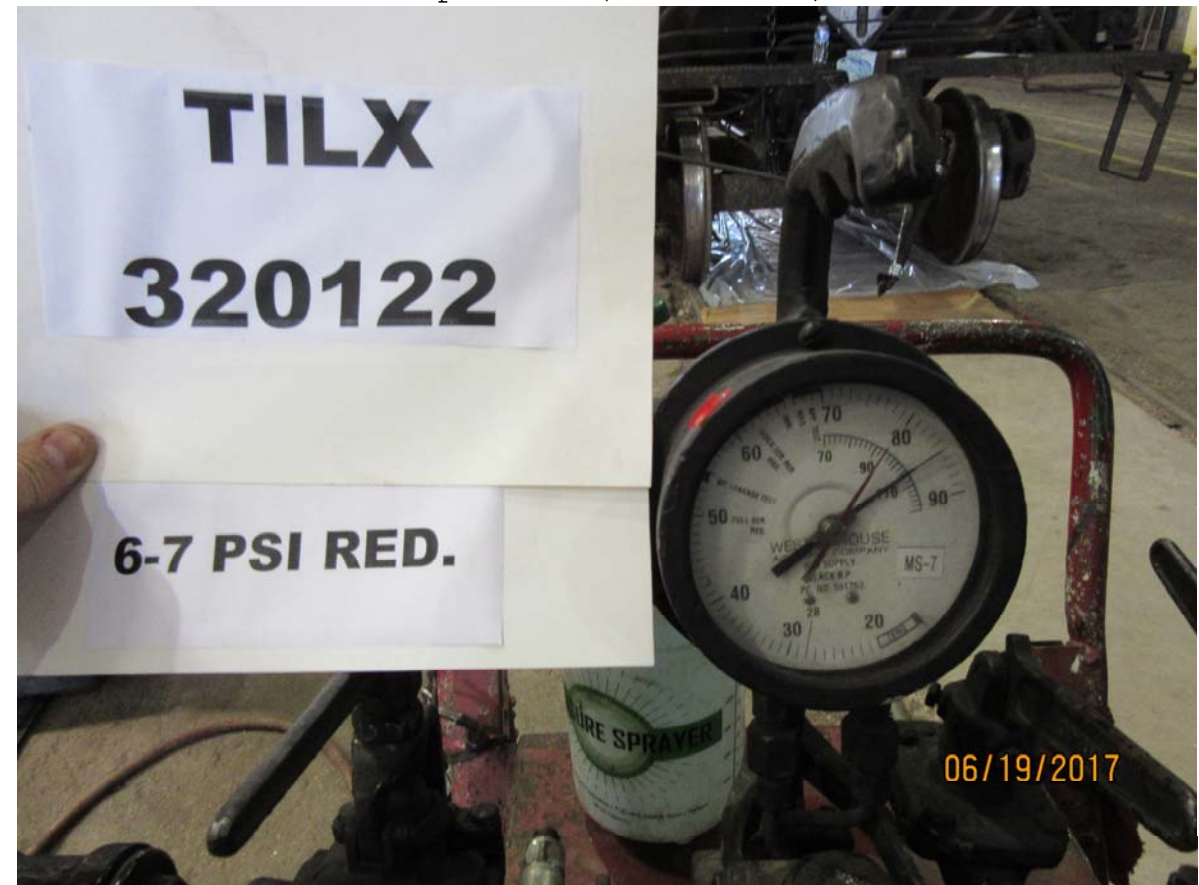
Figure 4330: TILX 320122, minimum service BPP reduction, car not equipped with empty load valve, brake pipe pressure
