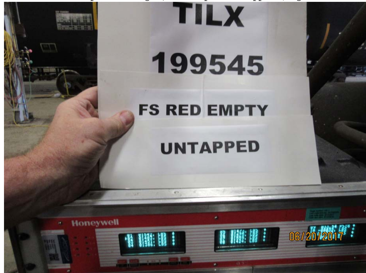
Figure 4368: TILX 199545, full service BPP reduction, empty car, brake shoe forces, brake pins untapped
