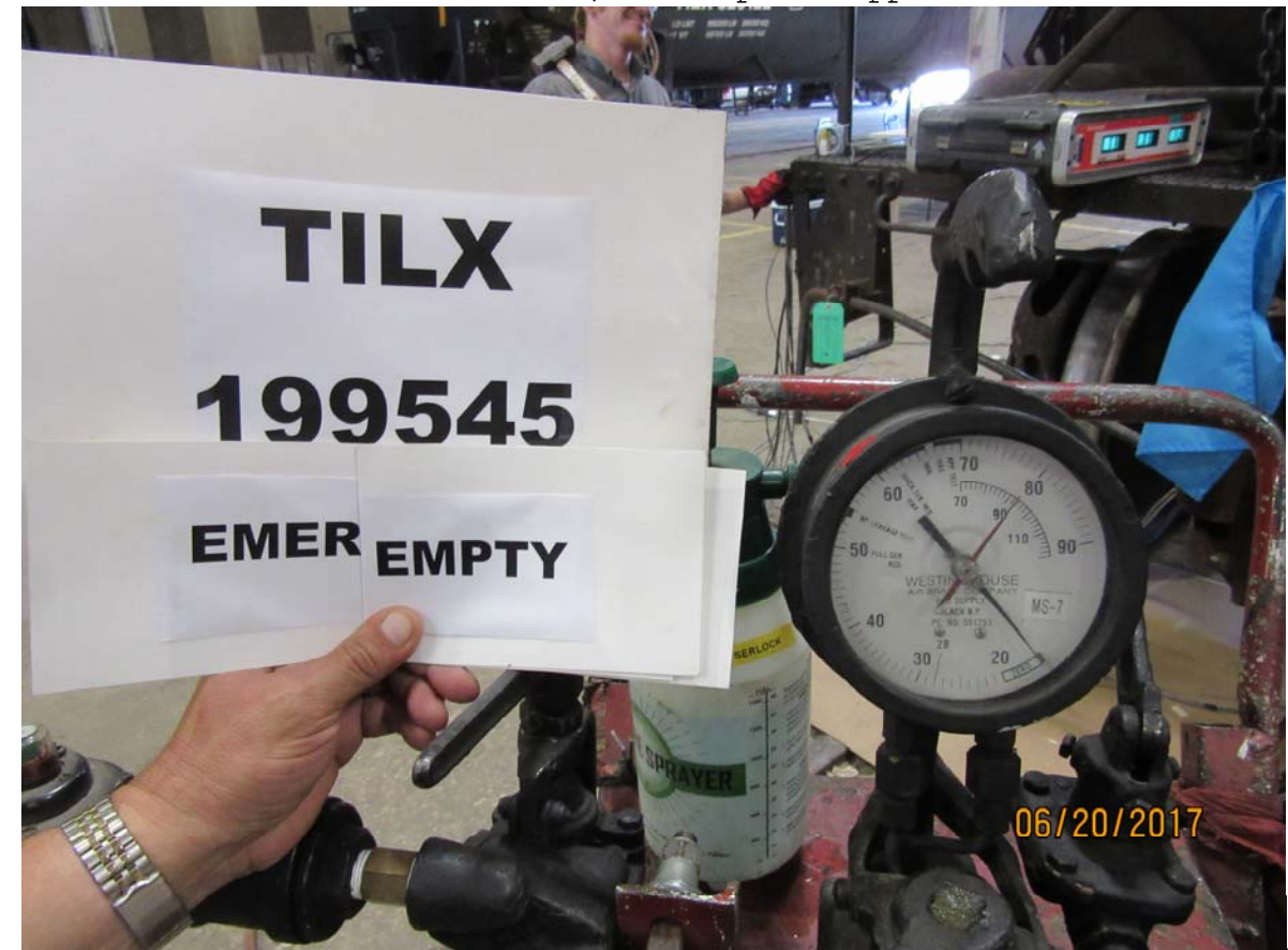
Figure 4373: TILX 199545, emergency BPP reduction, empty car, brake pipe pressure, brake pins untapped
