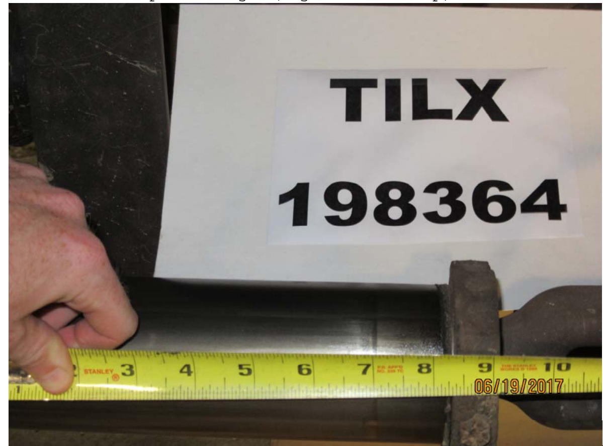
Figure 4280: TILX 198364, full service BPP reduction, loaded car, BC piston length (Figure 4279 backup)
