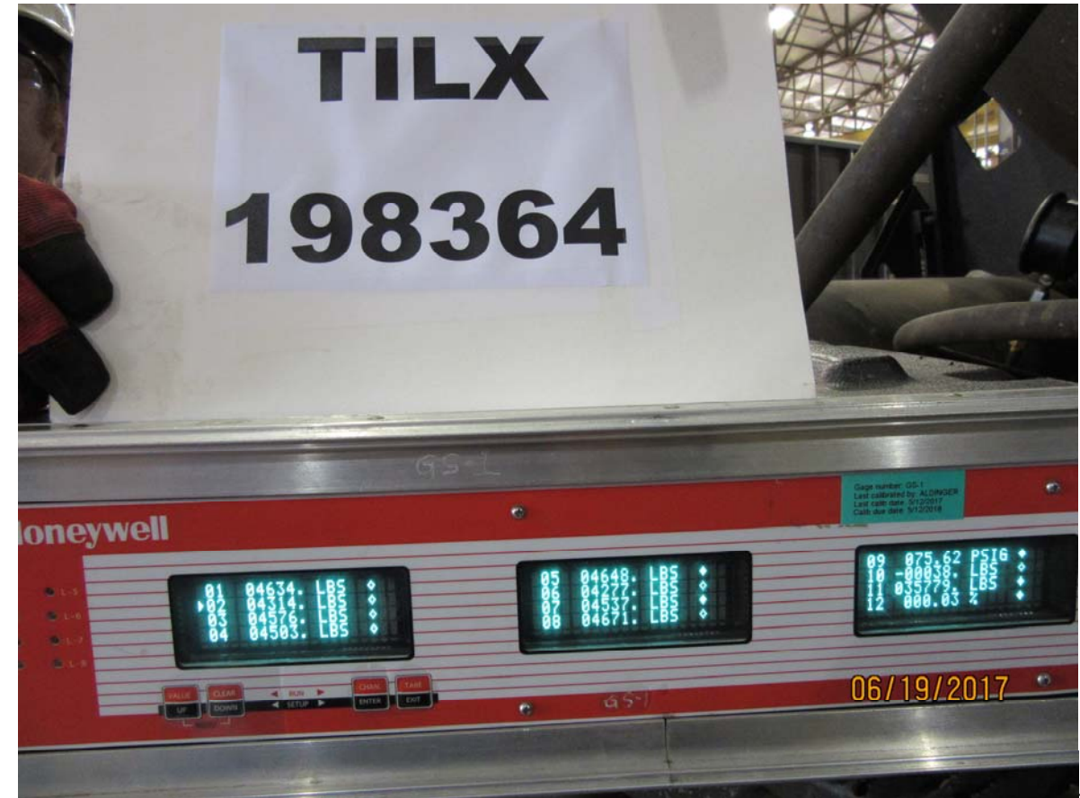
Figure 4310: TILX 198364, emergency BPP reduction, loaded car, brake shoe forces, brake pins tapped (Figure 4309 backup)
