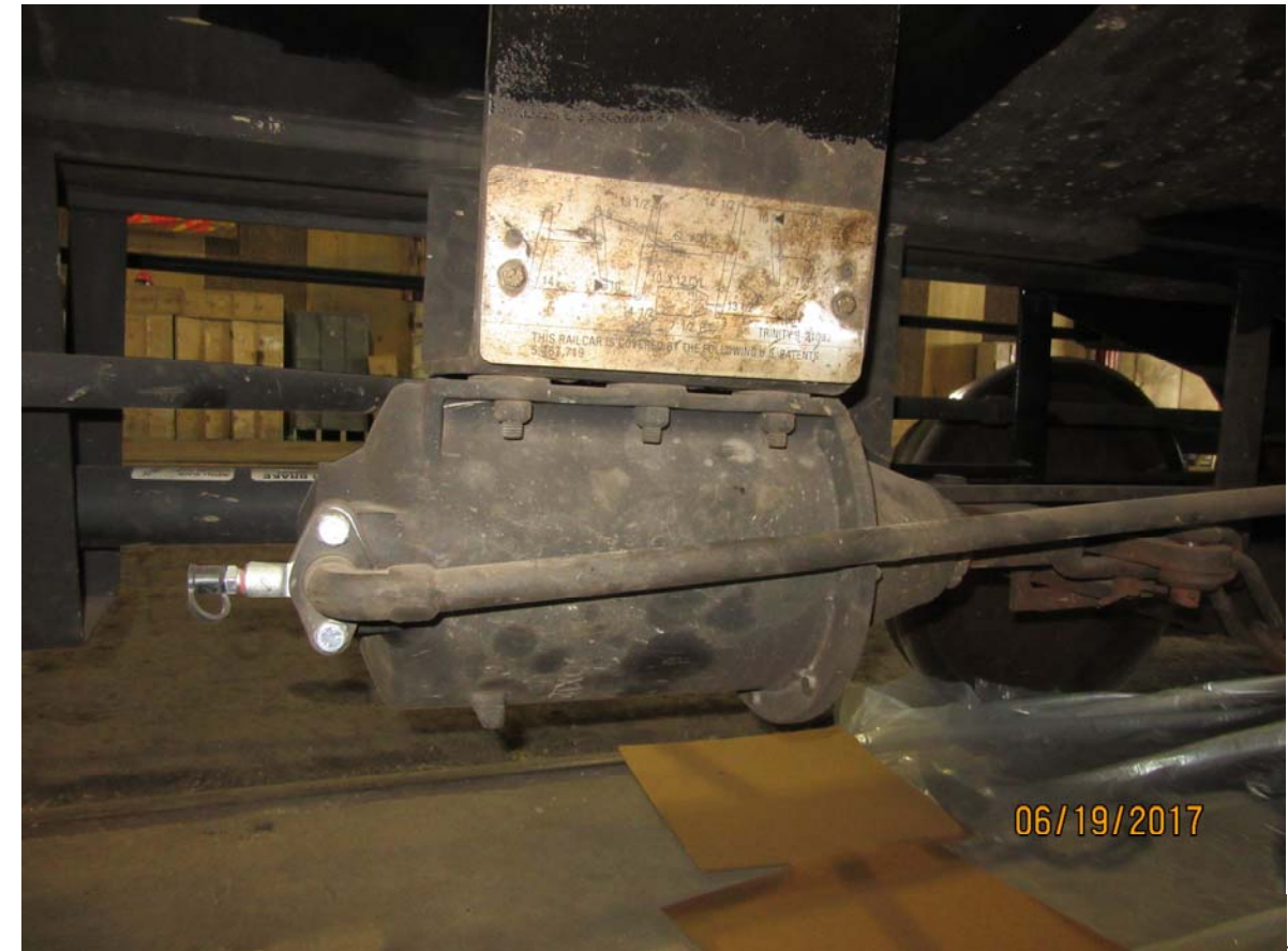
Figure 4259: TILX 198364, brake cylinder with brake cylinder pressure tap
