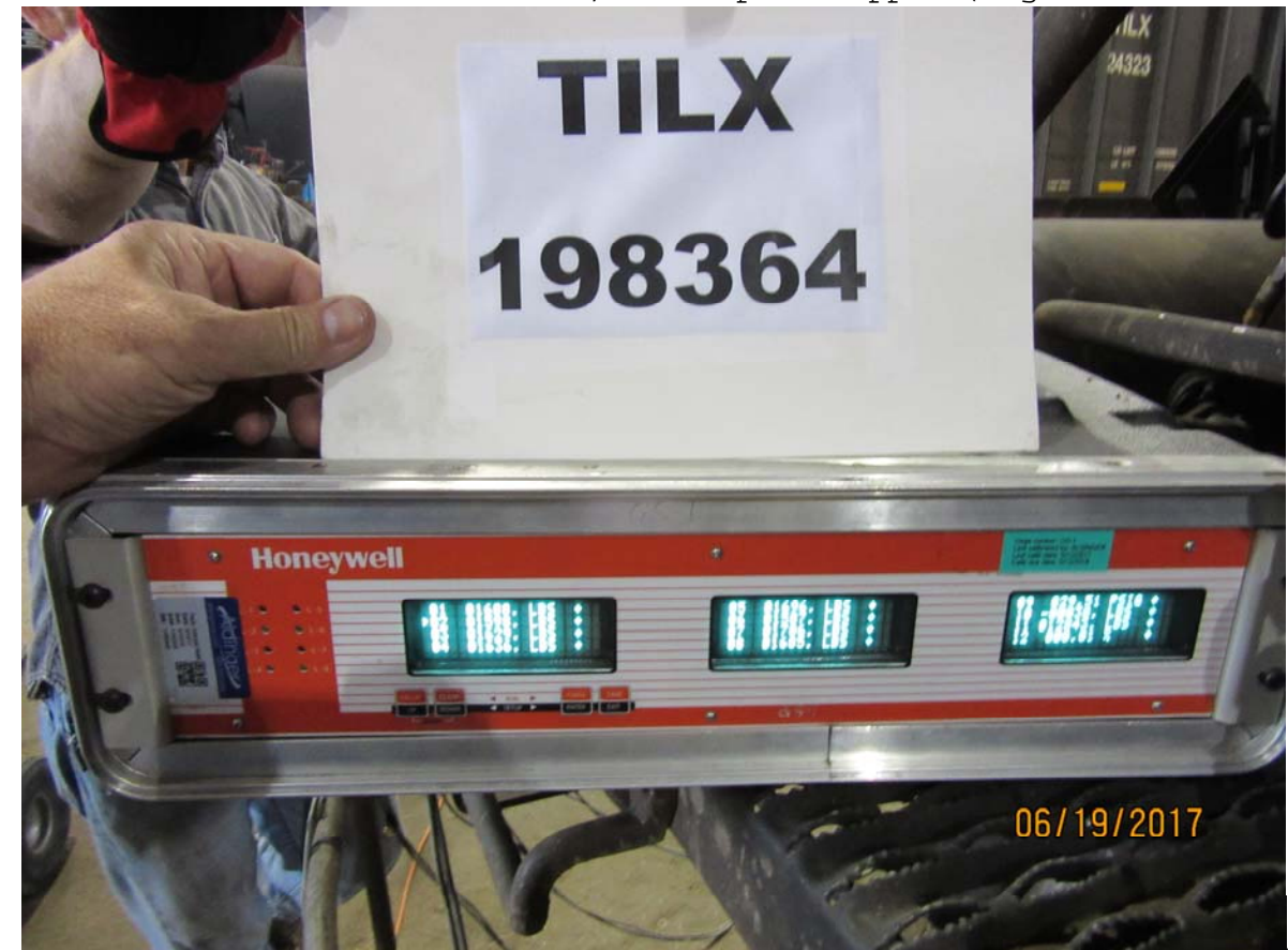
Figure 4312: TILX 198364, 20 pound BPP reduction, empty car, brake shoe forces, brake pins untapped
