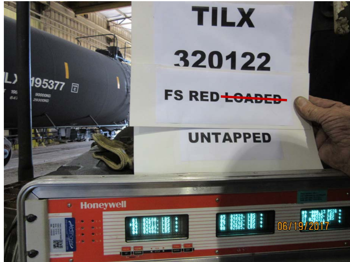
Figure 4335: TILX 320122, full service BPP reduction, car empty/loaded, brake shoe forces, brake pins untapped (Figure 4334 backup)
