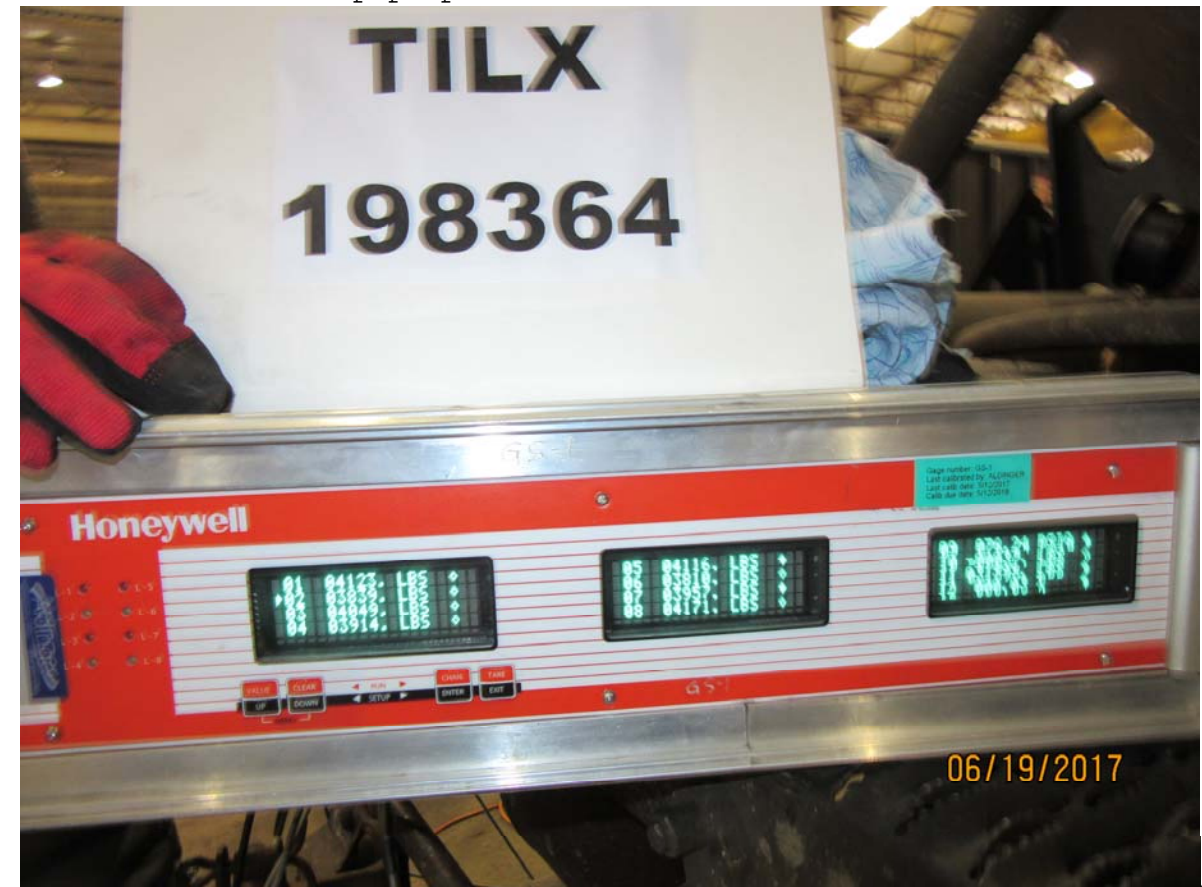
Figure 4308: TILX 198364, emergency BPP reduction, loaded car, brake shoe forces, brake pins untapped (Figure 4307 backup)
