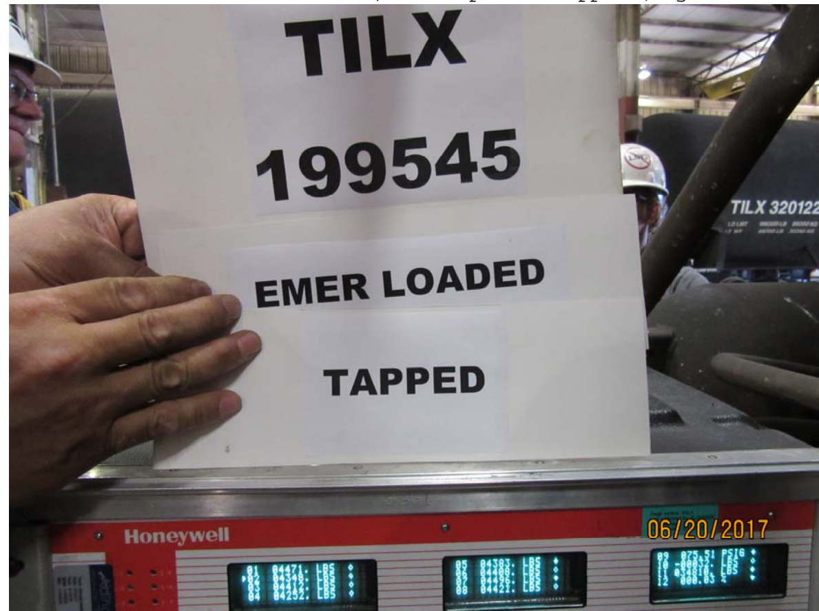
Figure 4360: TILX 199545, emergency BPP reduction, loaded car, brake shoe forces, brake pins tapped (Figure 4359 backup)
