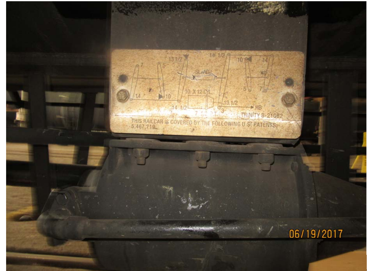
Figure 4231: TILX 199545, brake system mechanical linkage diagram
