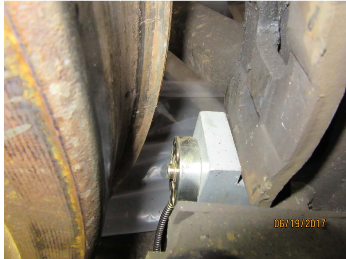
Figure 4327: TILX 320122, force transducer installed in nominal brake shoe position (view 3 of 4)
