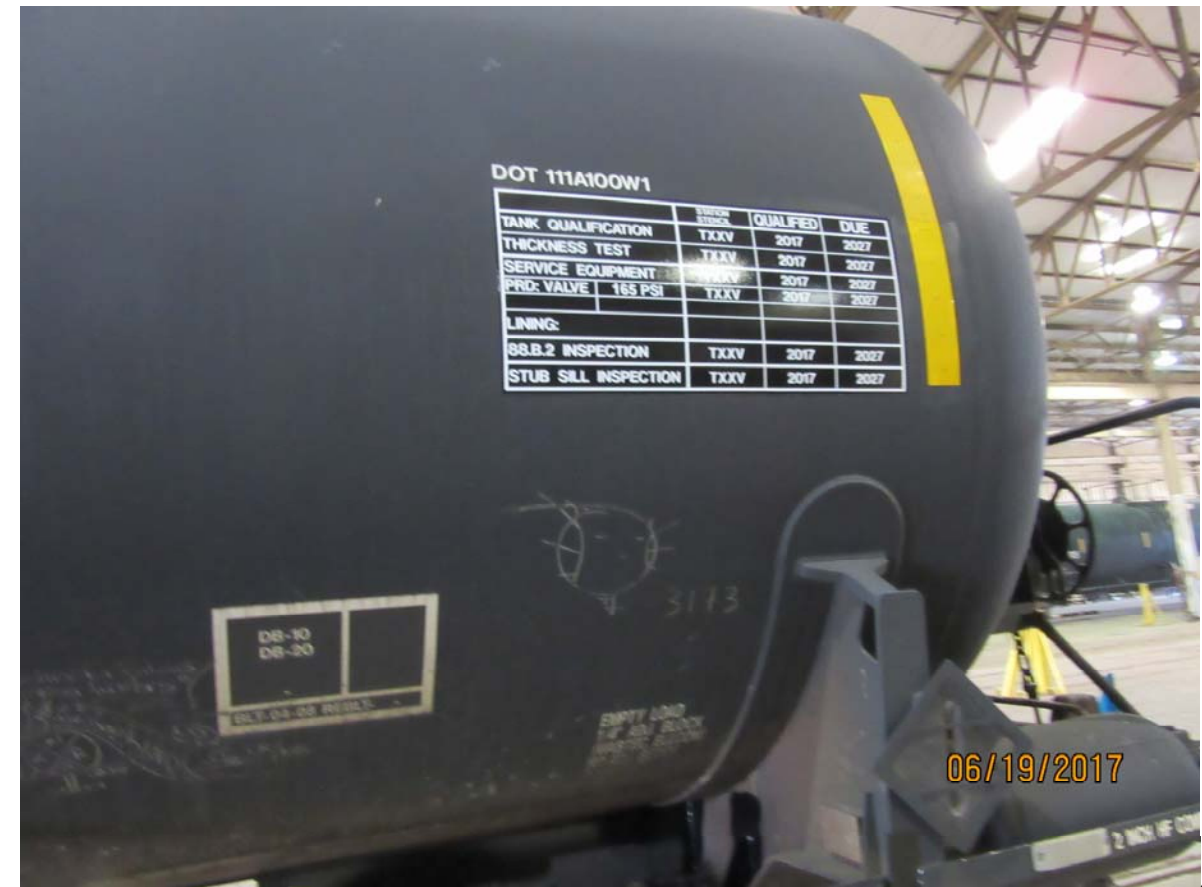
Figure 4229: TILX 199545, tank qualification and inspection schedules
