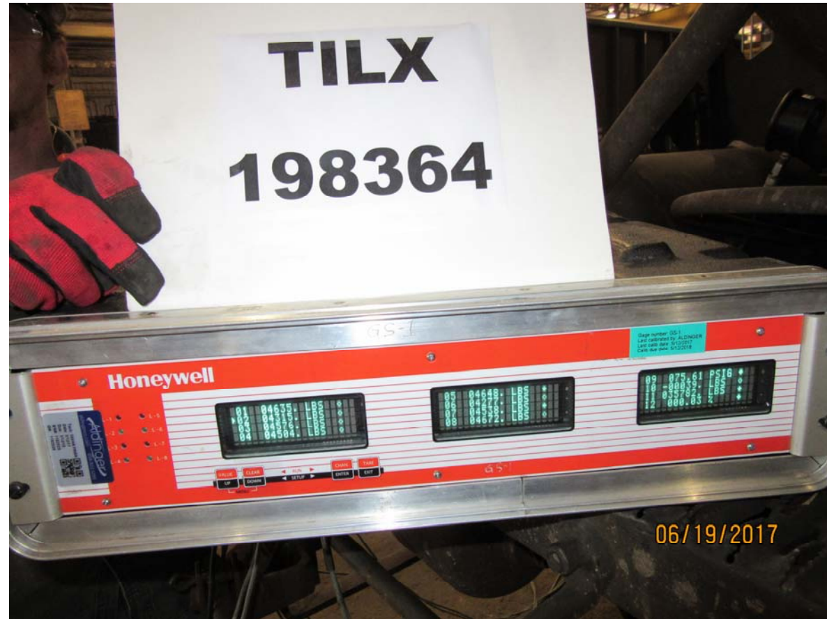
Figure 4309: TILX 198364, emergency BPP reduction, loaded car, brake shoe forces, brake pins tapped
