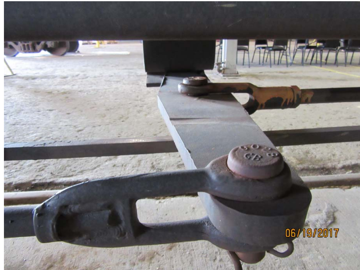
Figure 4254: TILX 320122, mechanical linkages and brake pins
