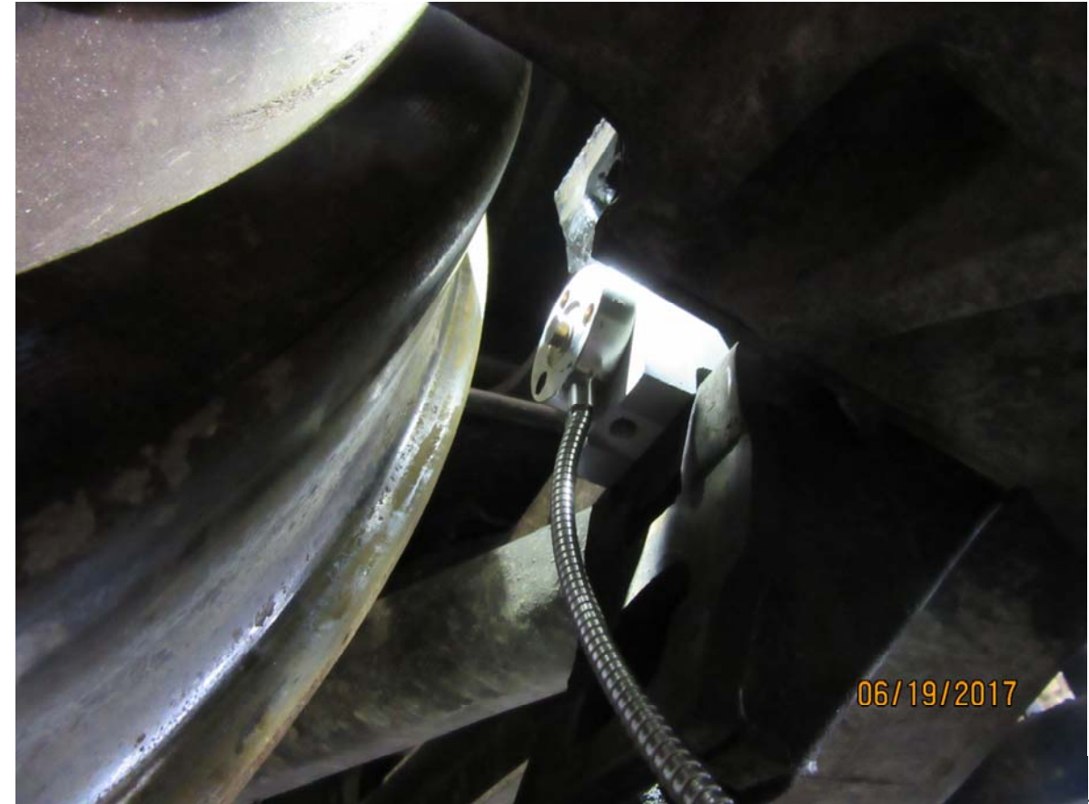
Figure 4328: TILX 320122, force transducer installed in nominal brake shoe position (view 4 of 4)
