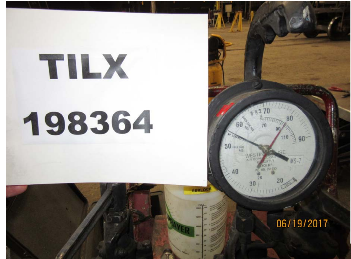
Figure 4314: TILX 198364, full service BPP reduction, empty car, brake pipe pressure
