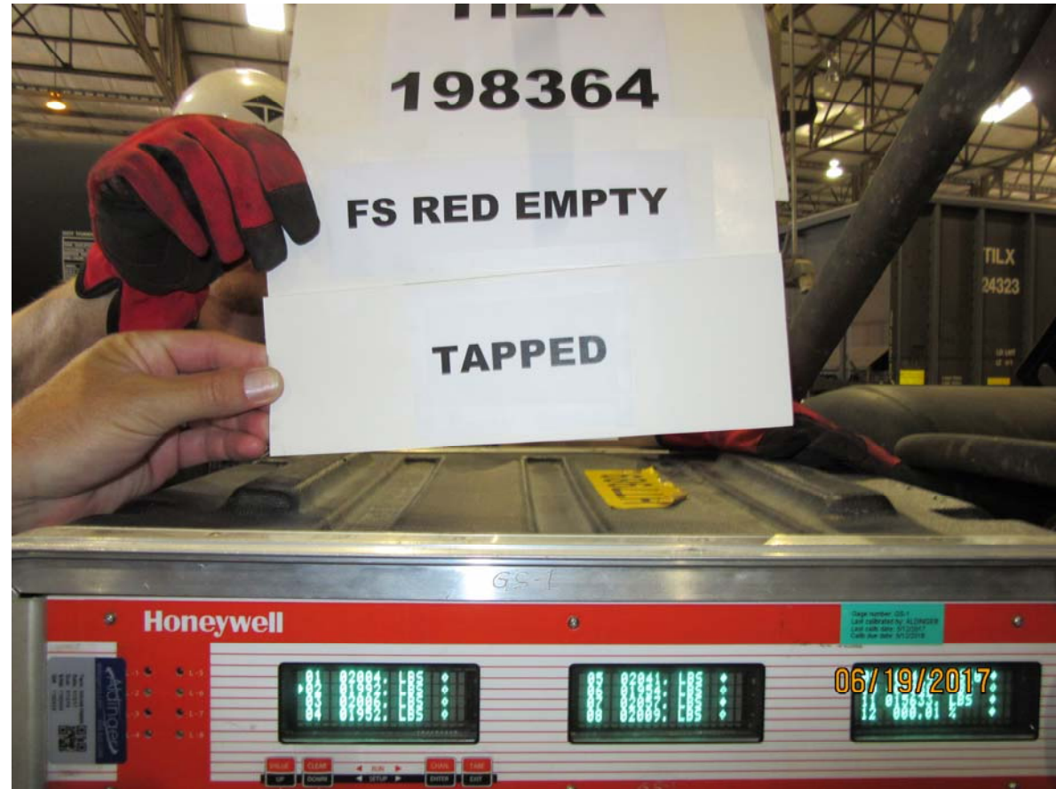
Figure 4318: TILX 198364, full service BPP reduction, empty car, brake shoe forces, brake pins tapped
