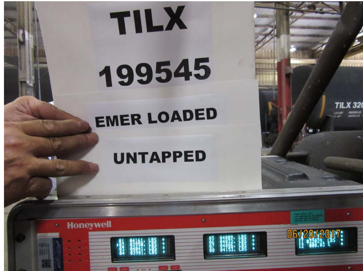
Figure 4358: TILX 199545, emergency BPP reduction, loaded car, brake shoe forces, brake pins untapped (Figure 4357 backup)
