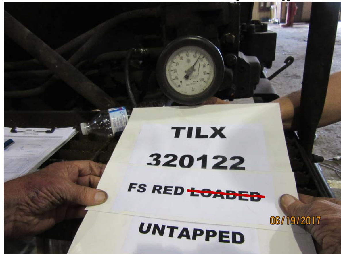
Figure 4333: TILX 320122, full service BPP reduction, car empty/loaded, BC pressure, brake pins untapped
