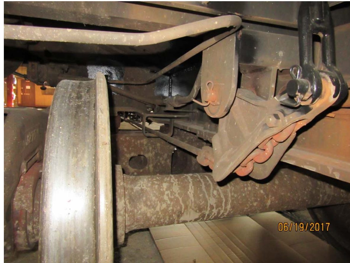
Figure 4234: TILX 199545, hand brake chain connection to input linkage
