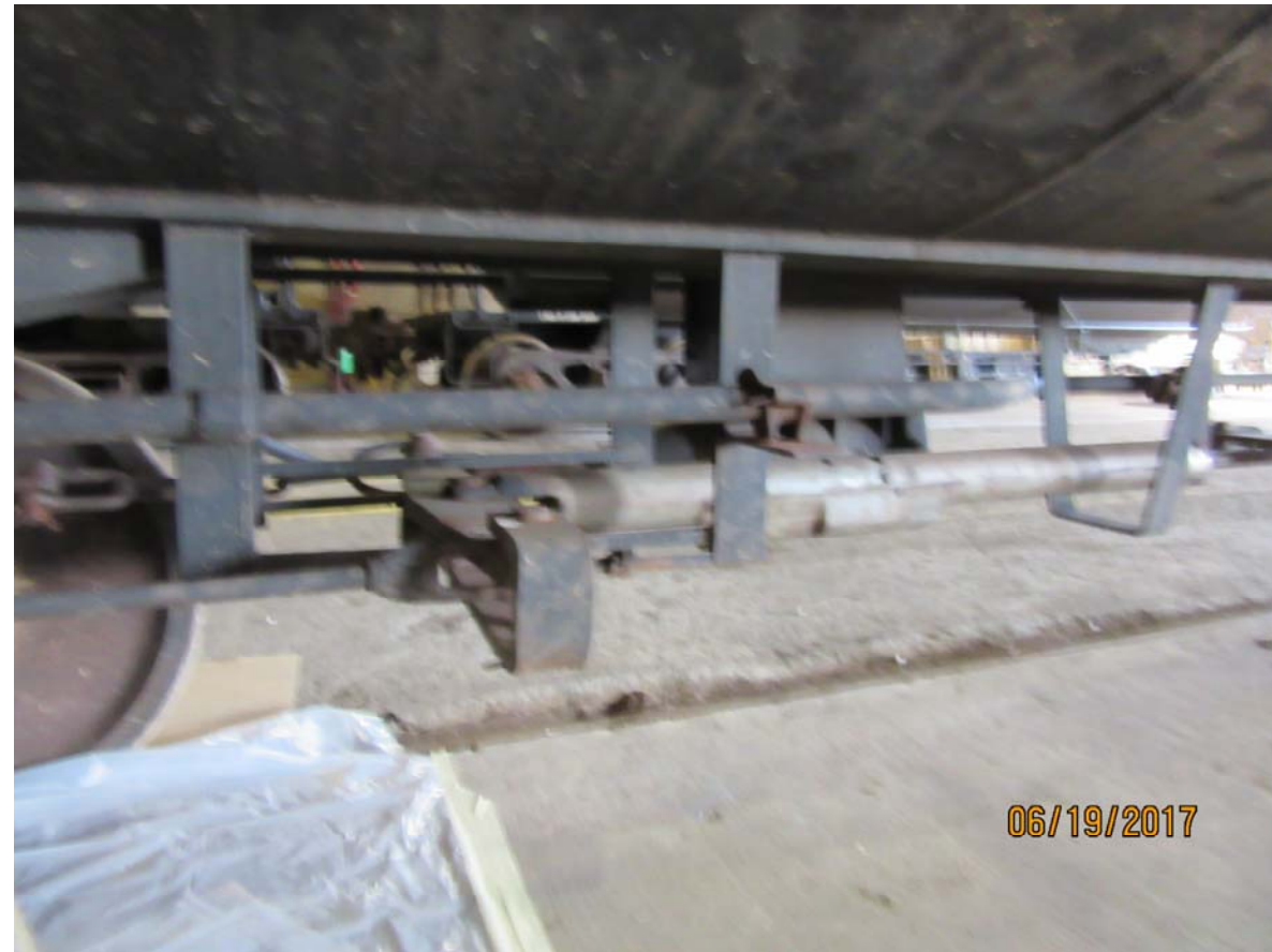
Figure 4250: TILX 320122, slack adjuster and mechanical linkages
