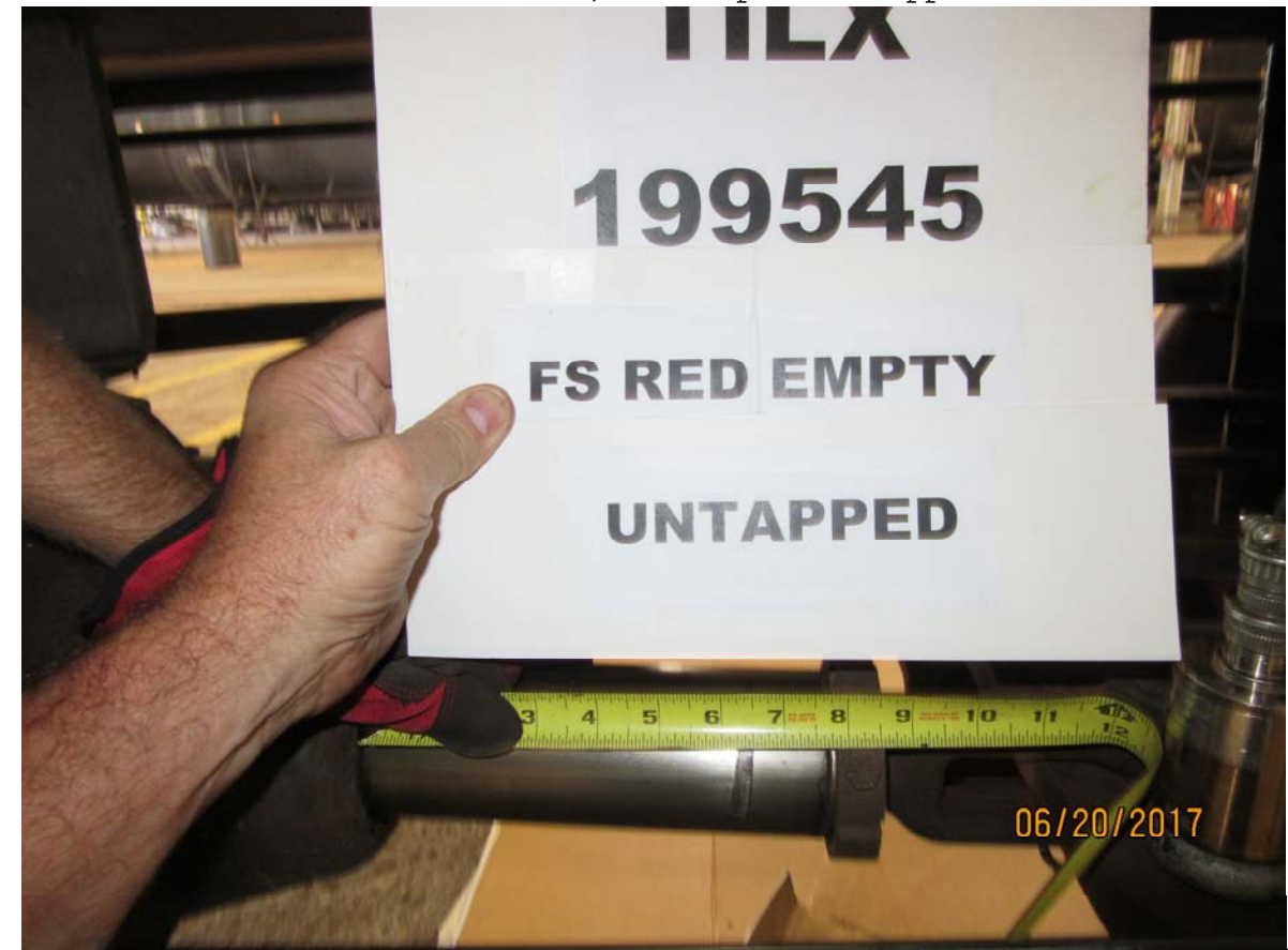
Figure 4365: TILX 199545, full service BPP reduction, empty car, BC piston length, brake pins untapped
