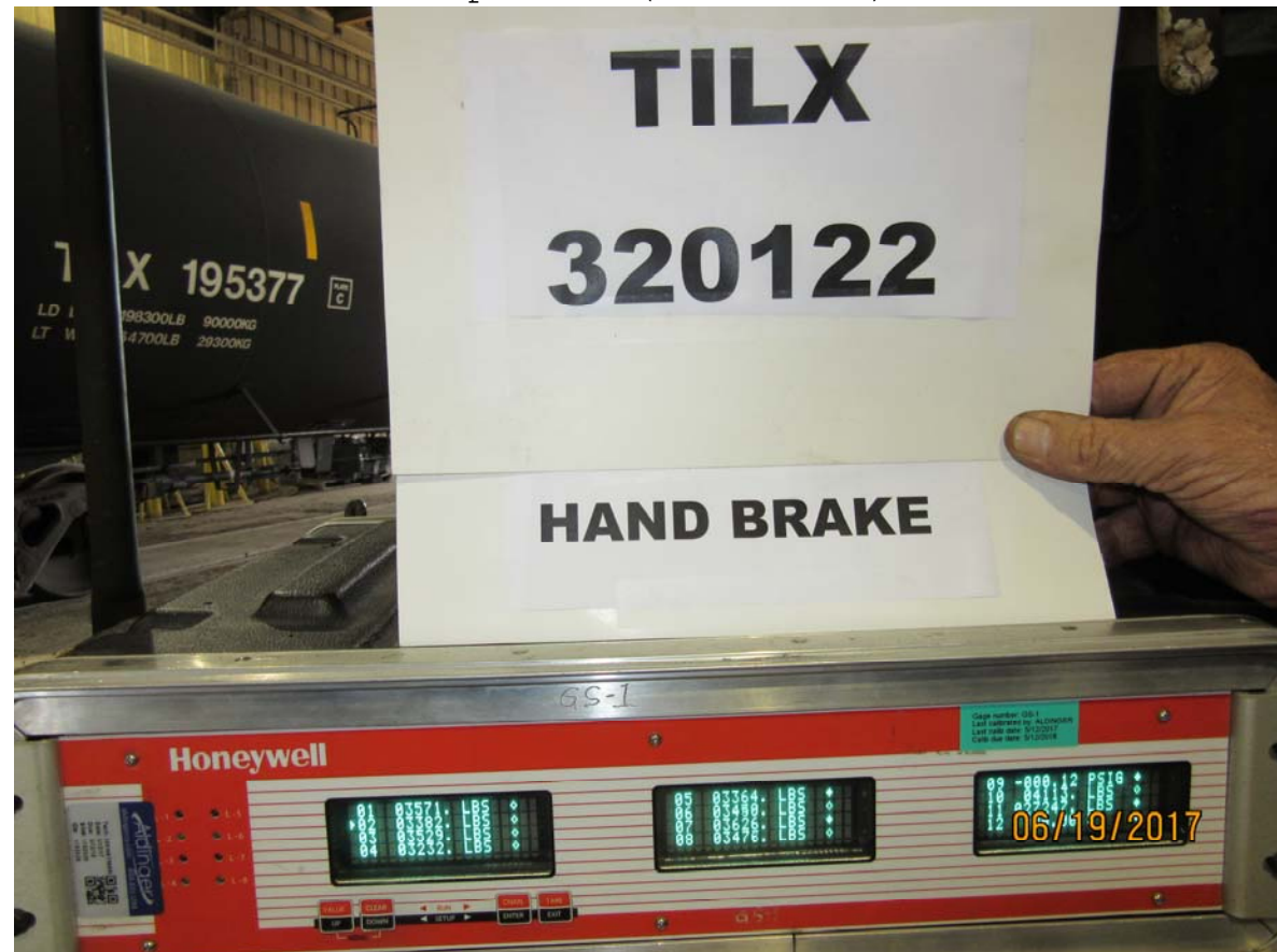
Figure 4329: TILX 320122, handbrake application, brake shoe forces, (channels 1-8 of 12 are L1, L2, L3, L4, R1, R2, R3, R4)
