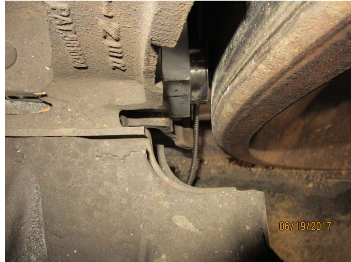
Figure 4290: TILX 198364, force transducer installed in nominal brake shoe position (view 1 of 2)
