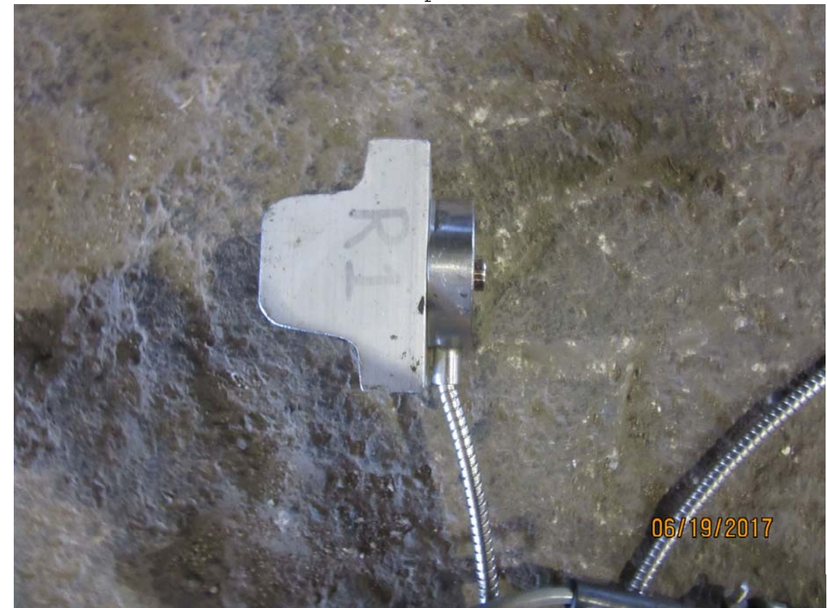
Figure 4288: TILX 198364, force transducer designed to measure equivalent brake shoe force (view 1 of 2)
