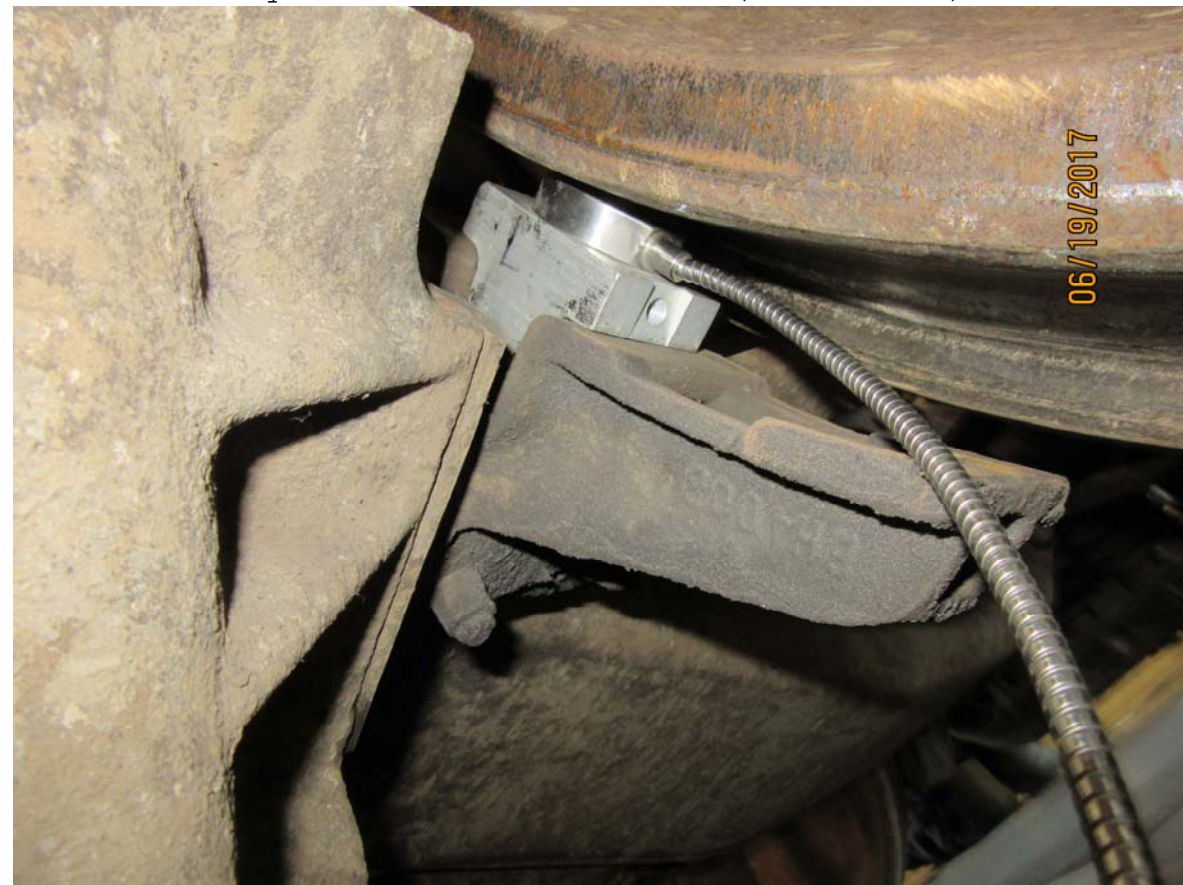
Figure 4291: TILX 198364, force transducer installed in nominal brake shoe position (view 2 of 2)
