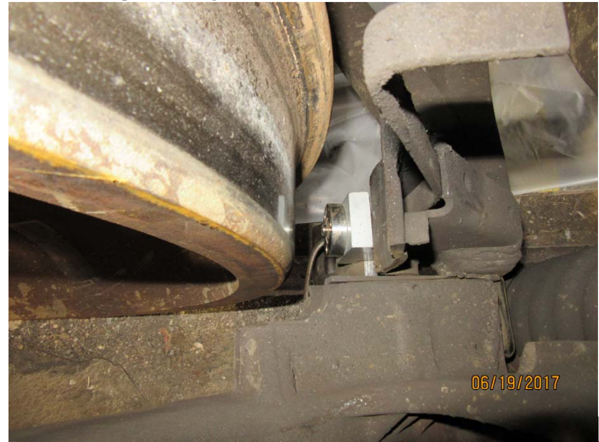
Figure 4326: TILX 320122, force transducer installed in nominal brake shoe position (view 2 of 4)
