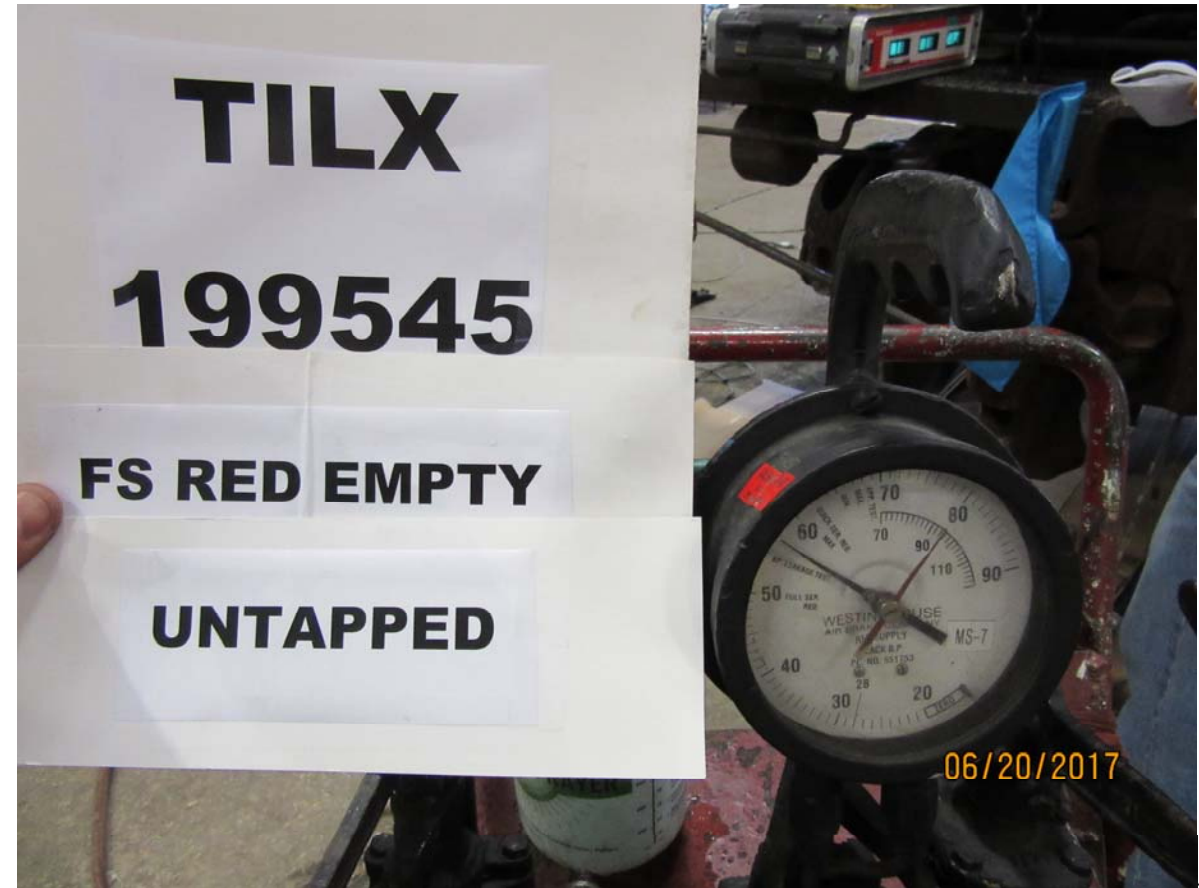
Figure 4367: TILX 199545, full service BPP reduction, empty car, brake pipe pressure, brake pins untapped
