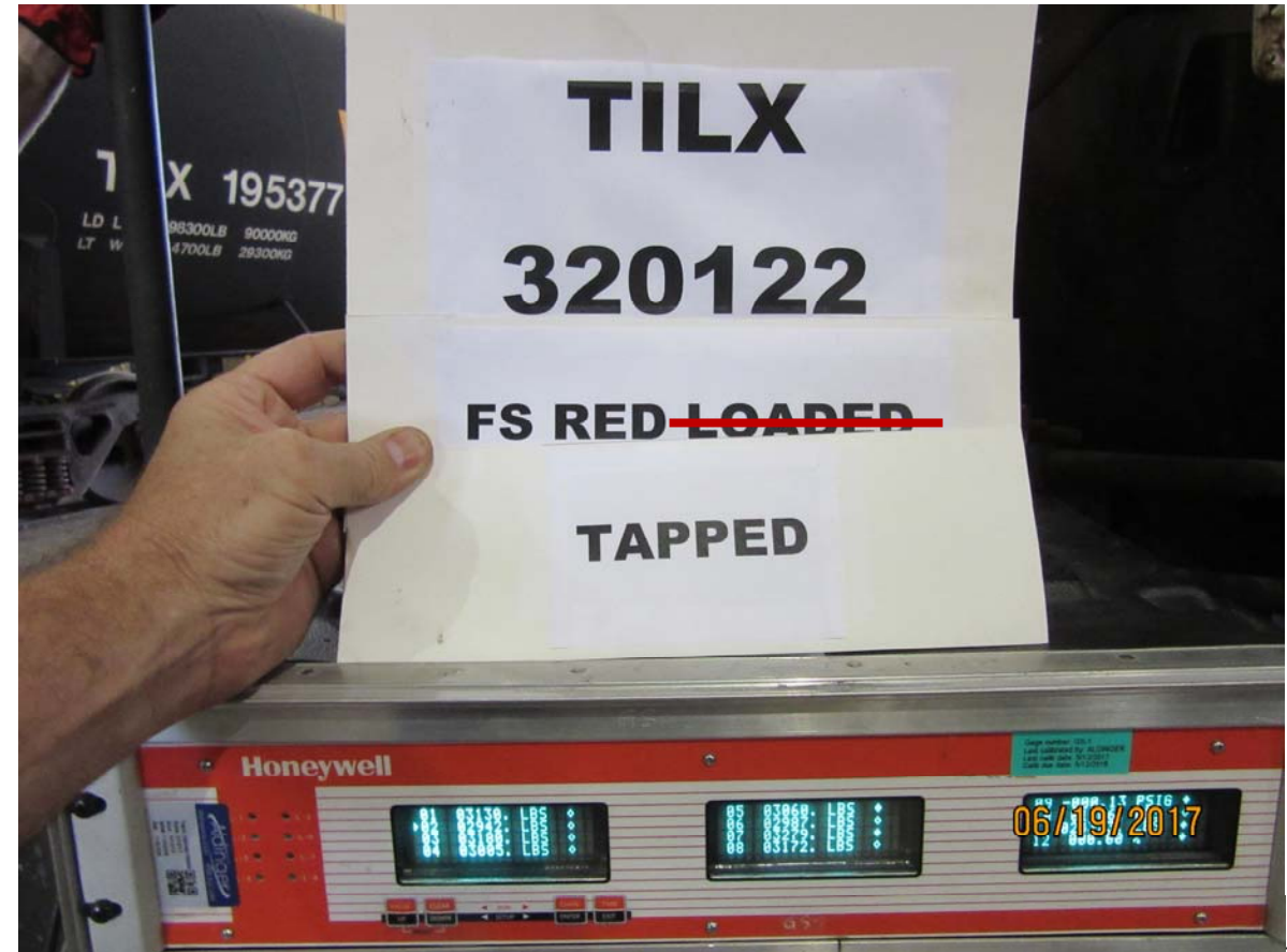
Figure 4336: TILX 320122, full service BPP reduction, car empty/loaded, brake shoe forces, brake pins tapped
