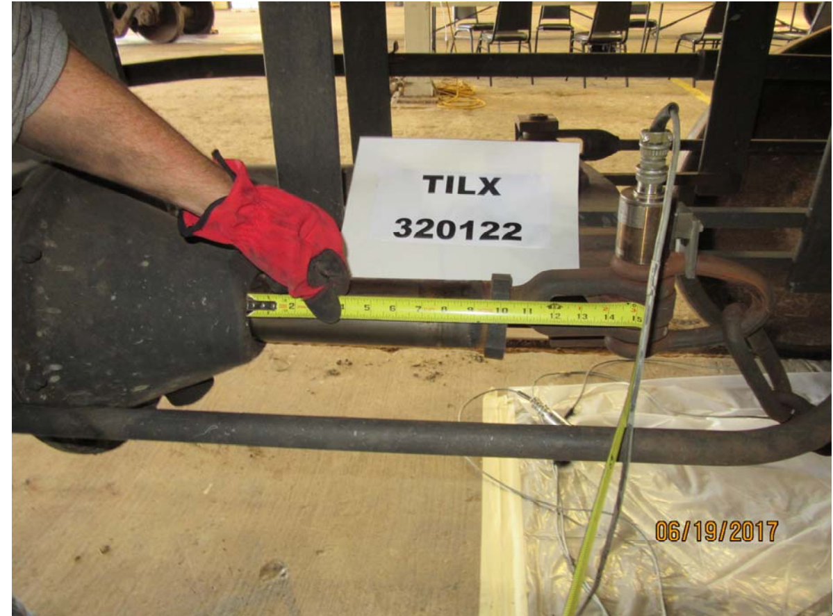
Figure 4324: TILX 320122, full service BPP reduction, brake cylinder piston length
