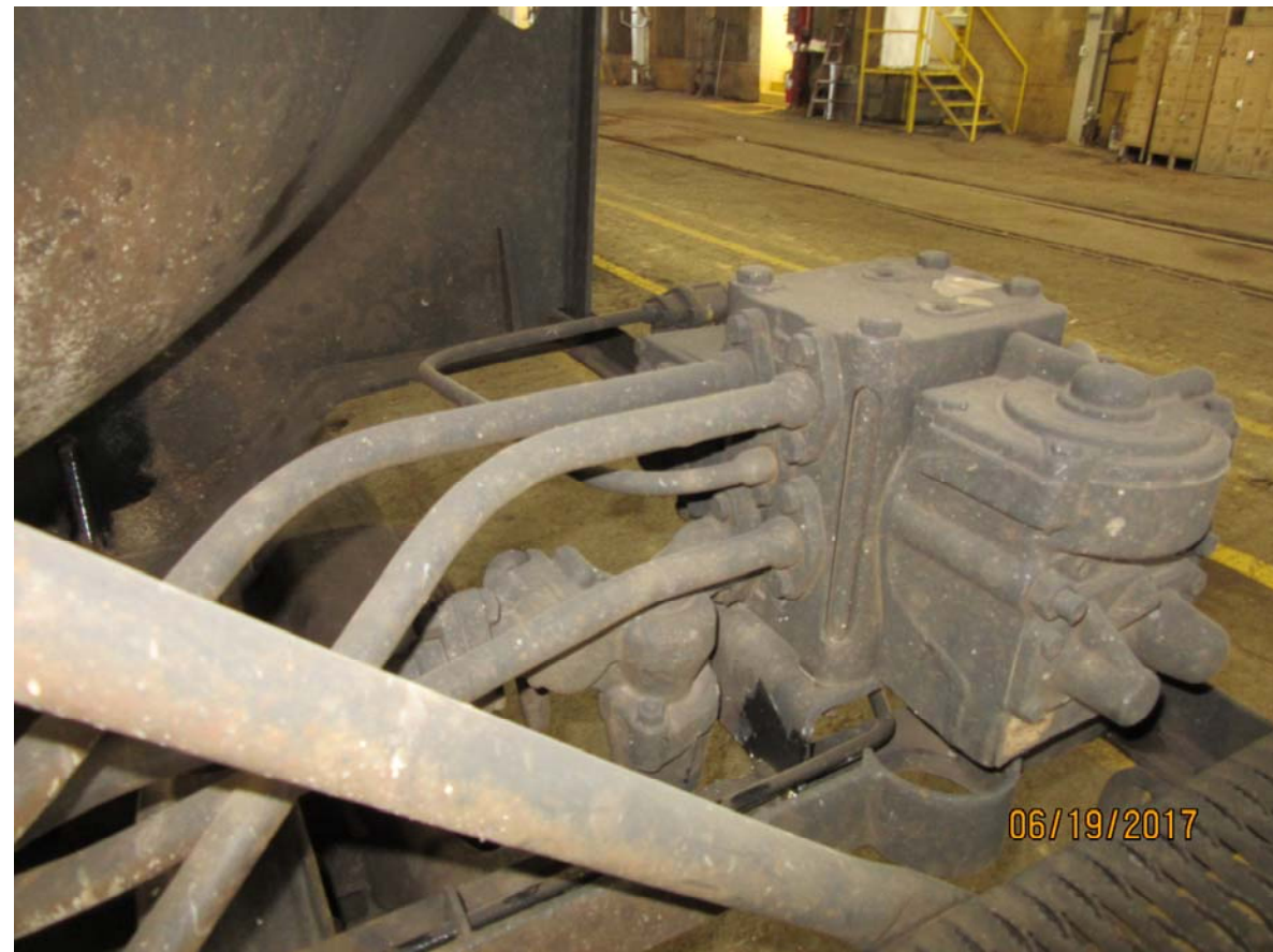
Figure 4264: TILX 198364, brake control valve
