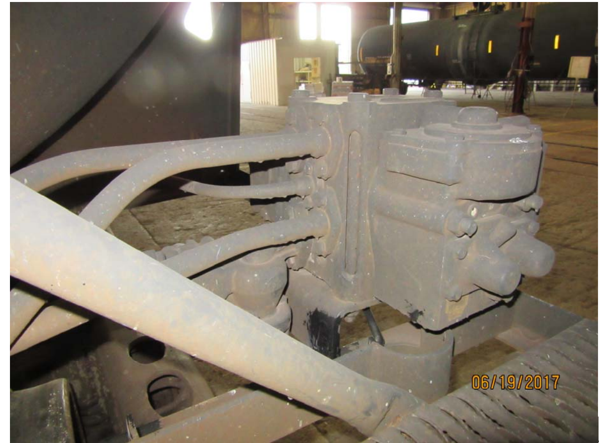
Figure 4235: TILX 199545, brake control valve
