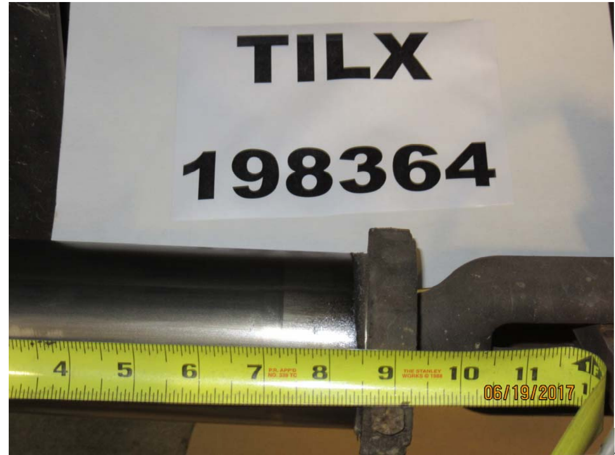
Figure 4282: TILX 198364, emergency BPP reduction, loaded car, BC piston length (Figure 4281 backup)
