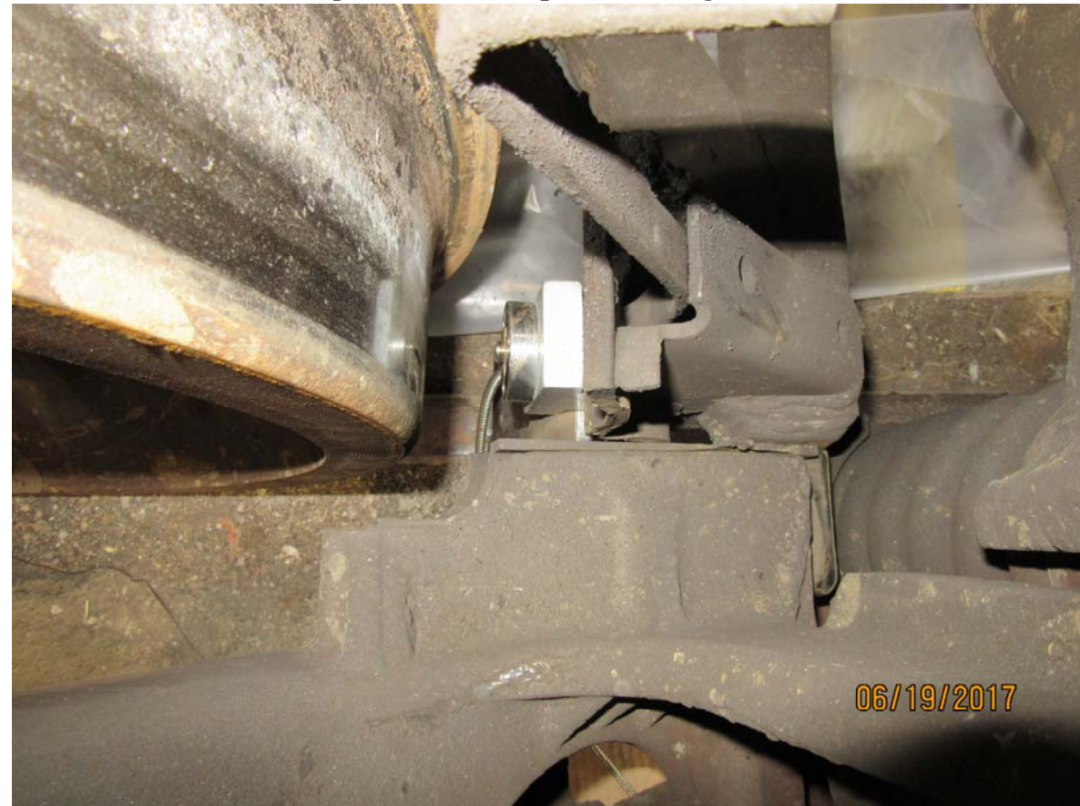
Figure 4325: TILX 320122, force transducer installed in nominal brake shoe position (view 1 of 4)
