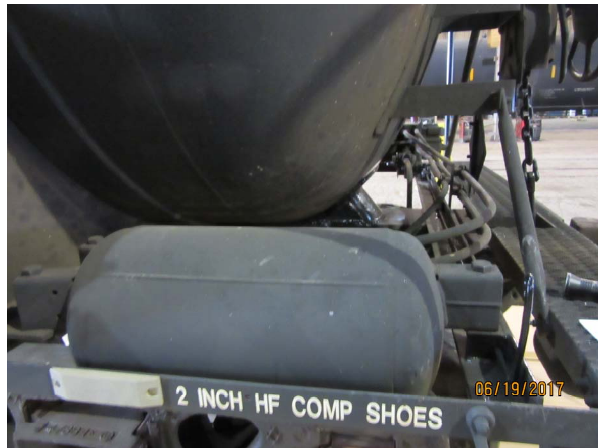
Figure 4232: TILX 199545, car air reservoir (auxiliary and emergency)
