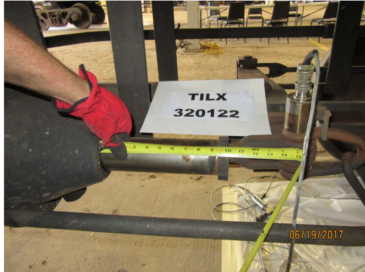
Figure 4323: TILX 320122, 20 pound brake pipe pressure (BPP) reduction, brake cylinder (BC) piston length
