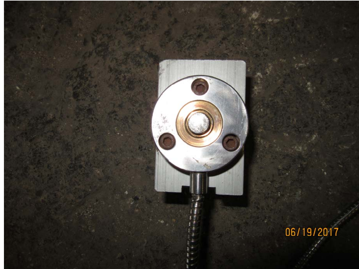
Figure 4289: TILX 198364, force transducer designed to measure equivalent brake shoe force (view 2 of 2)
