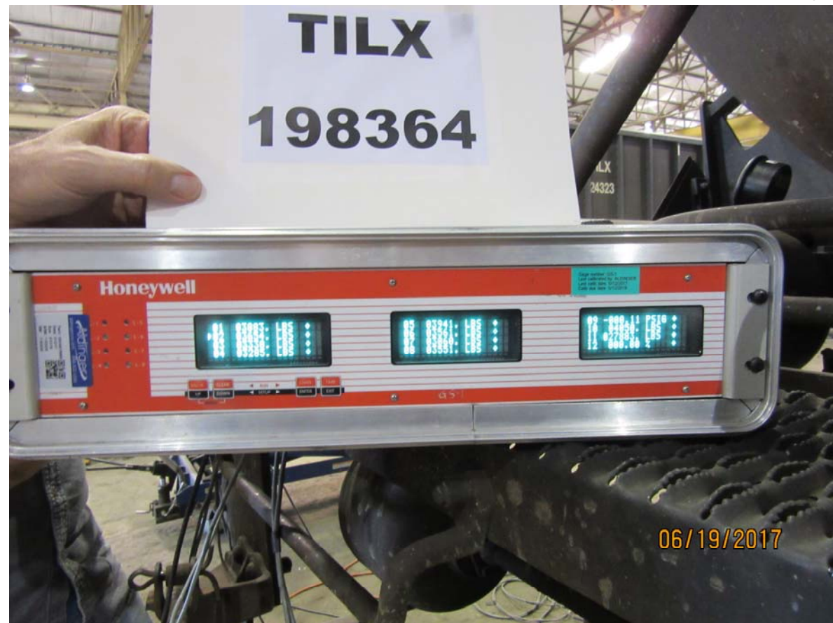
Figure 4293: TILX 198364, handbrake application, brake shoe forces, (channels 1-8 of 12 are L1, L2, L3, L4, R1, R2, R3, R4)
