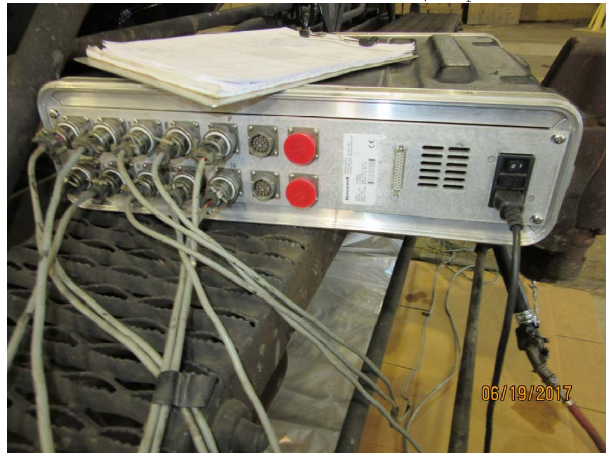
Figure 4287: TILX 198364, force and pressure data acquisition unit, transducer input arrangement, channels 1-10
