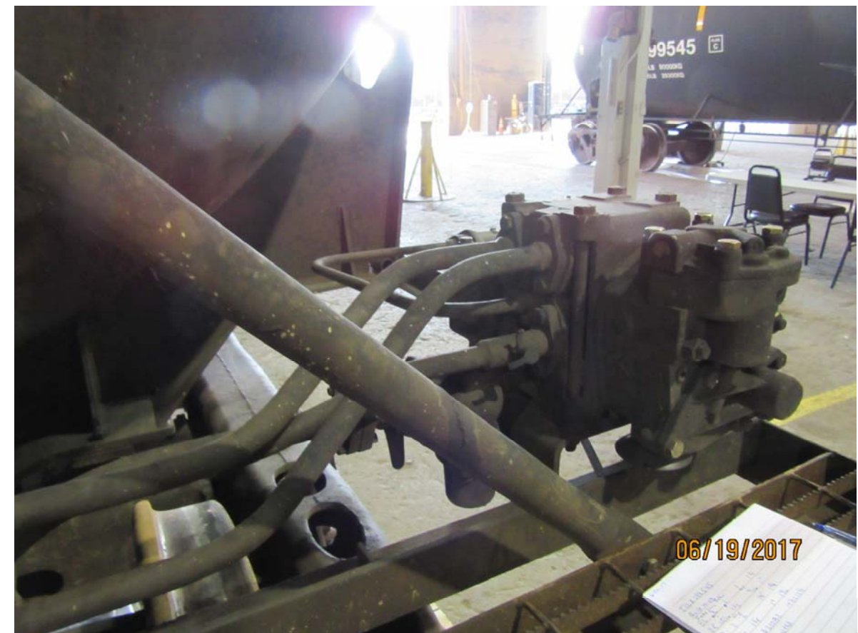
Figure 4245: TILX 320122, brake control valve
