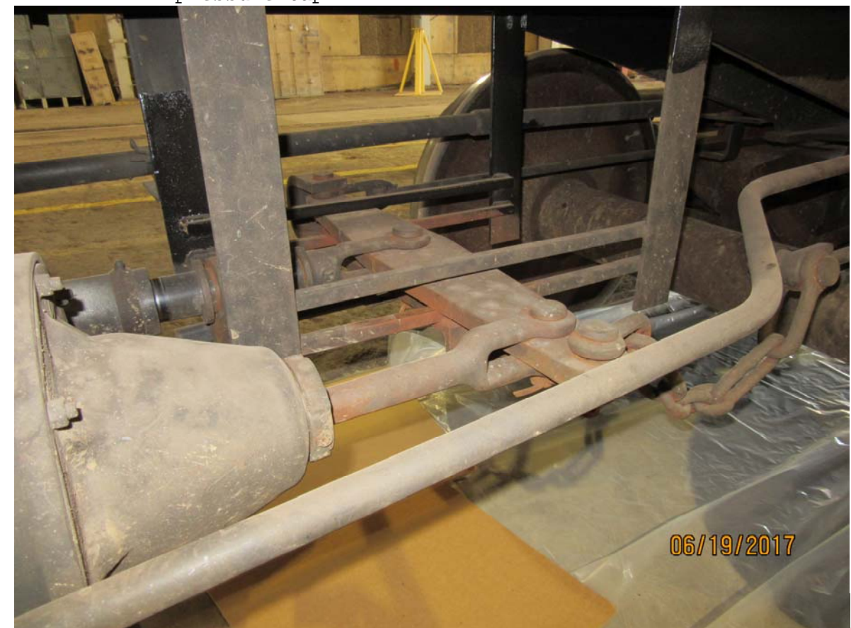
Figure 4261: TILX 198364, mechanical linkages to brake cylinder, handbrake, and slack adjuster with brake pin connections
