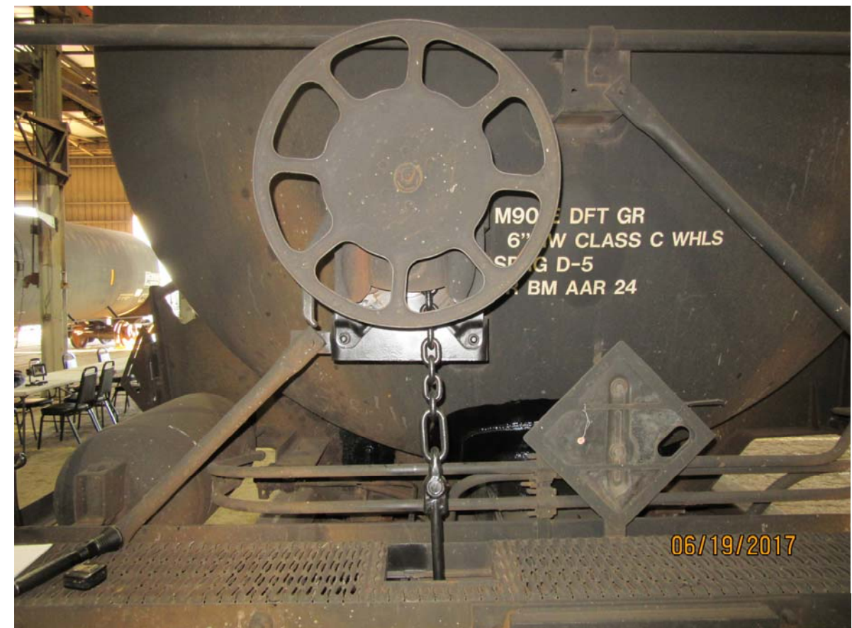
Figure 4233: TILX 199545, handbrake control wheel and chain
