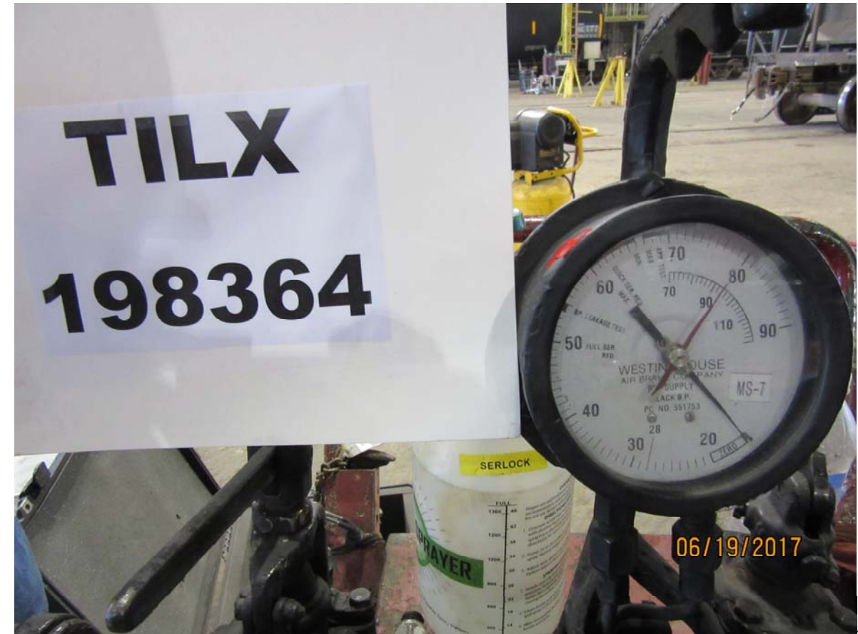
Figure 4306: TILX 198364, emergency BPP reduction, loaded car, brake pipe pressure
