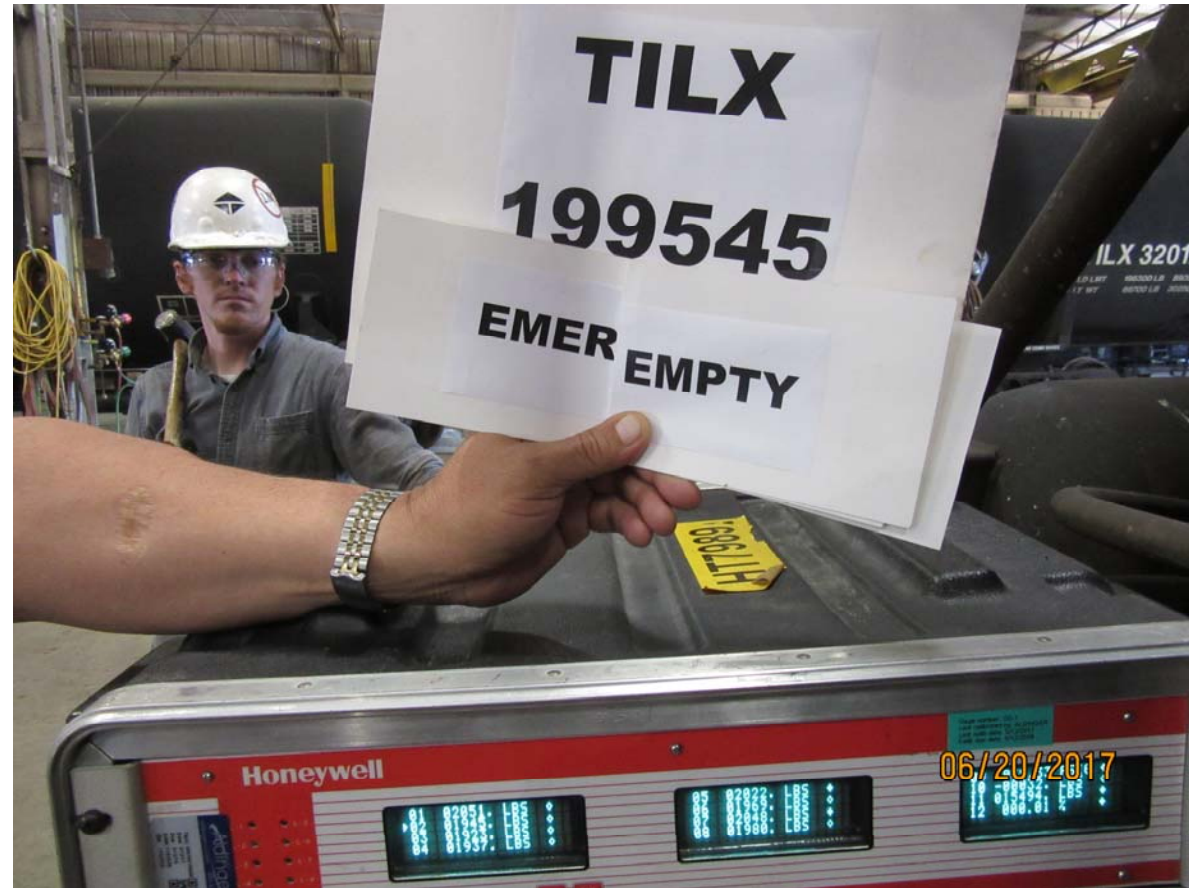
Figure 4374: TILX 199545, emergency BPP reduction, empty car, brake shoe forces, brake pins untapped
