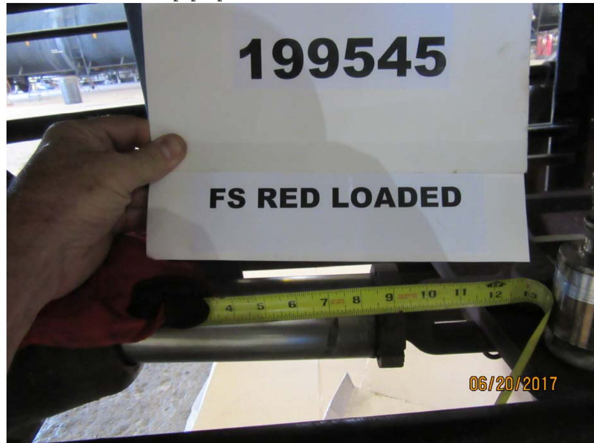
Figure 4344: TILX 199545, full service BPP reduction, loaded car, BC piston length (Figure 4343 backup)
