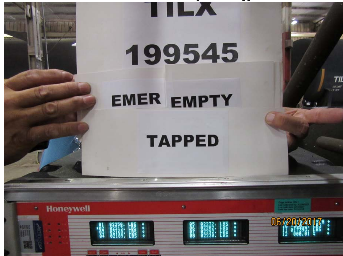
Figure 4376: TILX 199545, emergency BPP reduction, empty car, brake shoe forces, brake pins tapped
