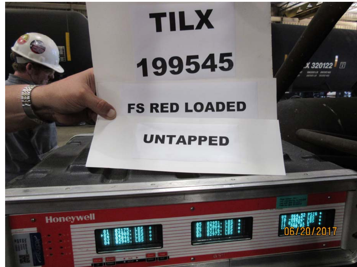
Figure 4353: TILX 199545, full service BPP reduction, loaded car, brake shoe forces, brake pins untapped
