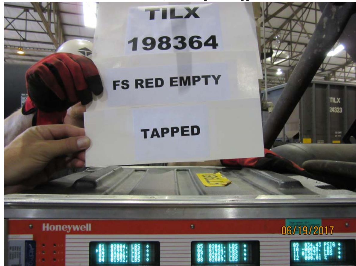
Figure 4319: TILX 198364, full service BPP reduction, empty car, brake shoe forces, brake pins tapped (Figure 4319 backup)
