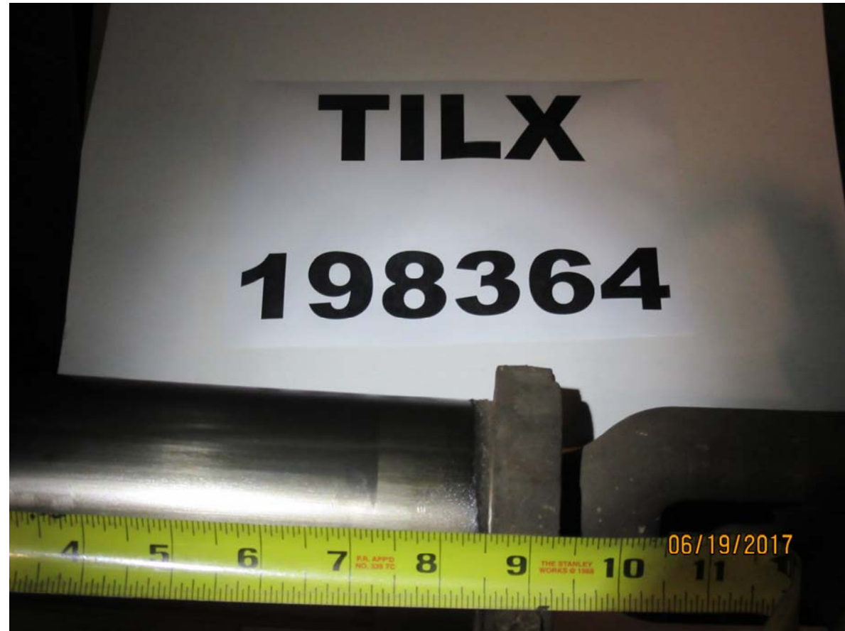
Figure 4281: TILX 198364, emergency BPP reduction, loaded car, BC piston length
