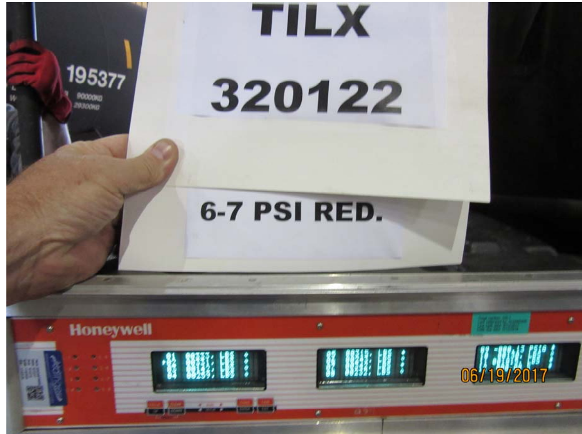
Figure 4331: TILX 320122, minimum service BPP reduction, car empty/loaded, brake shoe forces, brake pins untapped
