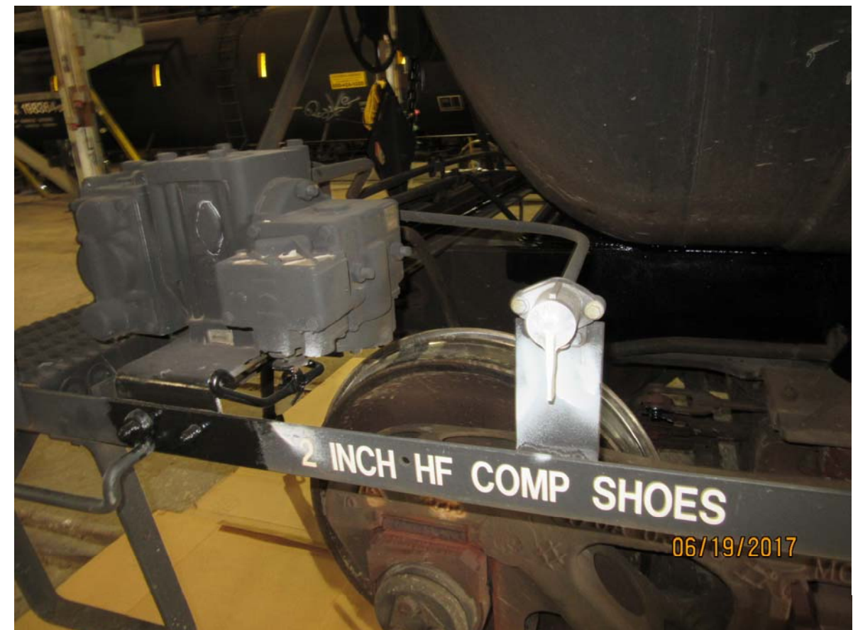
Figure 4237: TILX 199545, retainer valve
