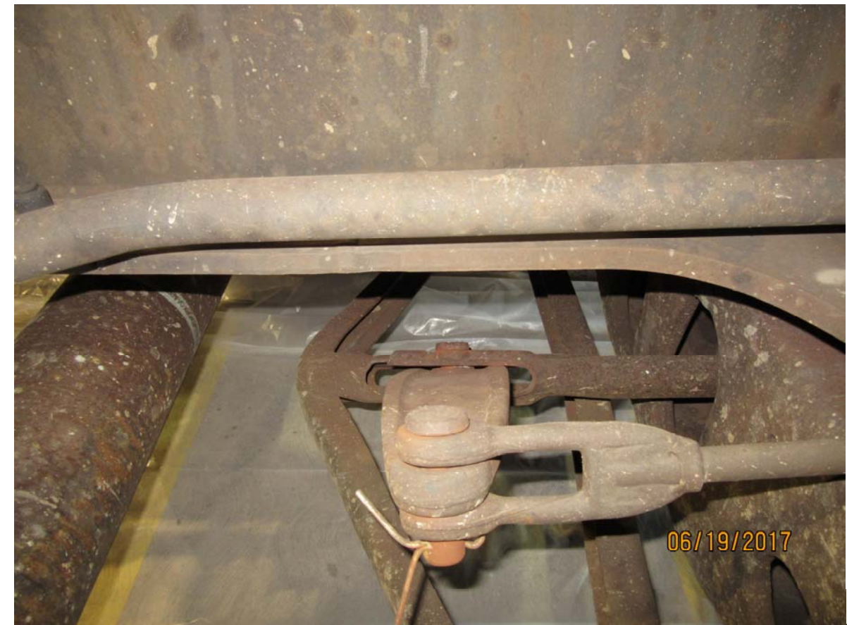
Figure 4249: TILX 320122, brake beam, brake pin, and mechanical linkages
