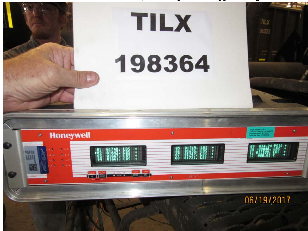
Figure 4315: TILX 198364, full service BPP reduction, empty car, brake shoe forces, brake pins untapped
