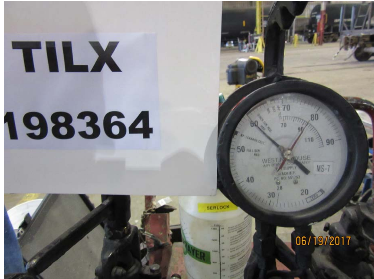
Figure 4301: TILX 198364, full service BPP reduction, loaded car, brake pipe pressure
