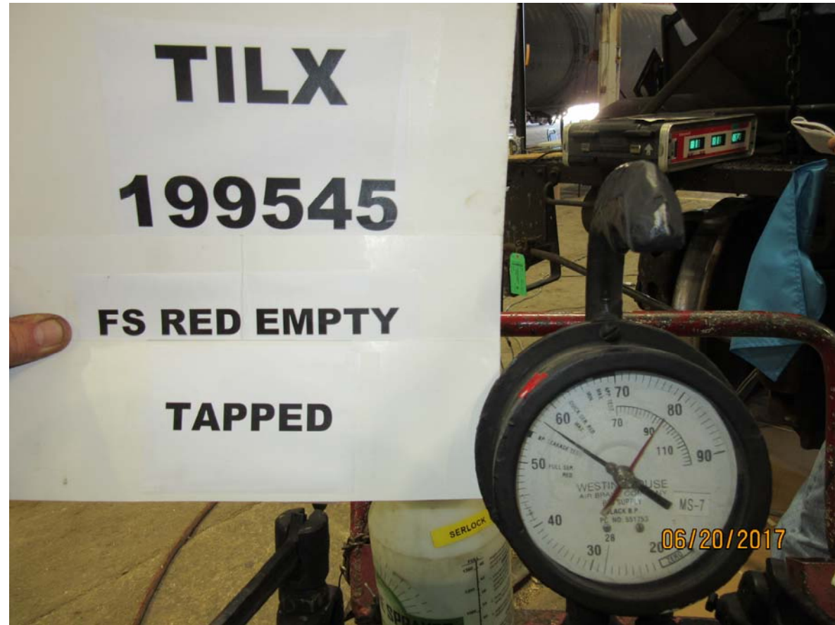
Figure 4370: TILX 199545, full service BPP reduction, empty car, brake pipe pressure, brake pins tapped
