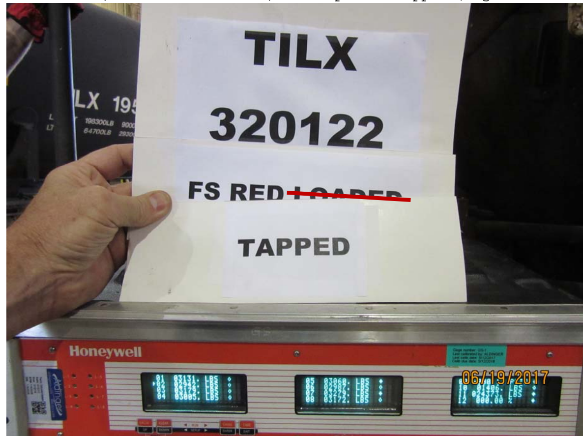
Figure 4337: TILX 320122, full service BPP reduction, car empty/loaded, brake shoe forces, brake pins tapped (Figure 4336 backup)
