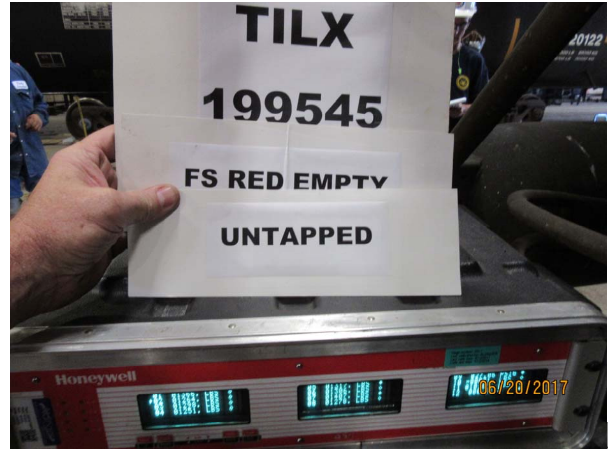
Figure 4363: TILX 199545, full service BPP reduction, empty car, brake shoe forces, brake pins untapped
