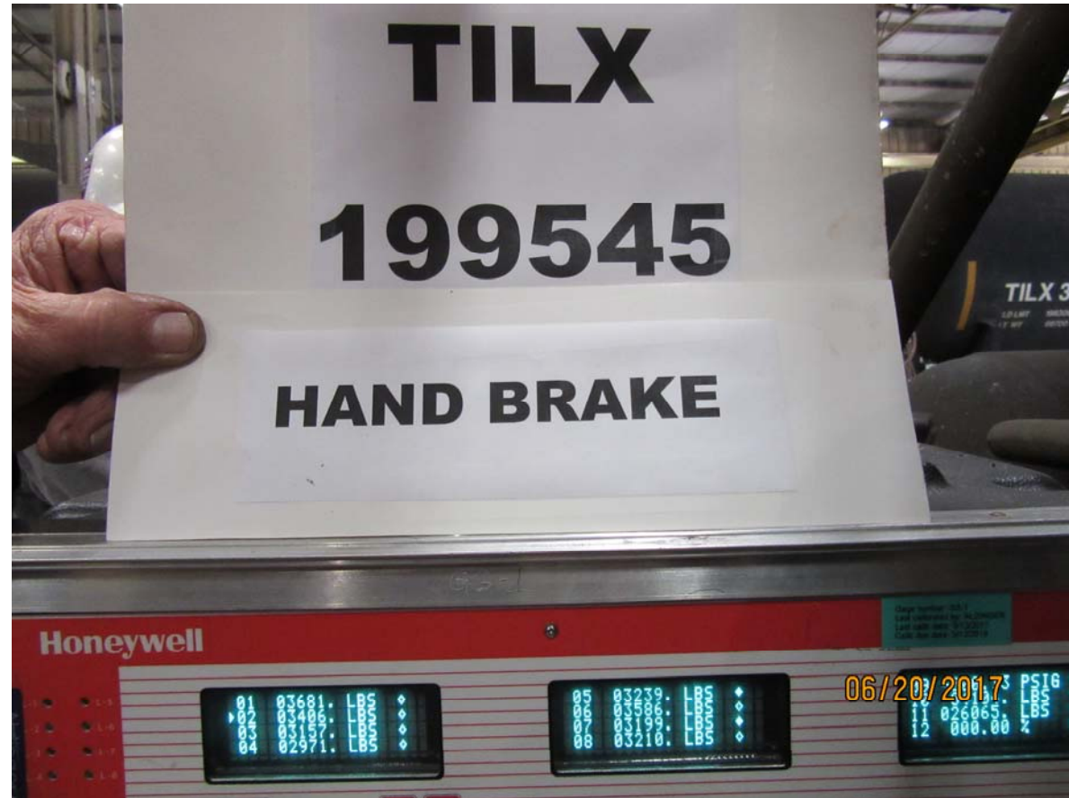
Figure 4346: TILX 199545, handbrake application, brake shoe forces, (channels 1-8 of 12 are L1, L2, L3, L4, R1, R2, R3, R4)
