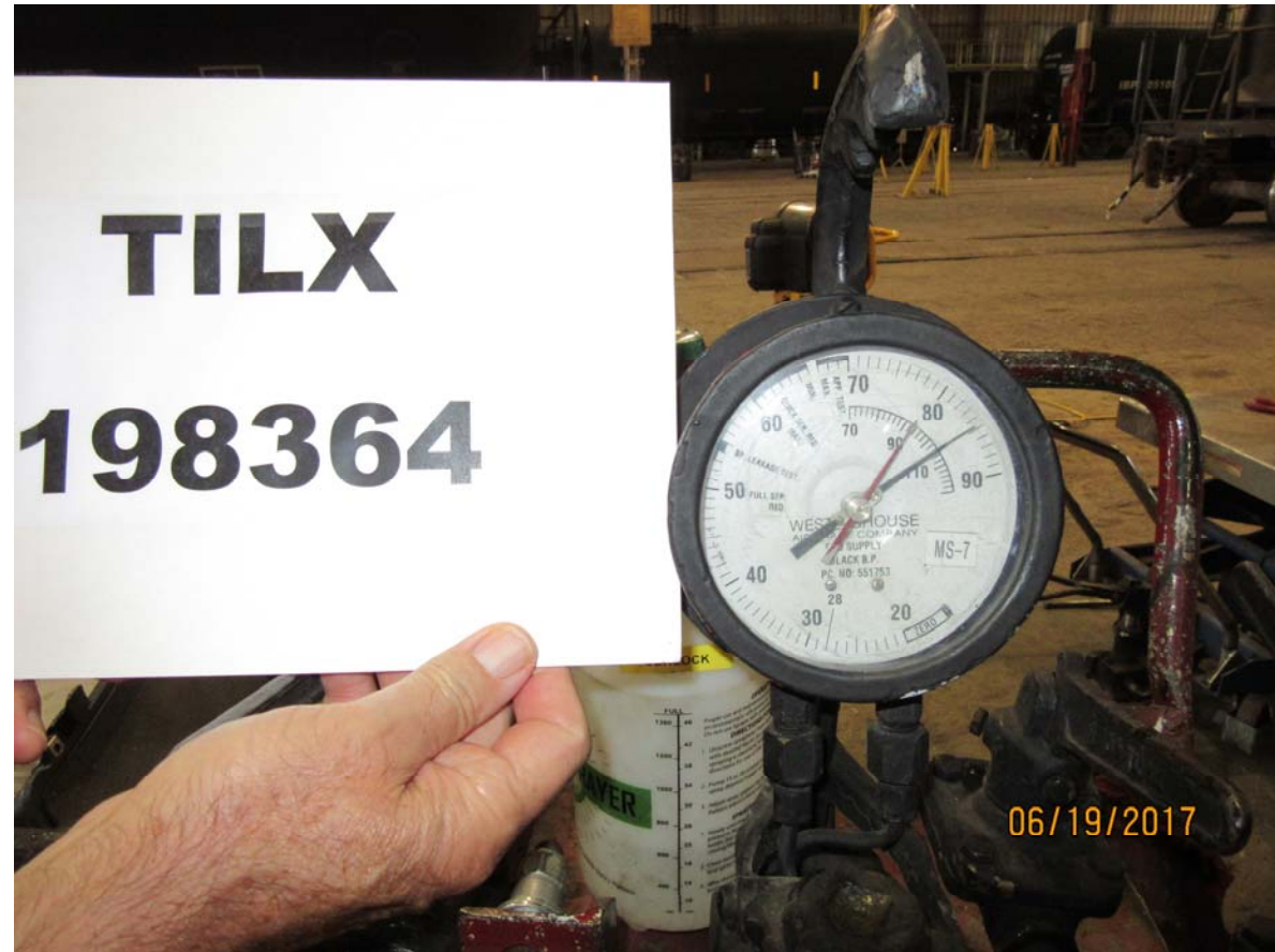
Figure 4297: TILX 198364, minimum service BPP reduction, loaded car, brake pipe pressure (Figure 4295 backup)
