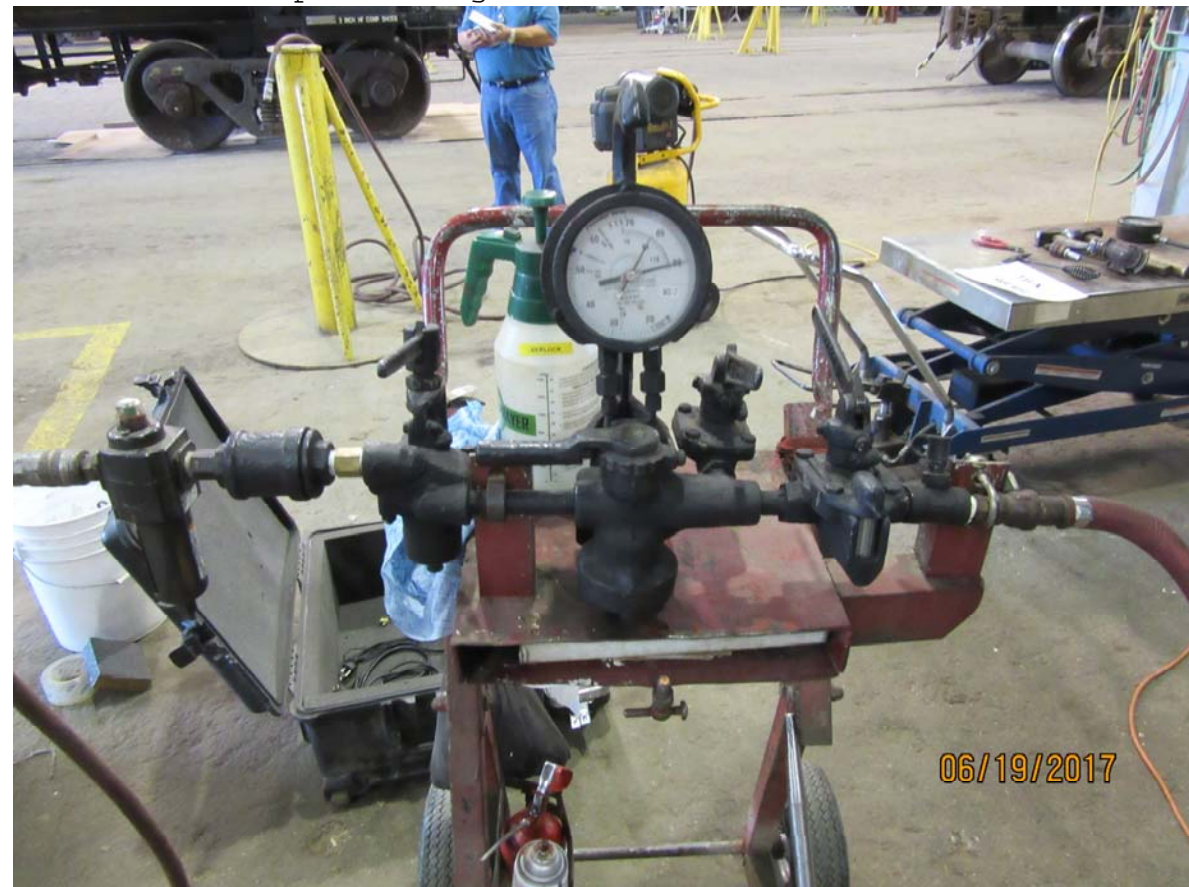
Figure 4283: TILX 198364, single car brake test stand
