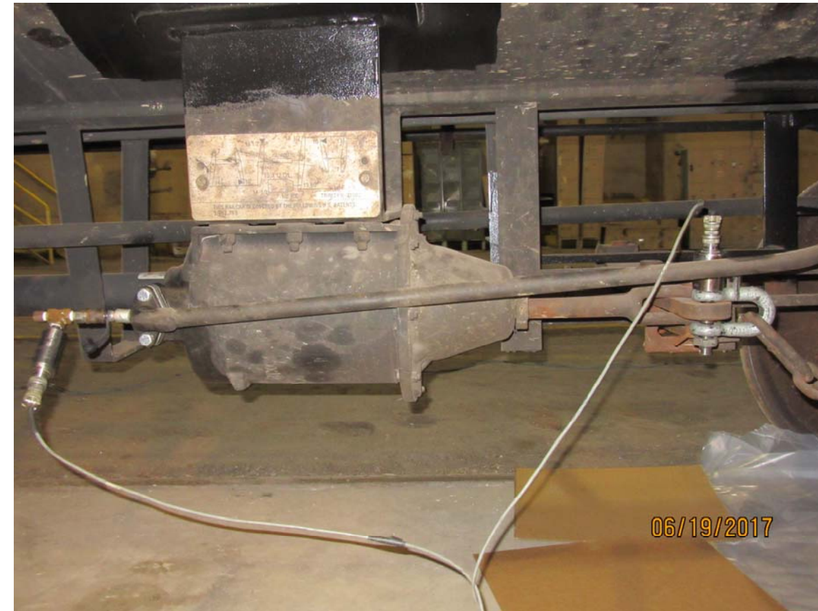
Figure 4275: TILX 198364, brake cylinder with test instrumentation to measure brake cylinder pressure and/or handbrake input force
