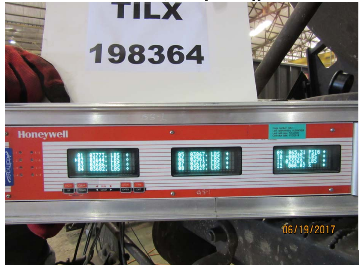
Figure 4304: TILX 198364, full service BPP reduction, loaded car, brake shoe forces, brake pins tapped
