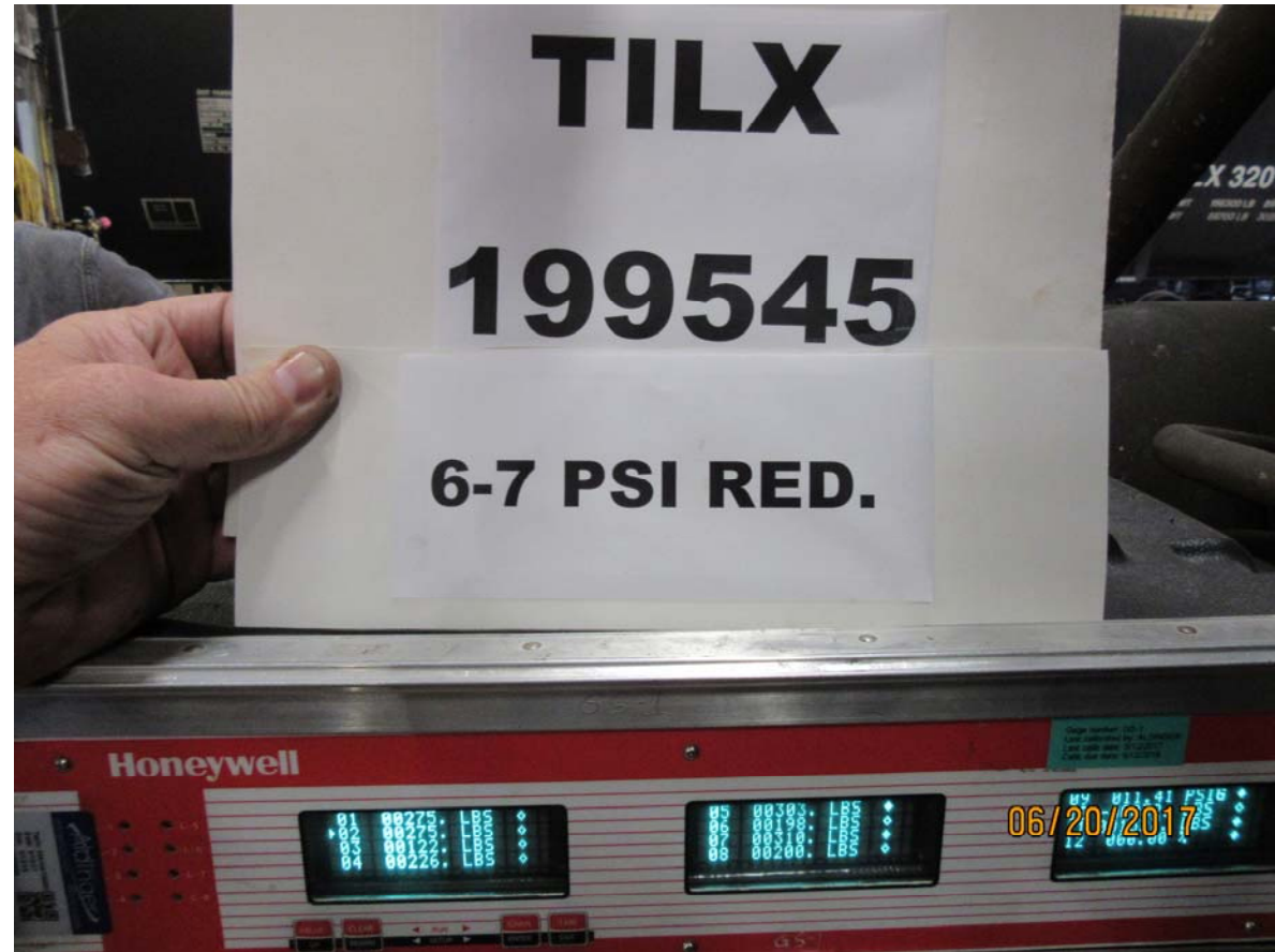
Figure 4350: TILX 199545, minimum service BPP reduction, loaded car, brake shoe forces, brake pins untapped (Figure 4349 backup)
