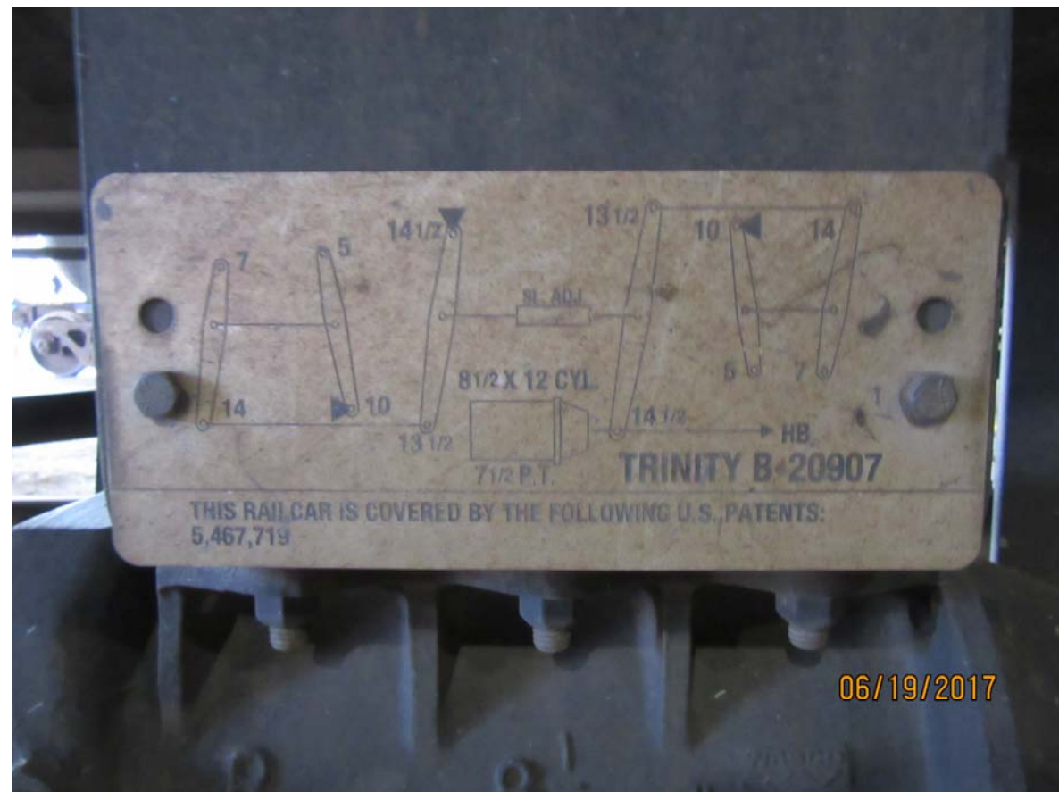
Figure 4252: TILX 320122, brake system mechanical linkage diagram
