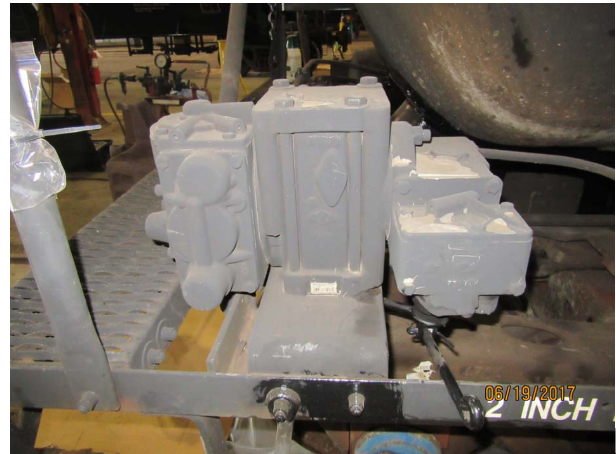
Figure 4265: TILX 198364, brake control valve
