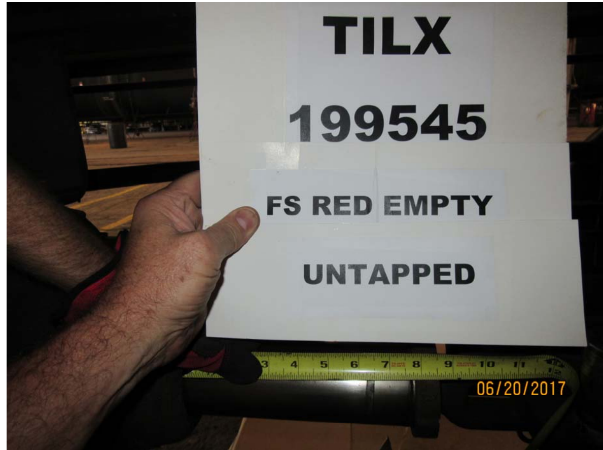
Figure 4366: TILX 199545, full service BPP reduction, empty car, BC piston length, brake pins untapped (Figure 4365 backup)
