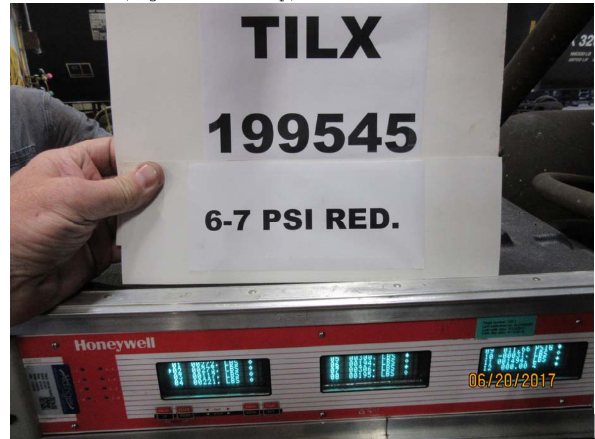
Figure 4349: TILX 199545, minimum service BPP reduction, loaded car, brake shoe forces, brake pins untapped
