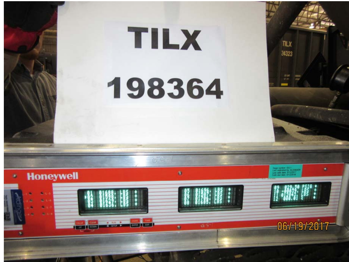
Figure 4313: TILX 198364, 20 pound BPP reduction, empty car, brake shoe forces, brake pins untapped (Figure 4312 backup)
