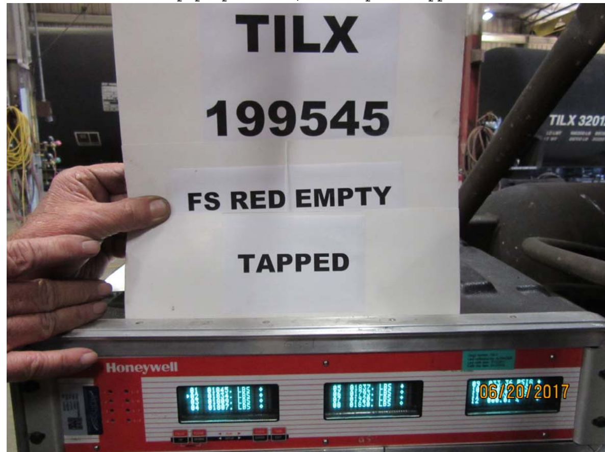
Figure 4372: TILX 199545, full service BPP reduction, empty car, brake shoe forces, brake pins tapped (Figure 4371 backup)
