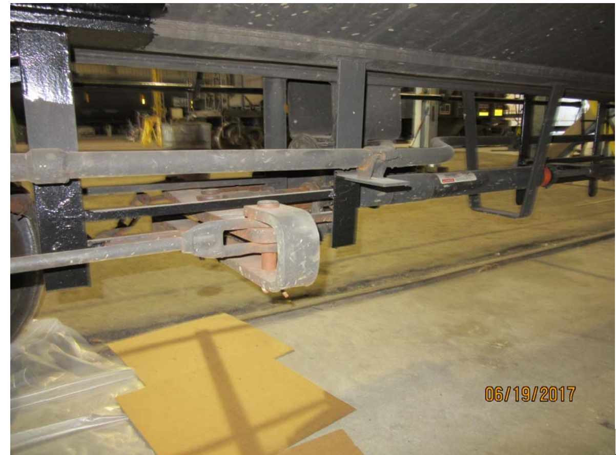
Figure 4269: TILX 198364, slack adjuster and mechanical linkages
