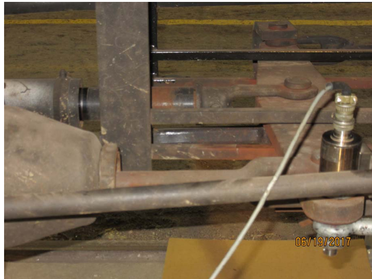
Figure 4276: TILX 198364, force transducer "smart" pin mounted to measure handbrake control input force
