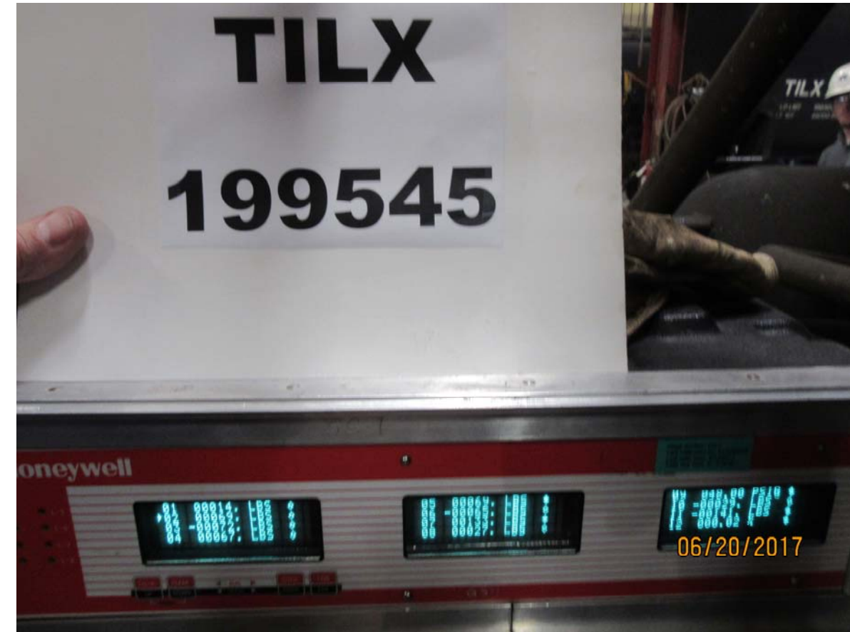
Figure 4339: TILX 199545, 20 pound BPP reduction, loaded car, brake cylinder (BC) pressure (channel 9 of 12)
