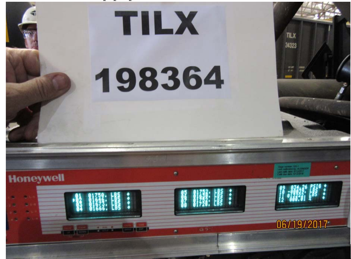
Figure 4316: TILX 198364, full service BPP reduction, empty car, brake shoe forces, brake pins untapped (Figure 4315 backup)
