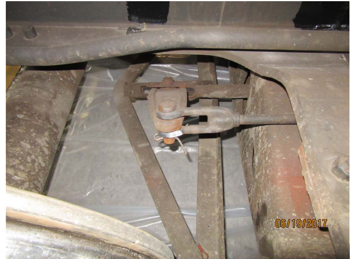
Figure 4267: TILX 198364, brake beam, pins, and mechanical linkages
