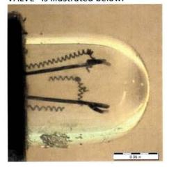
The filament in the bulb identified as #1 UNLOCK was difficult to see clearly so the glass envelope was removed to reveal the stretched filament illustrated below.
