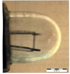
The bulbs identifies as "#1 BLEED VALVE", #2 BLEED VALVE" and "#2 UNLOCK displayed broken coils and #2 BLEED VALVE" is illustrated below.
