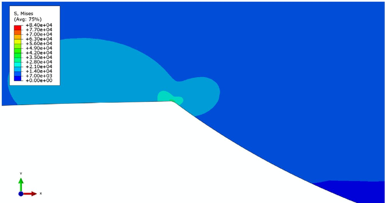
Figure 13. Contours of Mises stress at one interior corner of the weld bead in Model 1, at an internal pressure of 375 psi. Magnified 6 times with respect to figure 12.
