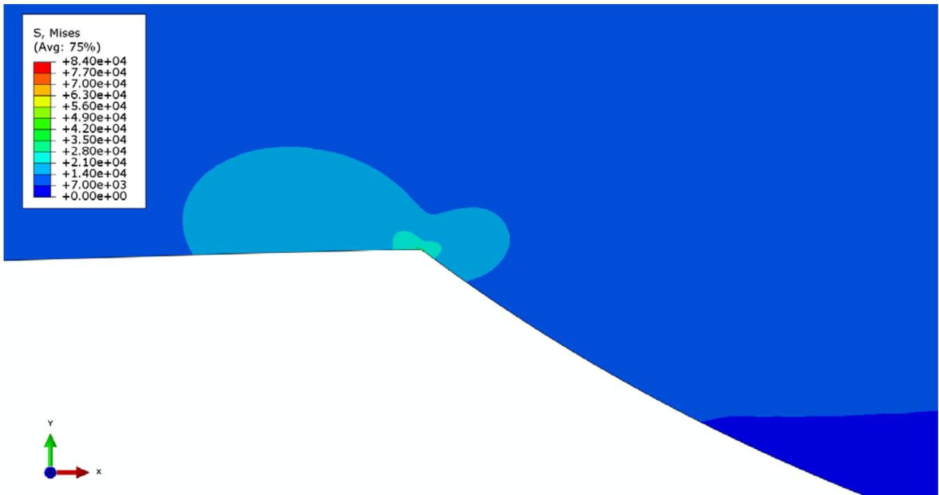
Figure 11. Contours of Mises stress at one interior corner of the weld bead in Model 1, at an internal pressure of 350 psi. Magnified 6 times with respect to figure 10.
