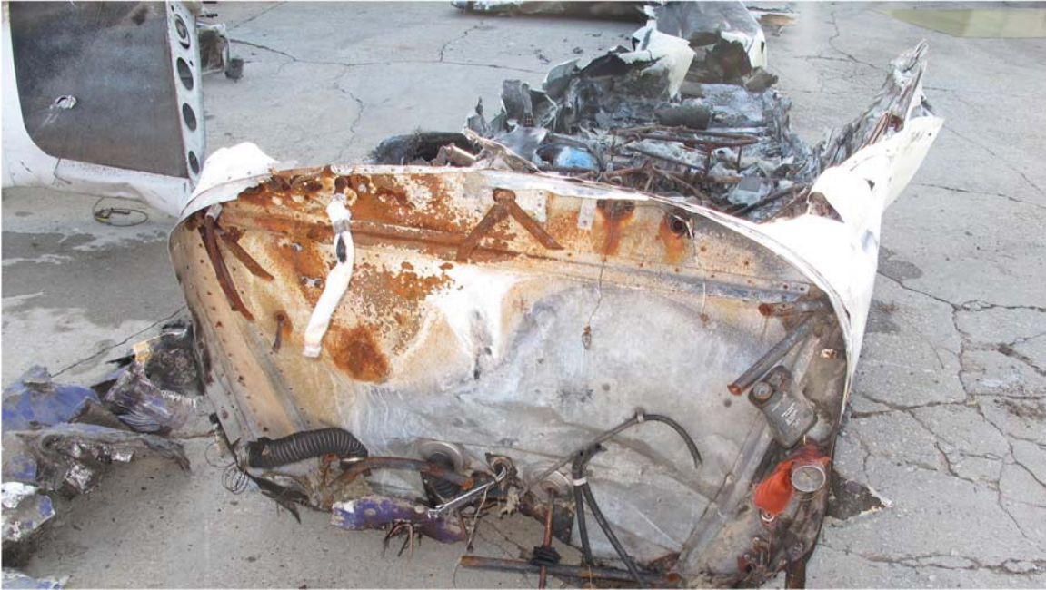
Figure 9. Photograph of forward surface of engine compartment firewall.
