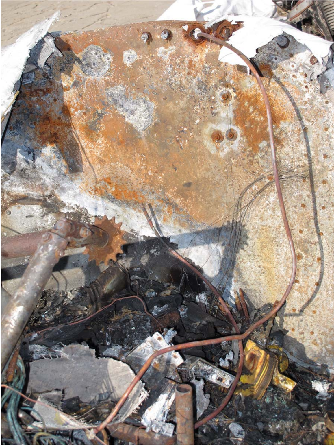
Figure 22. Photograph of aft surface of engine compartment firewall (cargo compartment forward wall).
