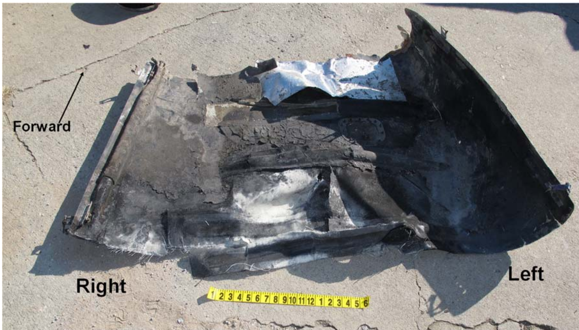
Figure 17. Photograph of lower surface of upper engine cowling.
