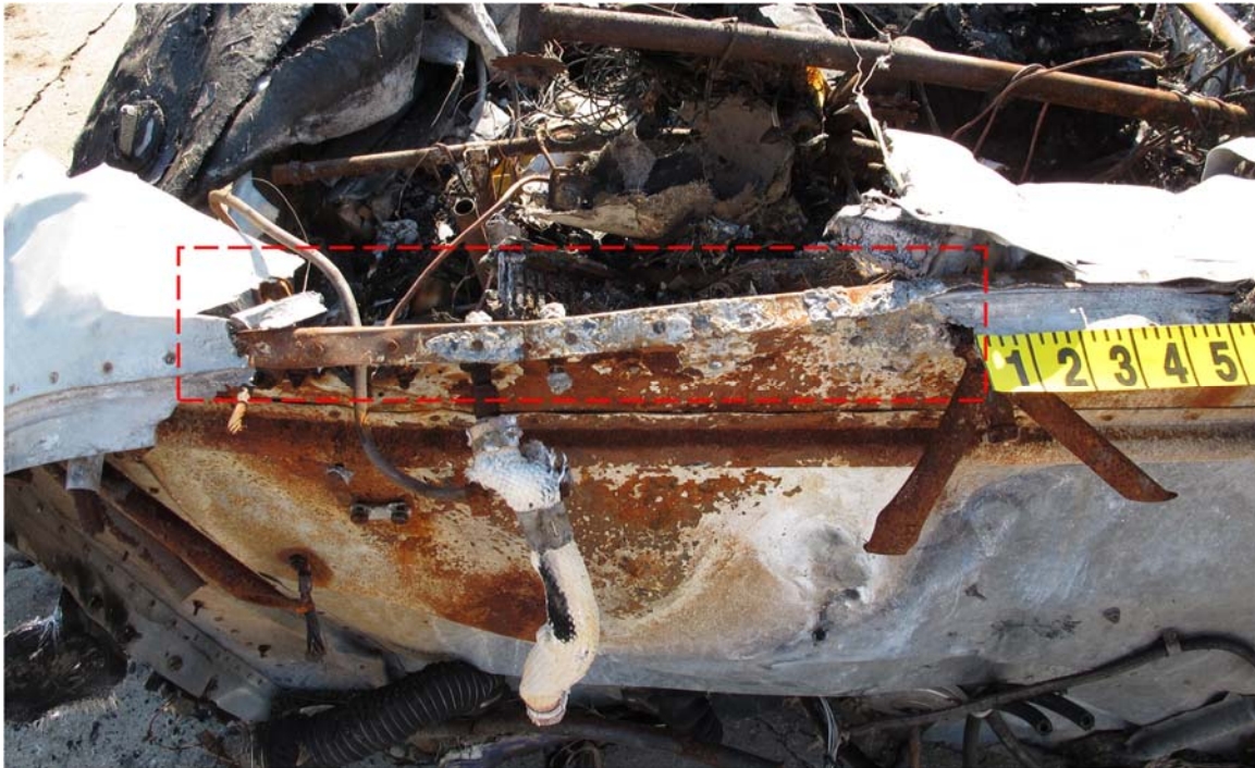
Figure 11. Photograph of missing section of aluminum strip (highlighted by the red box).
