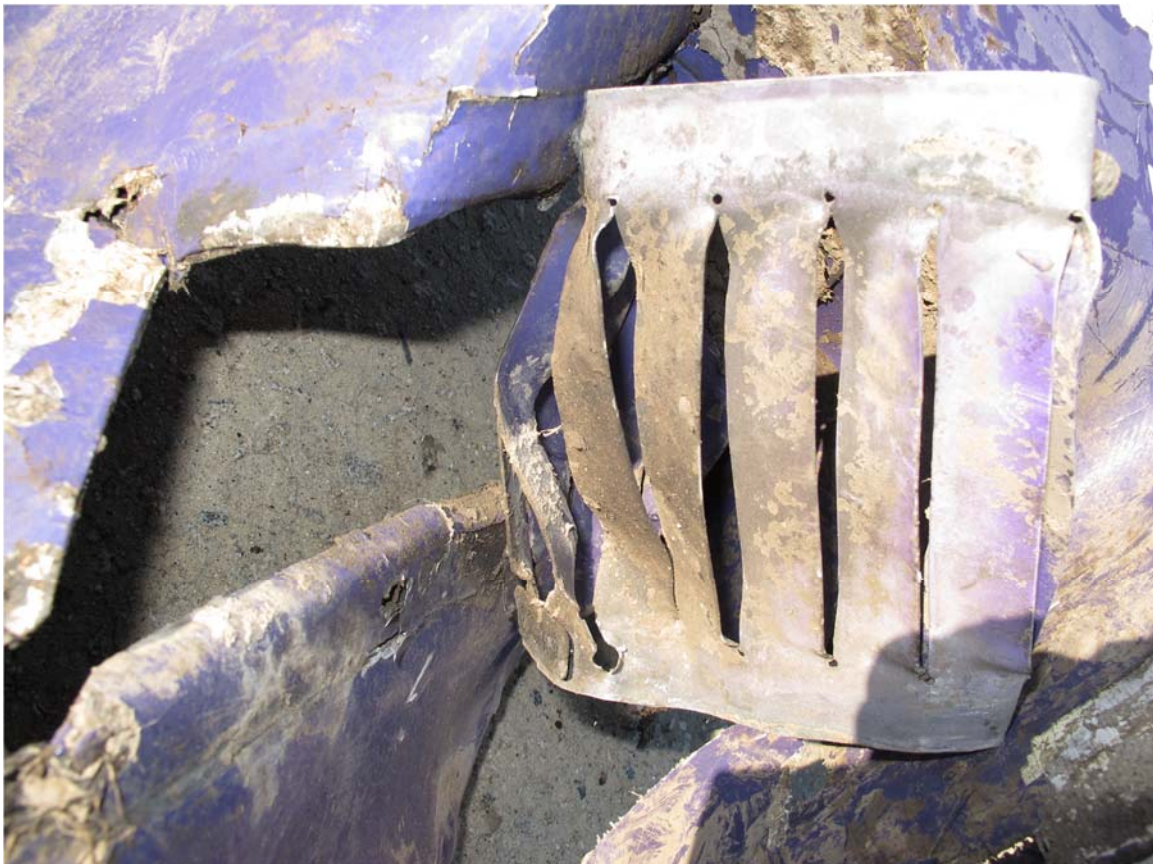
Figure 19. Photograph of lower right cowling exhaust louver.
