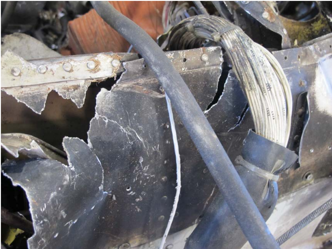
Figure 8. Closeup photograph of thermal tearing on right wing root.
