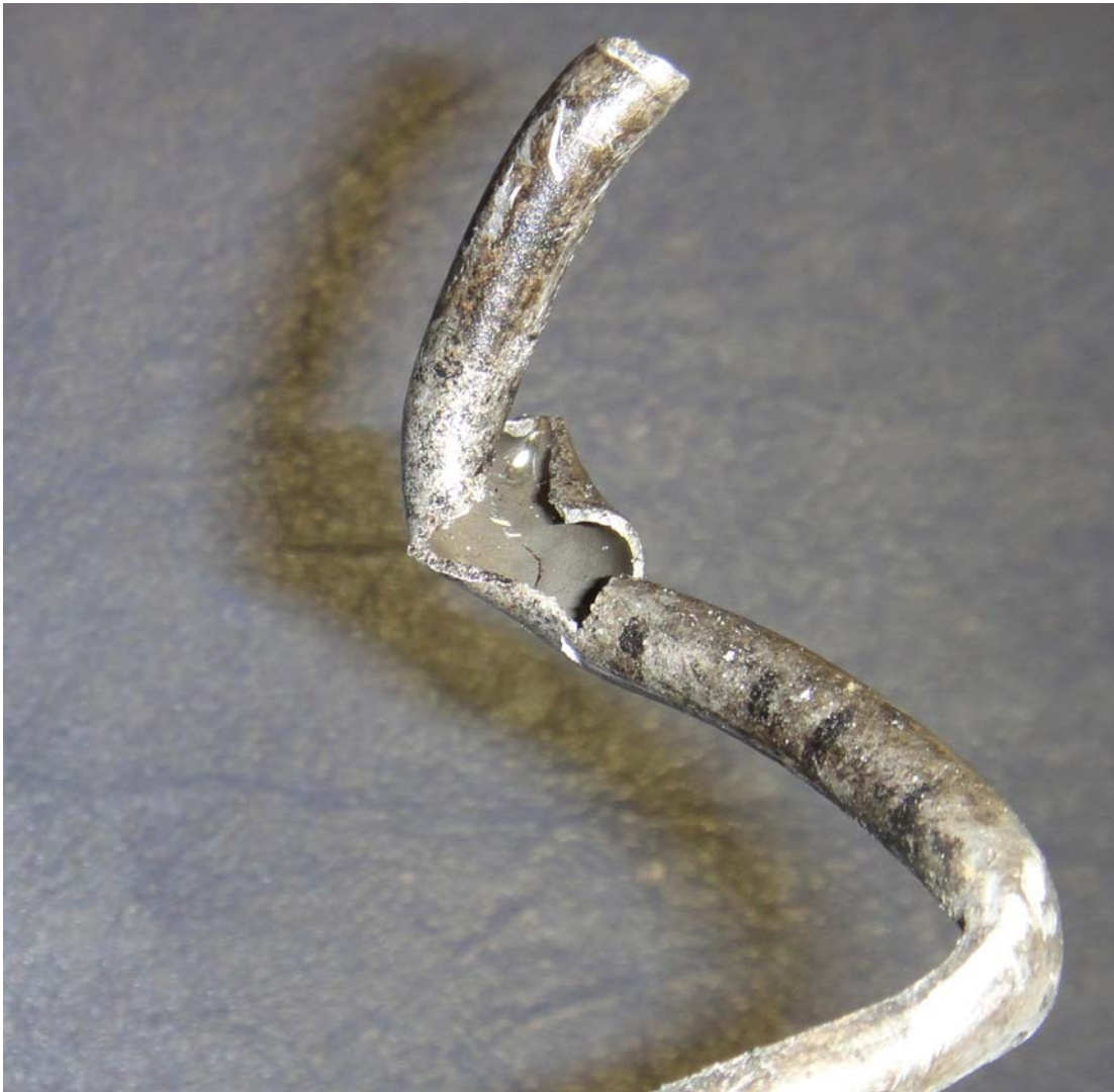
Figure 19. Closeup photograph of hole in cabin heater fuel supply line.
