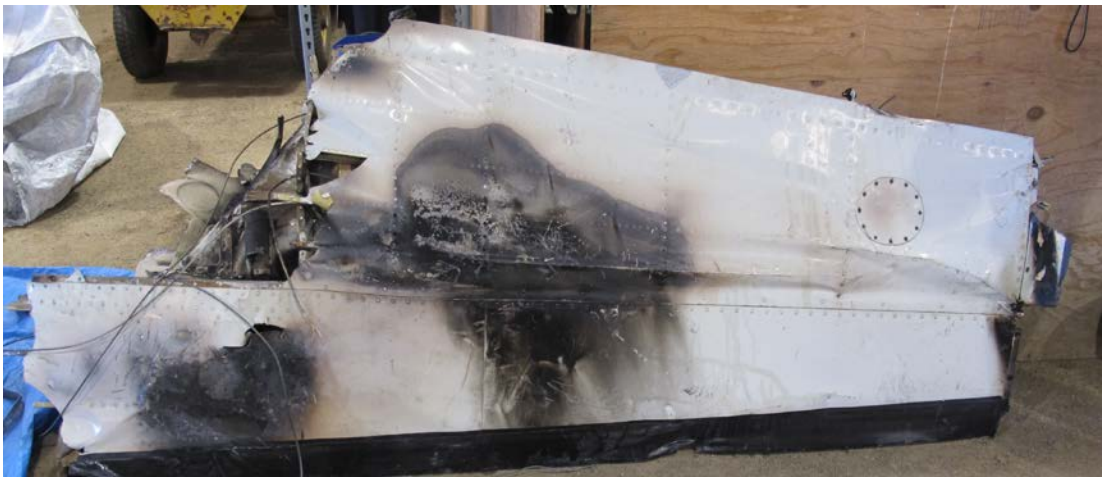
Figure 25. Photograph of thermal damage to left wing.
