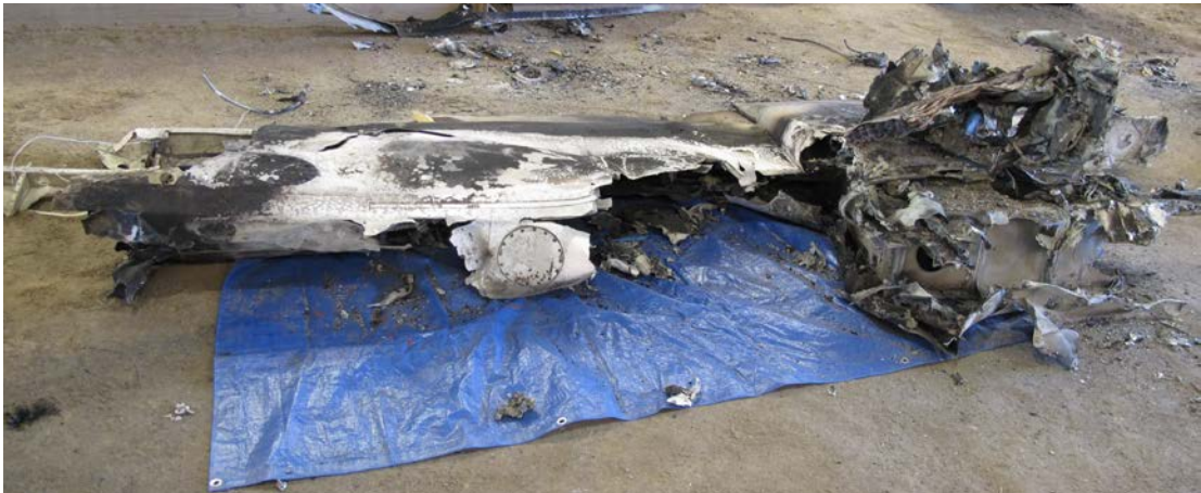
Figure 23. Photograph of remaining right wing structure.
