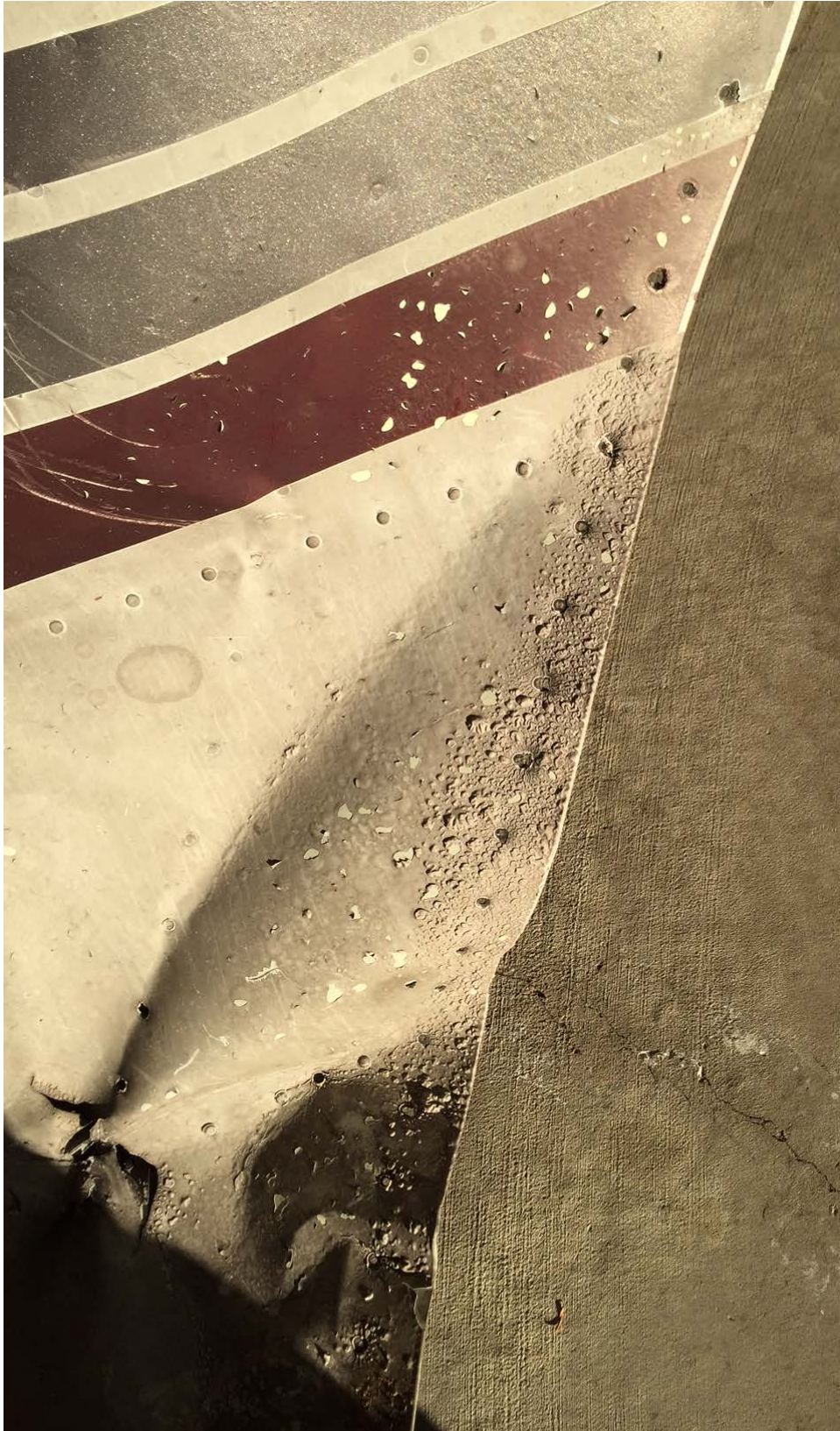
Figure 28. Closeup of thermal damage of left side section of vertical stabilizer.
