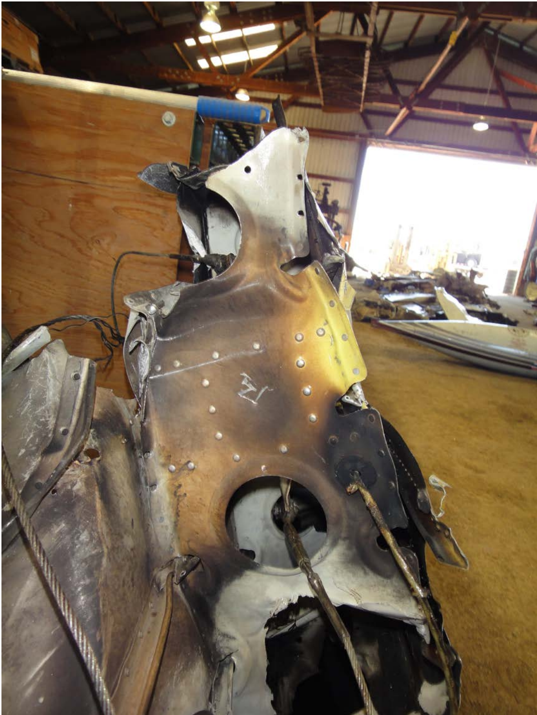
Figure 26. Photograph of thermal damage to interior of left wing fuel bay.
