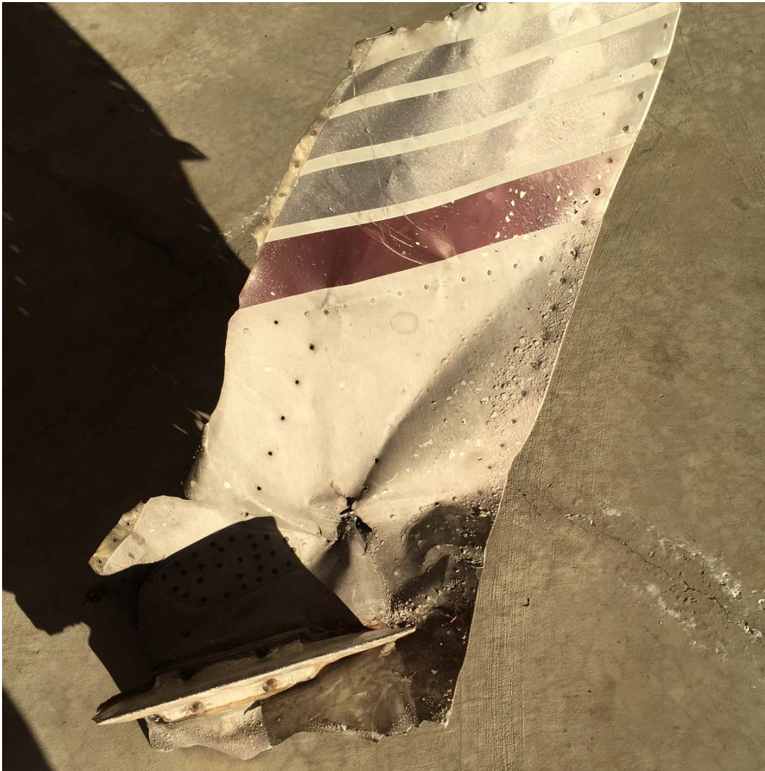
Figure 27. Overall photograph of recovered portion of the vertical stabilizer-left side.
