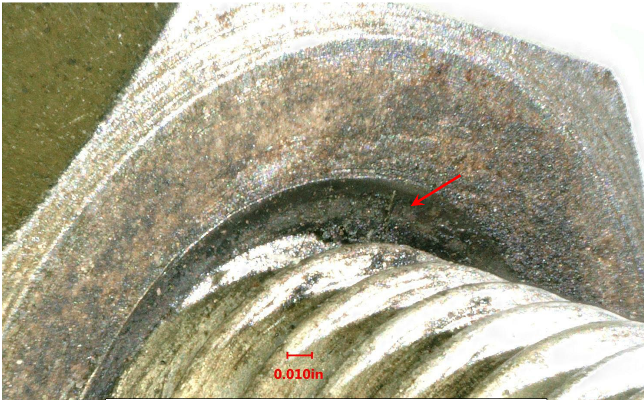
Figure 5. Two optical views showing the arc of wear, red arrow, on the rod side of the jam nut.
