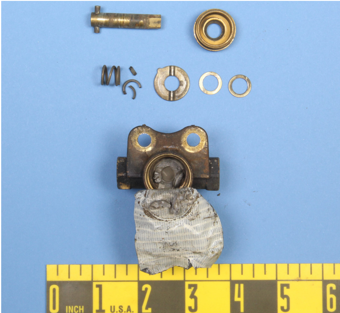
Figure 1. Overall photograph of fuel selector valve at intake.
