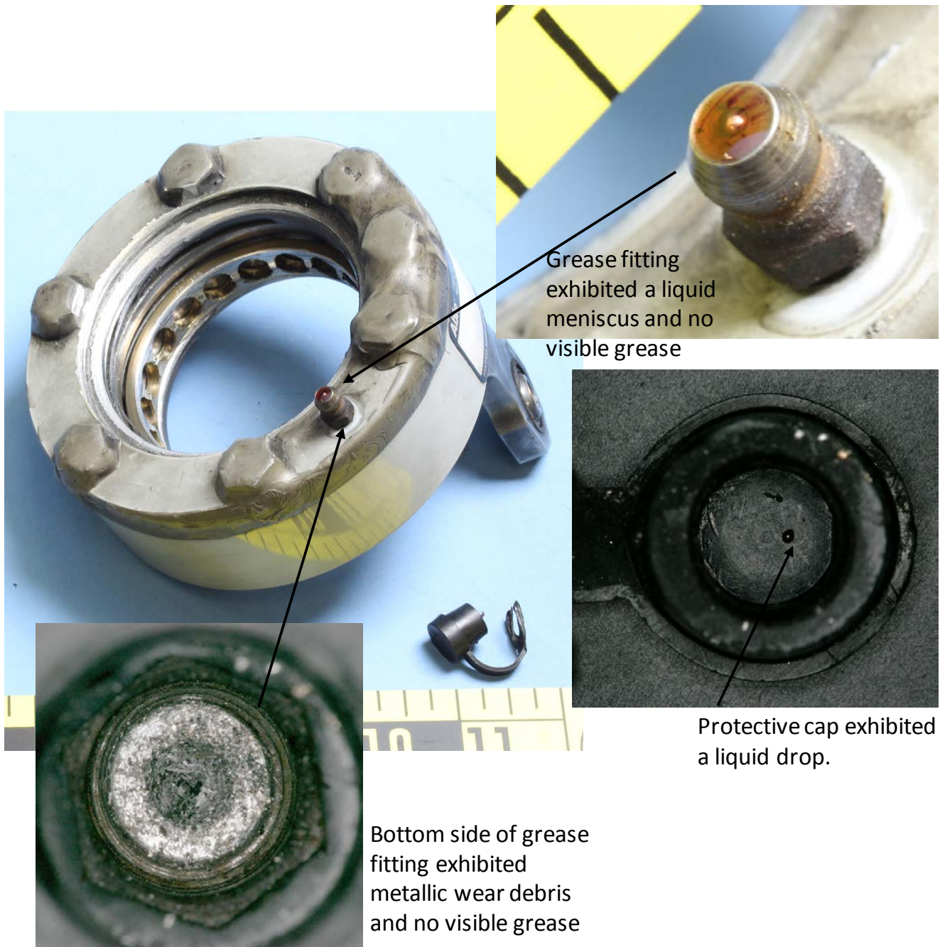
Figure 4 Portion of the stationary plate assembly depicting the presence of a liquid meniscus on the inlet portion of the grease fitting and metallic wear debris accumulated on the outlet portion of the grease fitting.
