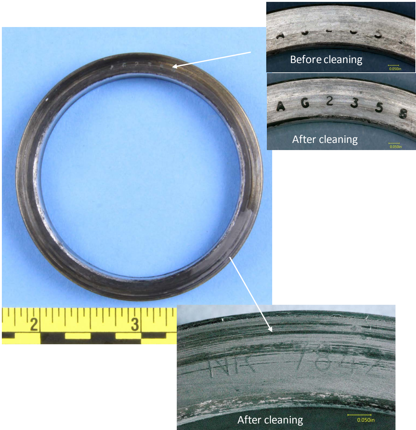
Figure 6 Images of the edge of the inner bearing half-race shown in Figure 5. The edge has been cleaned to reveal serial numbers.
