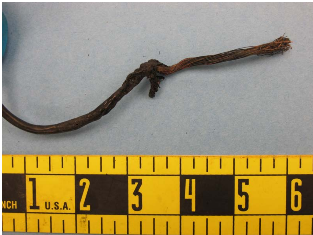
Figure 11. Close-up photograph of wiring damage.
