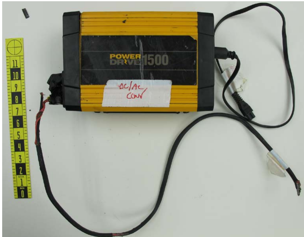
Figure 12. Photograph of the power inverter.
