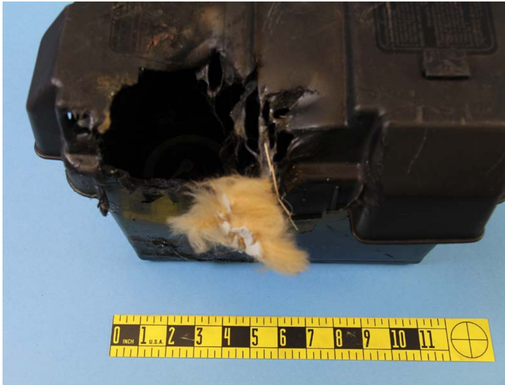
Figure 3. Close-up photograph of damaged battery box lid.
