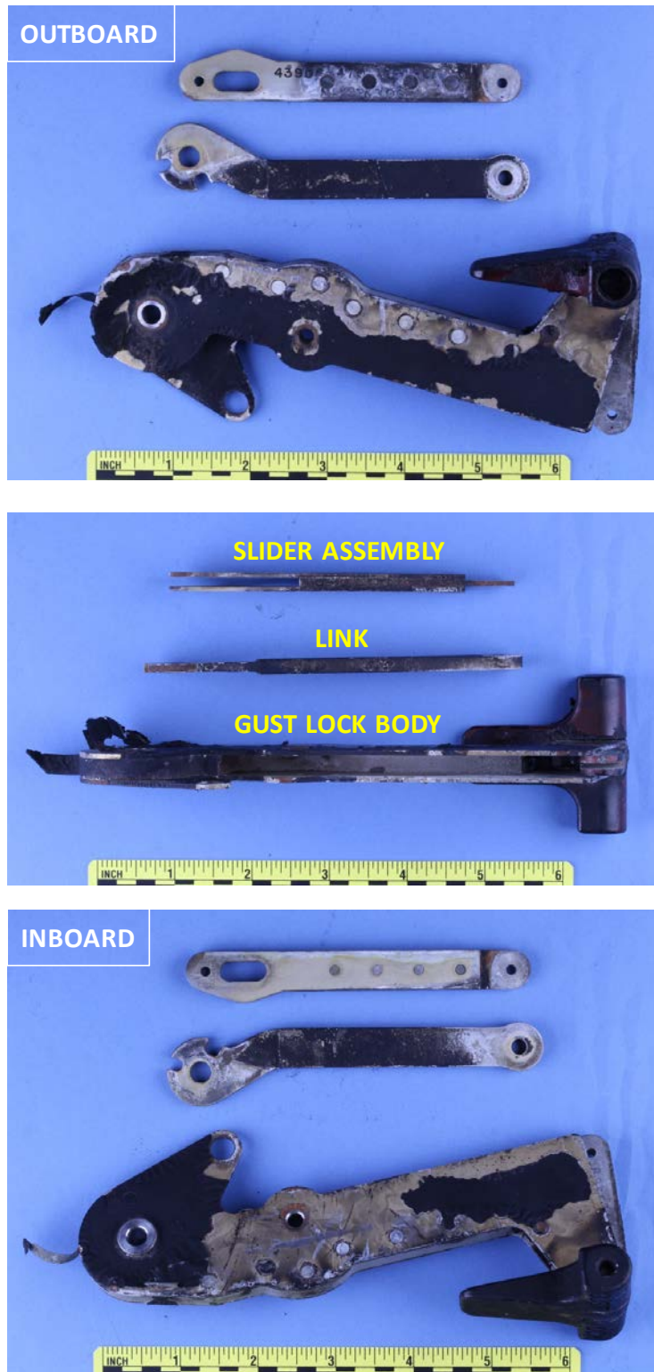
Figure 20: Overall photos of the disassembled gust lock body, link and slider assembly from the gust lock handle.
