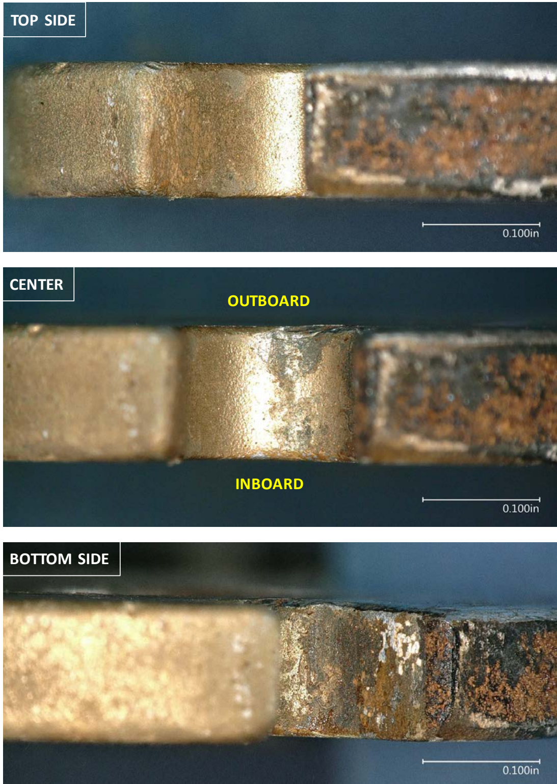
Figure 23: Digital microscope photos showing the down slot surface on the link from the gust lock handle.
