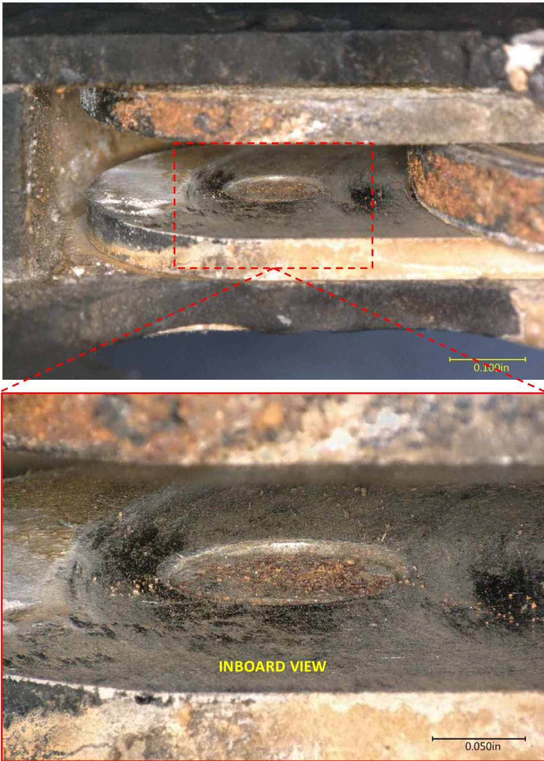
Figure 4: Digital microscope photos of the recessed lock pin piece on the inboard side of the gust lock handle.
