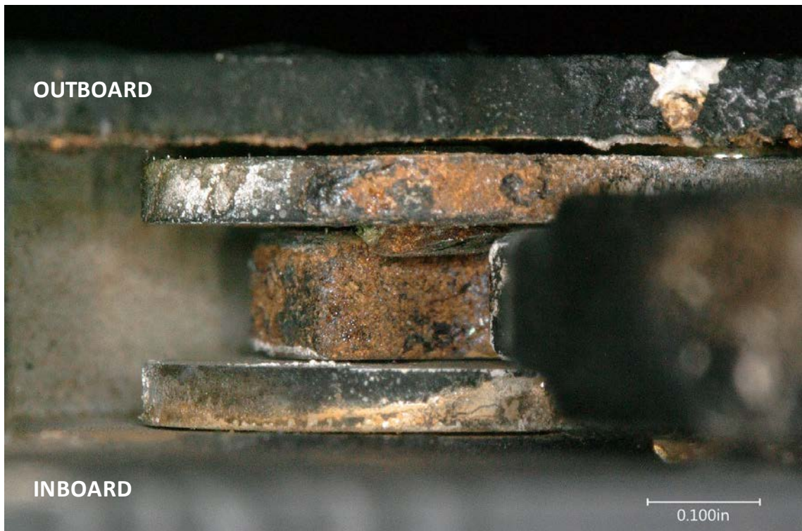
Figure 6: Digital microscope photos showing the protruding outboard lock pin piece contacted the outboard side of the link when the link was rotated within the gust lock handle.
