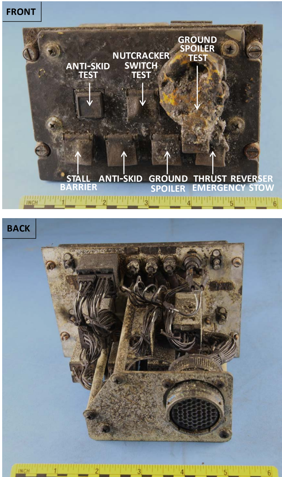
Figure 33: Overall photos of the pedestal switch panel.
