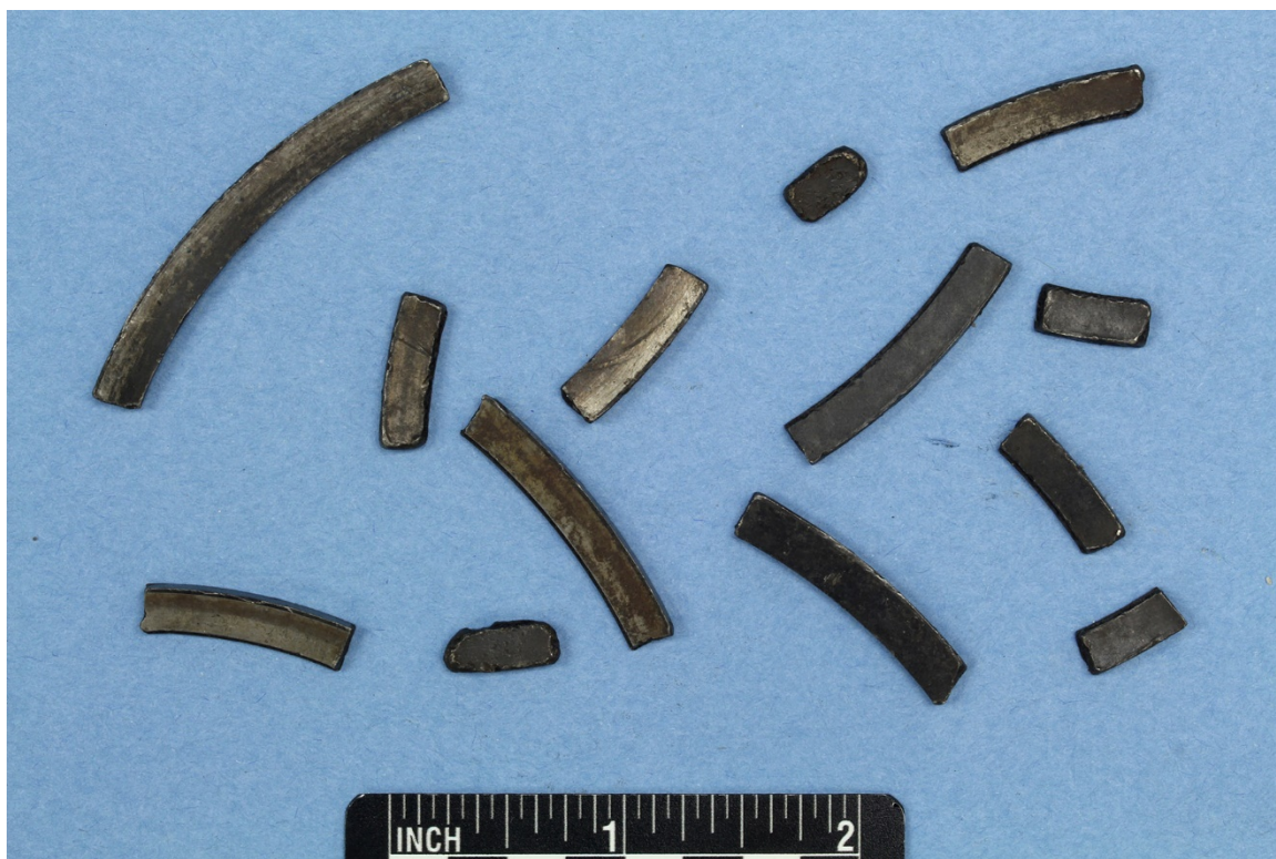
Figure 6 (cont.): c) Recovered pieces of the top compression ring. Approximately 70% of the ring was recovered.
