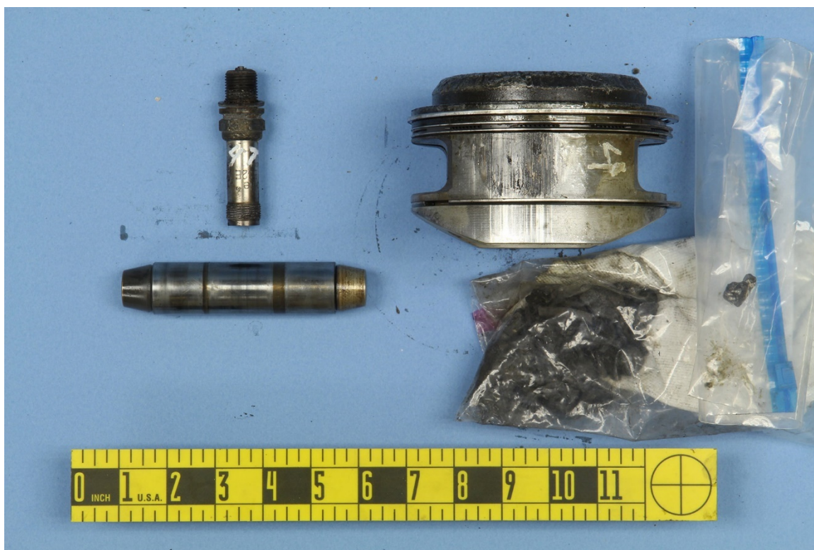
Figure 1 (cont.): c) image of the number 3 cylinder piston, piston pin, and upper spark plug; d) image of the number 4 cylinder piston, piston pin, upper spark plug, and bag containing piston, insert, and ring fragments;
