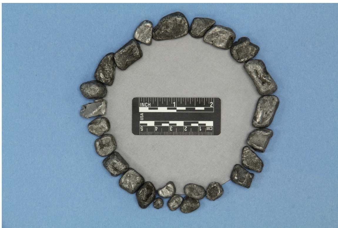
Figure 6: a) Pieces of the top ring insert. An estimated 80% to 90% of the insert was recovered; b) pieces of the piston from the top land/crown region. An estimated 80% to 90% of the top land/crown material was recovered.
