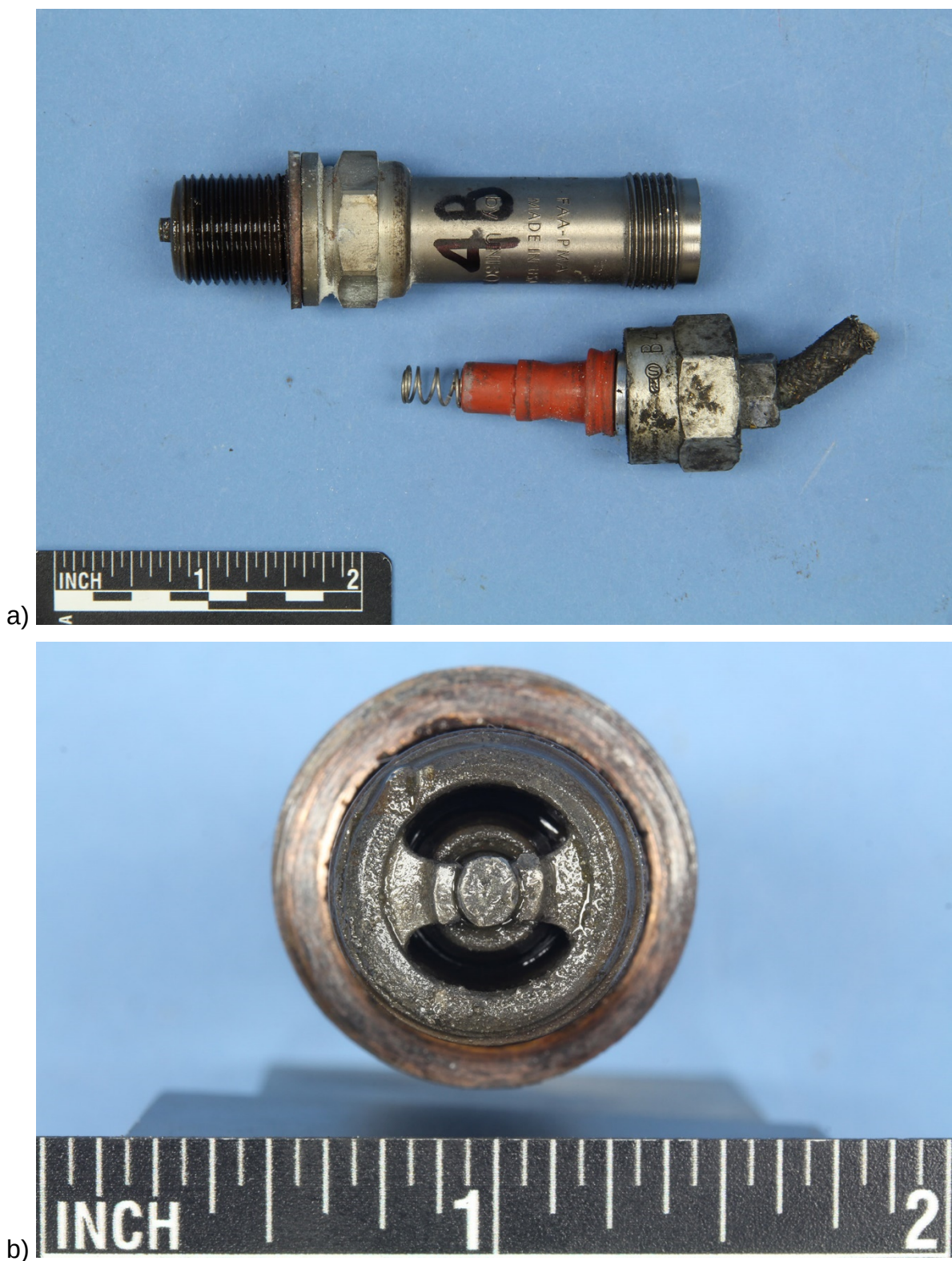
Figure 25: Images of the number 4 cylinder bottom spark plug: a) overview image of the plug and the terminal connector and b) image of the spark plug tip.
