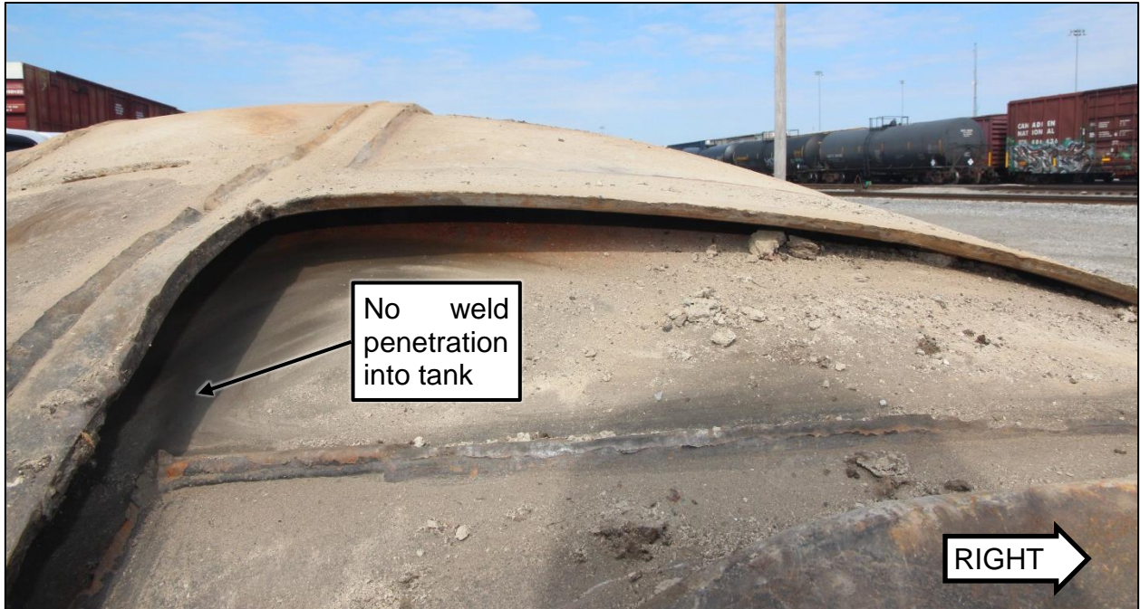
Figure 4. Views of deformation at the right side of the sill pad where it intersected the body bolster pad. No weld penetration into the tank was observed where the body bolster pad was welded to the sill pad, consistent with the zero root opening bevel weld specified at the inboard end of the body bolster pad.
