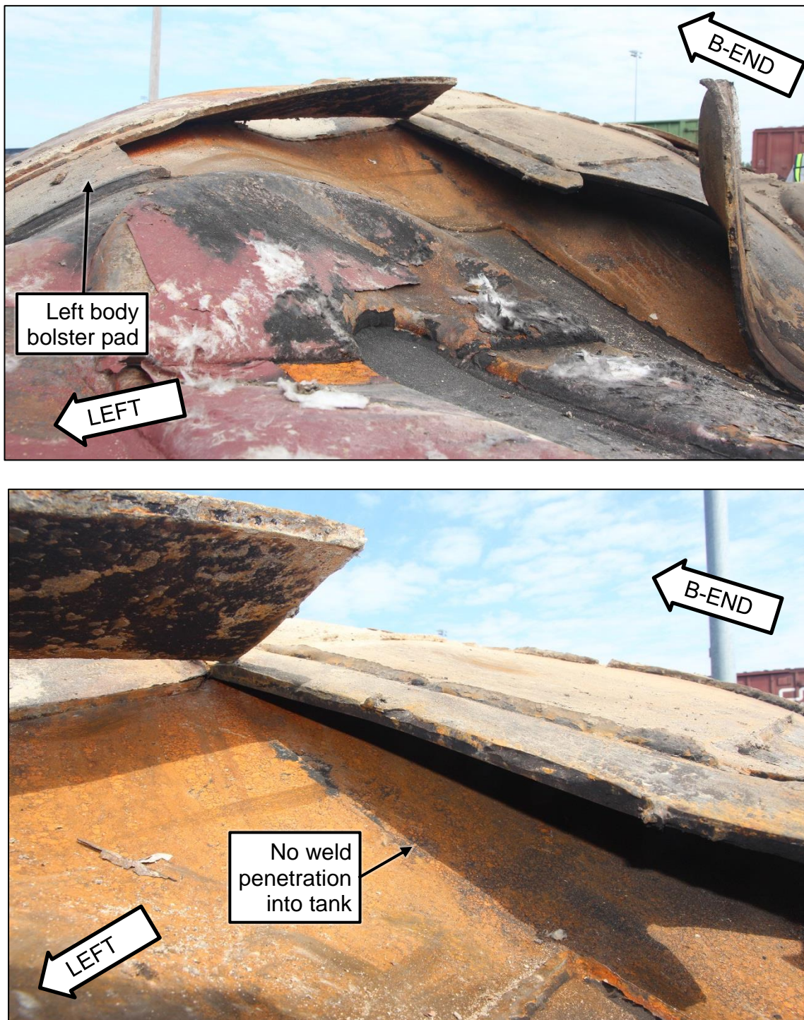
Figure 3. Views of deformation at the left side of the sill pad where it intersected the body bolster pad. No weld penetration into the tank was observed where the body bolster pad was welded to the sill pad, consistent with the zero root opening bevel weld specified at the inboard end of the body bolster pad.
