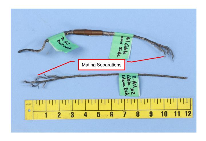
Figure 1. An overall view of the as-received aileron cable pieces with mating wire rope separations denoted.
