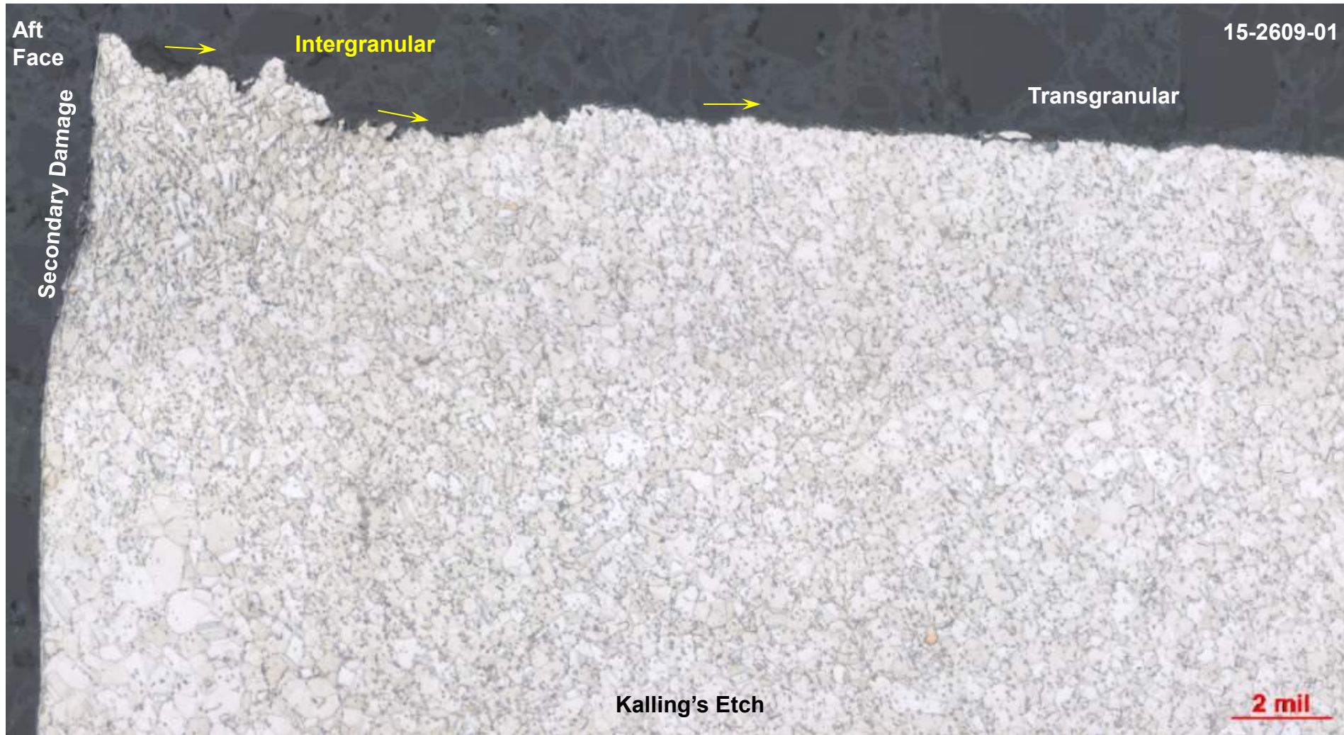
Figure 52: View of the 2 nd step polish into the inboard side of the fracture after etching with Kalling's etch showing a microstructure consistent with properly processed material with no anomalies noted. The corner in the impacted areas was slightly worked, consistent with secondary damage.
