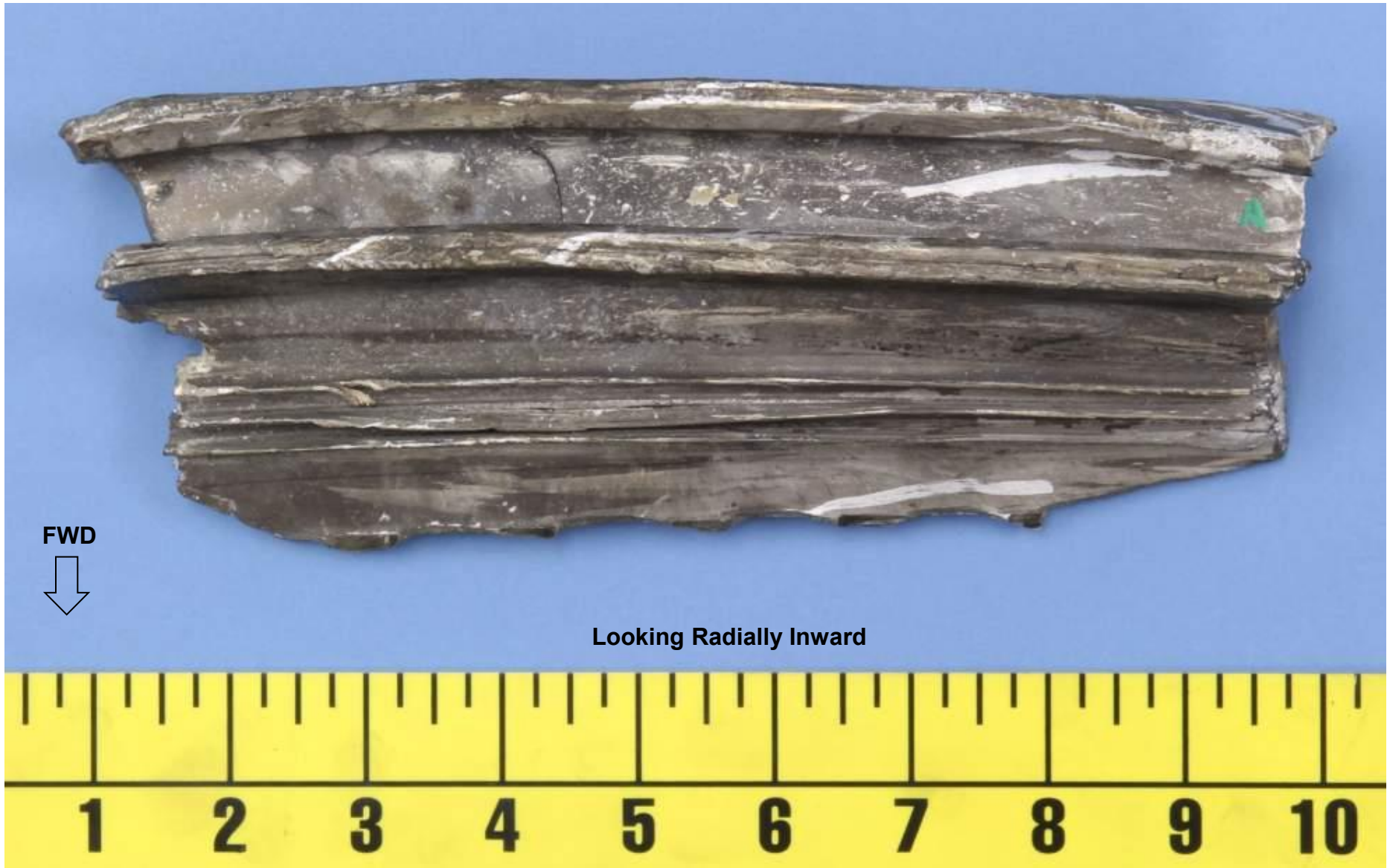
Figure 5: Optical view of the portion of the liberated stage 8 rim piece containing the fatigue fracture in the web (not visible).
