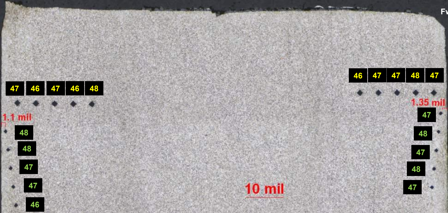
Figure 55: Micro-hardness measurements taken near the forward and aft faces ranged between HRC 46-48 and conformed to the requirement of C50TF81.
