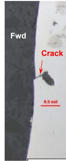
Figure 103: A mount made through one of the cracked areas near the rim fracture end showed that the minimum web wall thickness was reduced to 0.114 inch and multiple polishes could not clearly resolve the small surface cracks on the aft face (lower images), but on the forward face 0.5 mil deep cracks were found that extended at an angle, consistent with event-induced shear cracks.
