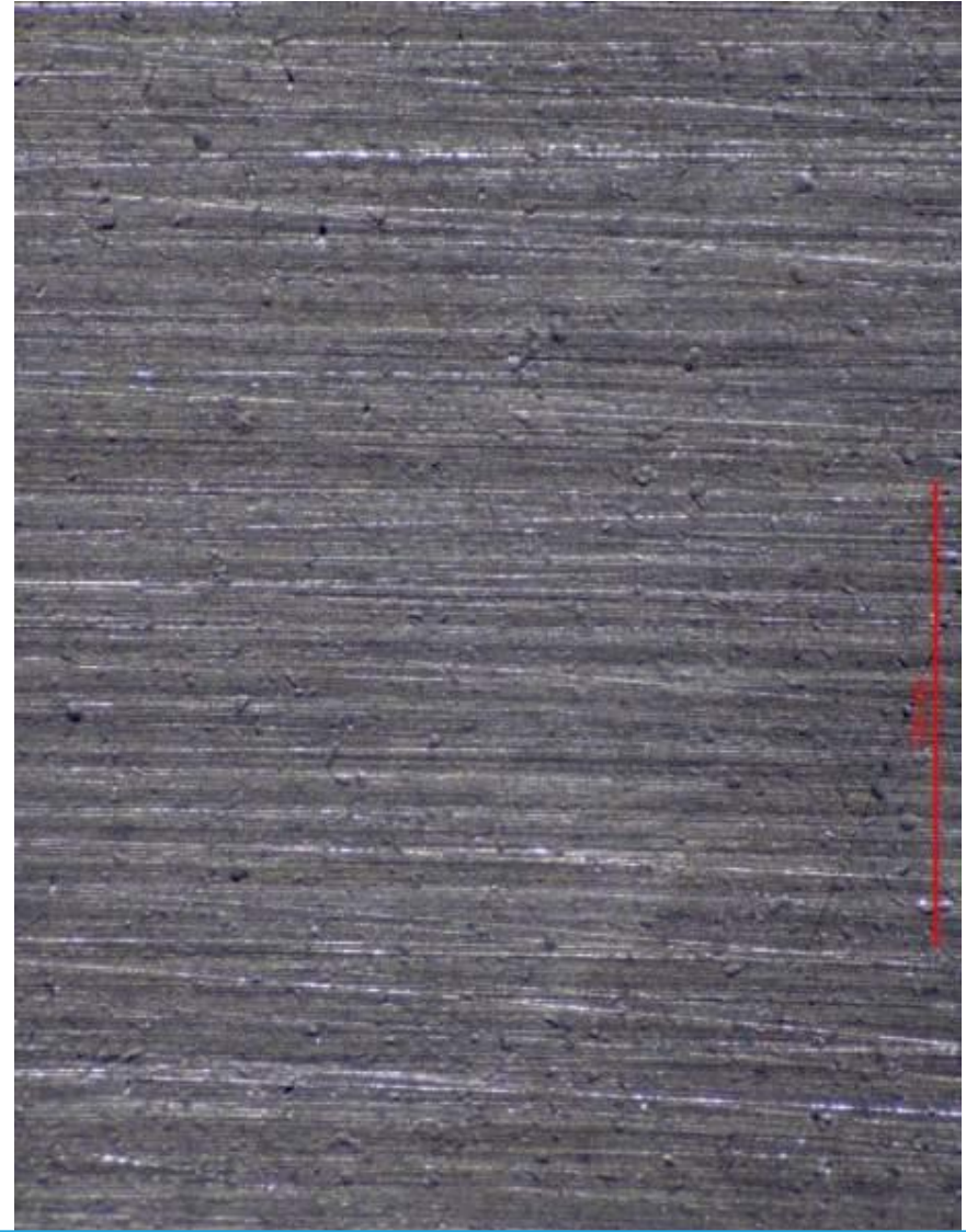
Appendix B1: Representative views of the stage 8 disk forward and aft web faces from spool S/N GWNHA139 showing visual differences in the peening with the forward side being more pronounced, like the event disk.
