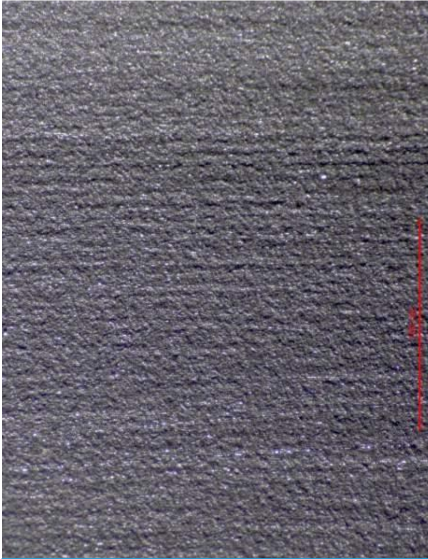
Appendix B1: Representative views of the stage 8 disk forward and aft web faces from spool S/N GWNHA139 showing visual differences in the peening with the forward side being more pronounced, like the event disk.
