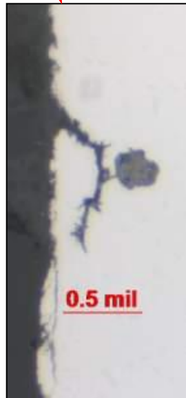
Figure 44: As-polished 5 th step view of the inboard fracture through the approximate origin area showing initial intergranular growth that transitioned to transgranular growth with no material anomalies noted. The first 1 mil of the aft face was damaged by post-fracture smearing. In the current plane of polish the predominantly intergranular region was up to 16 mils deep.
