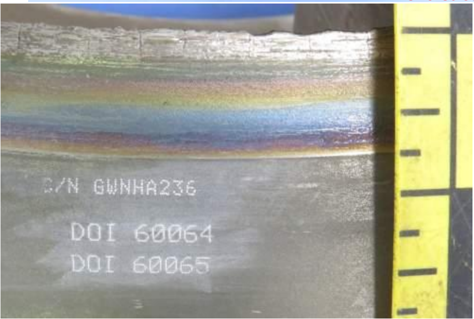
Appendix A1: Optical views of the aft end of the 8-10 spool showing the part markings and fracture locations. There was a fracture forward of the stage 9 disk, consistent with the liberation event, and the aft cone arm was fractured consistent with rubbing against the static structure/CDP seal.
