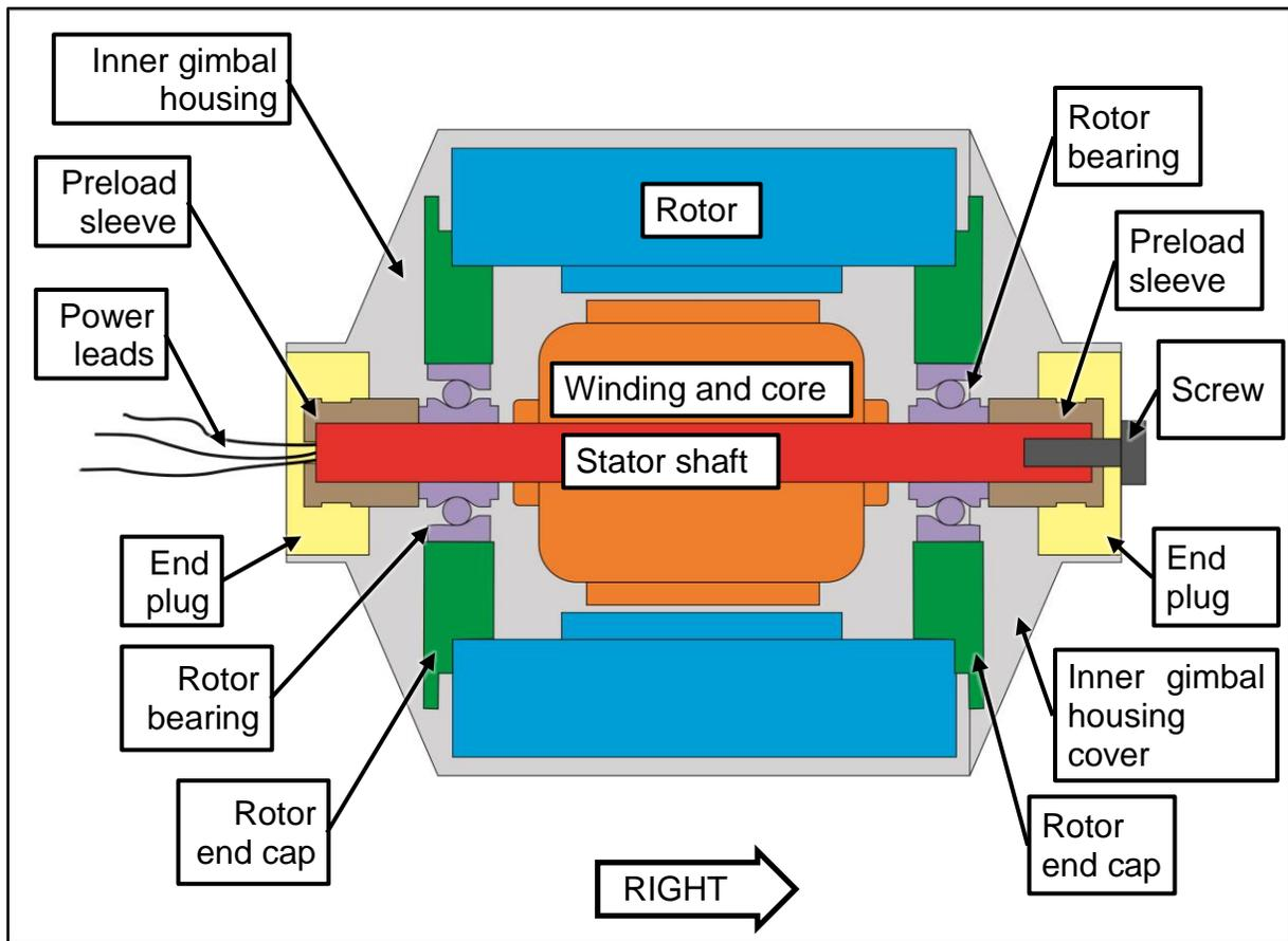
Figure 2. Illustration of a cross-section through the inner gimbal assembly from the vertical gyro showing components of the assembly.
