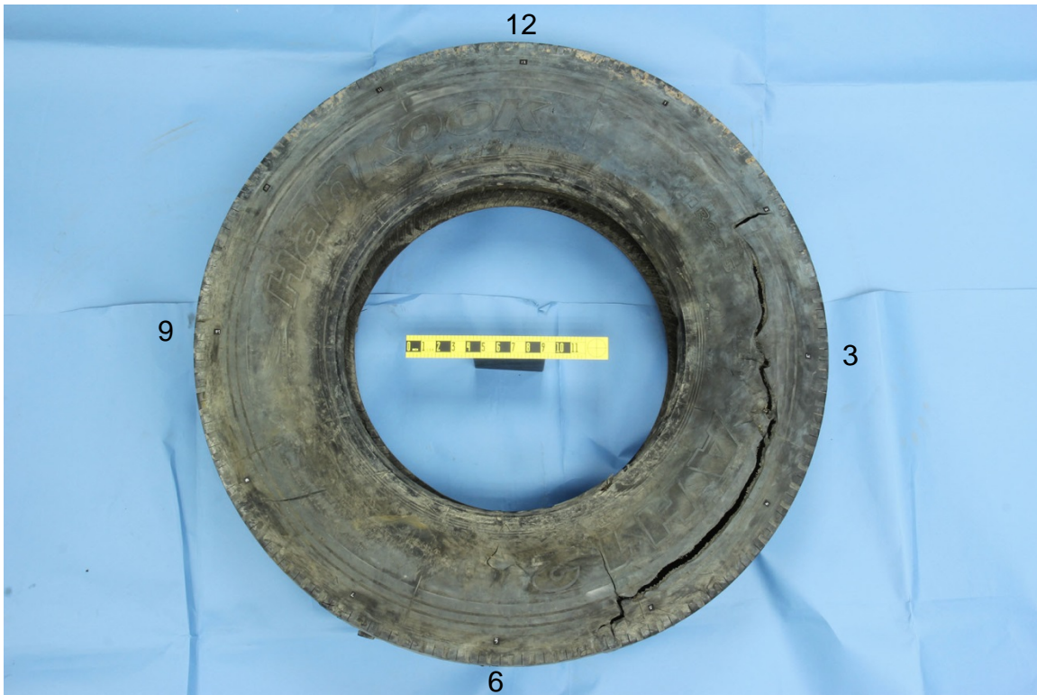
Figure 1: The outboard sidewall of the left front tire. The indicated clock positions are referenced off of the "O" in "DOT", part of the tire identification number.
