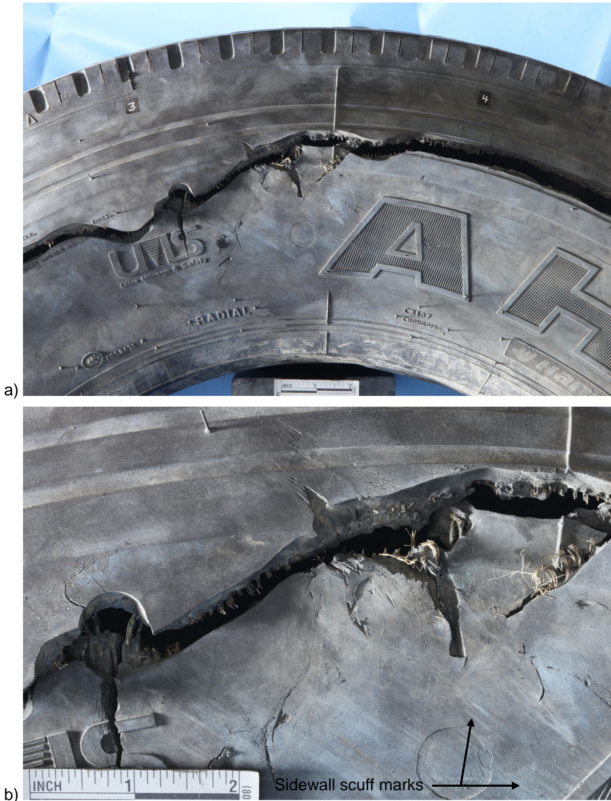
Figure 2: a) The outboard sidewall of the left front tire between 3:00 and 4:00 and b) higher magnification image of two notable features at approximately the 3:15 position: a round hole, approximately 5/8 inch in diameter and a triangular gouge, approximately 1 inch across.
