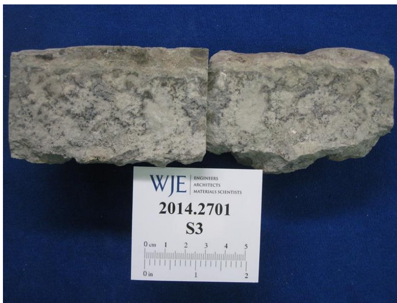
Figure A8. Core S3, fracture surface of the upper segment. Fracture does not appear to be recent.
