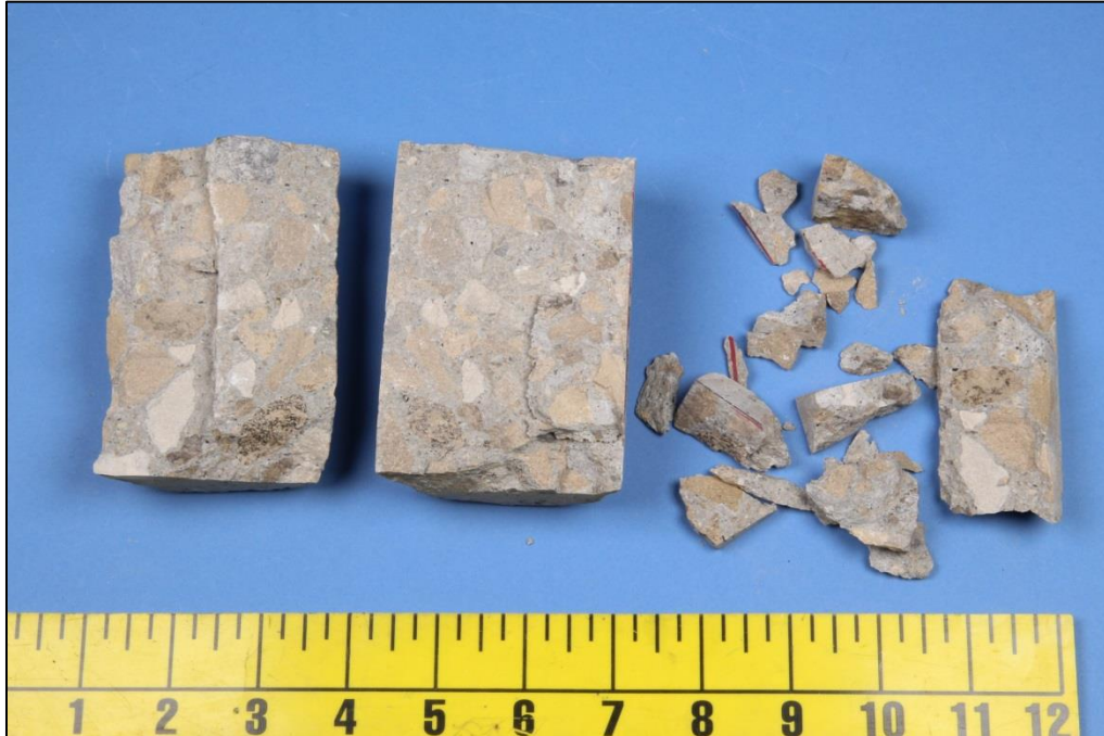
Figure 7. View of splitting tension test specimen from tie S3 shown after testing.
