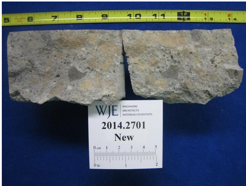
Figure A4. Core NEW, opened fracture surface of the upper segment. The fracture appears to be fresh.
