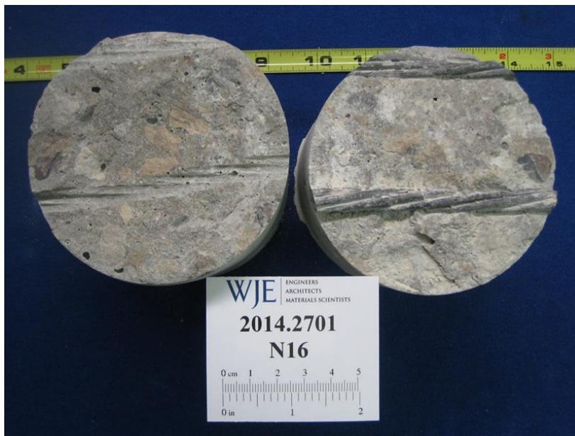
Figure A24. Core N16, fracture surface at reinforcement.
