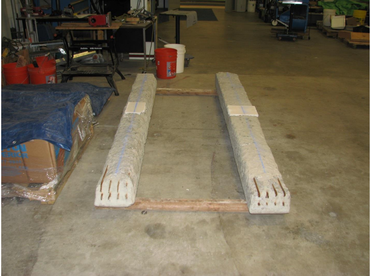
Figure 11. Hydrostone capping used at the loading area on used railroad ties N10 (left) and S5 (right).
