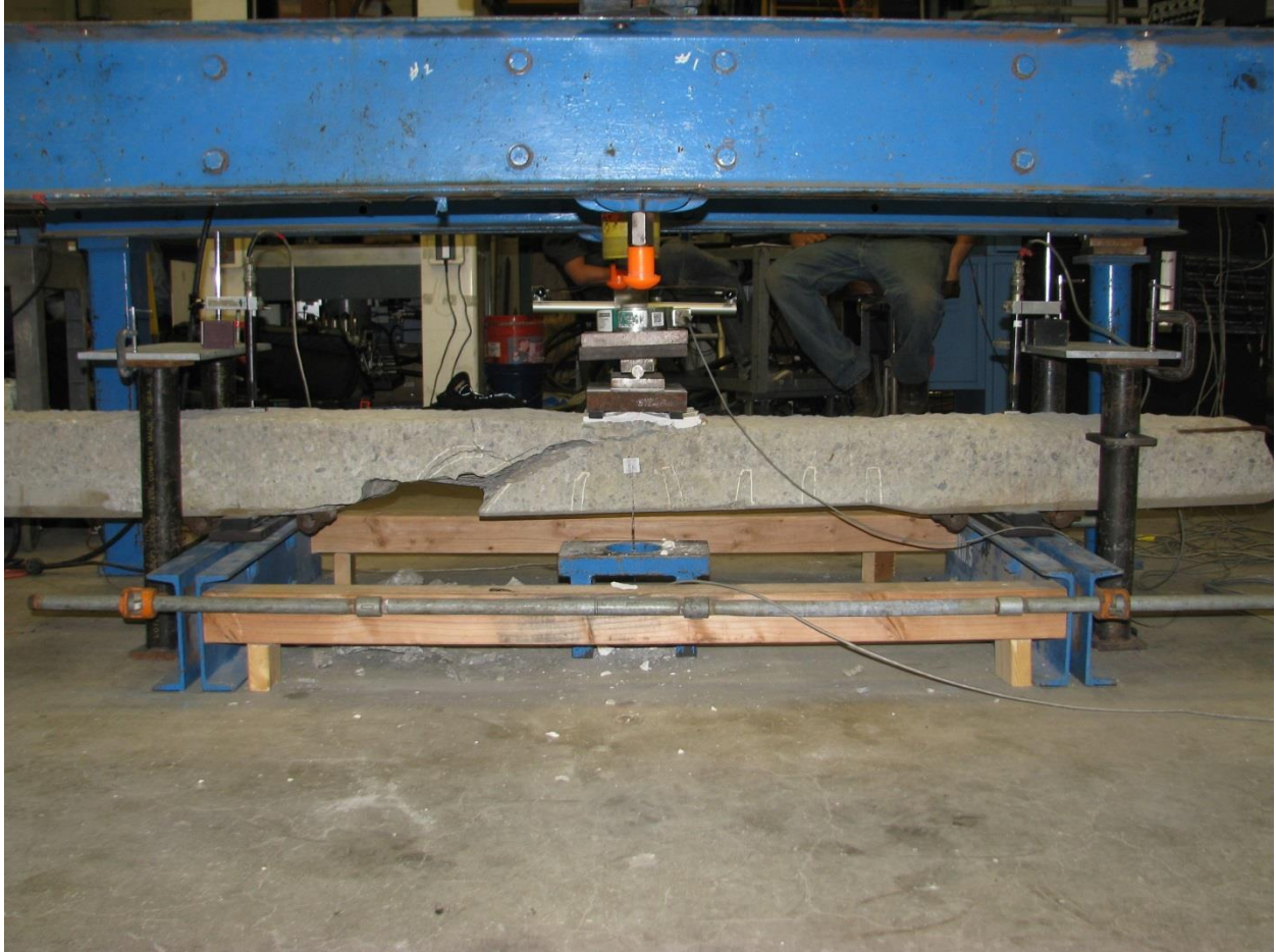
Figure 22. View of east face of tie S5 after failure.
