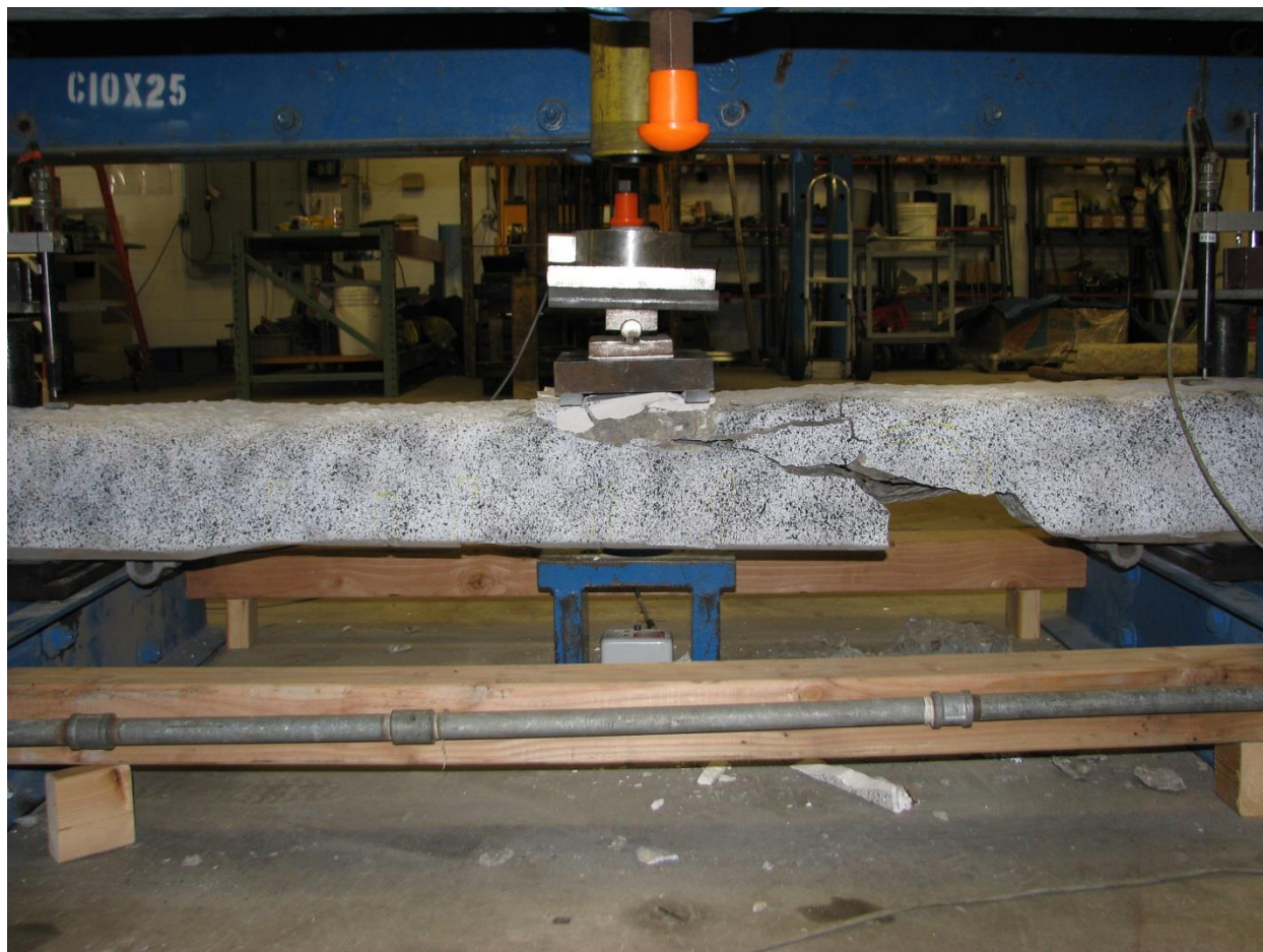
Figure 23. View of west face of tie S5 after failure.
