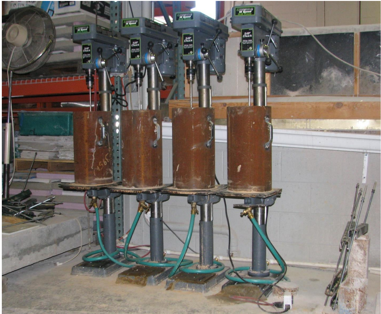
Figure 52. Abrasion test set-up.
