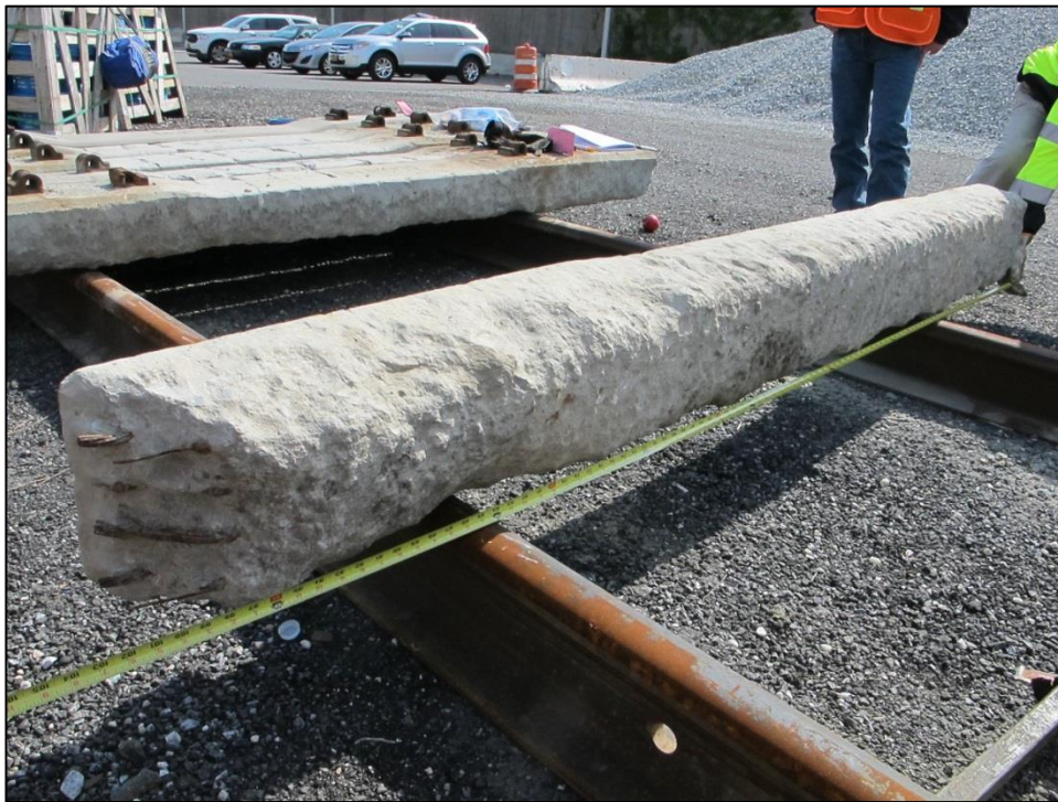
Figure 4. View of the lower surface of tie N16 showing typical features observed on the lower side of the ties.
