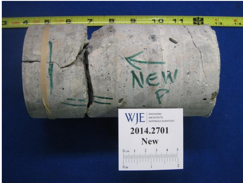
Figure A3. Core NEW, side view. Top surface (cast bottom) is on left.
