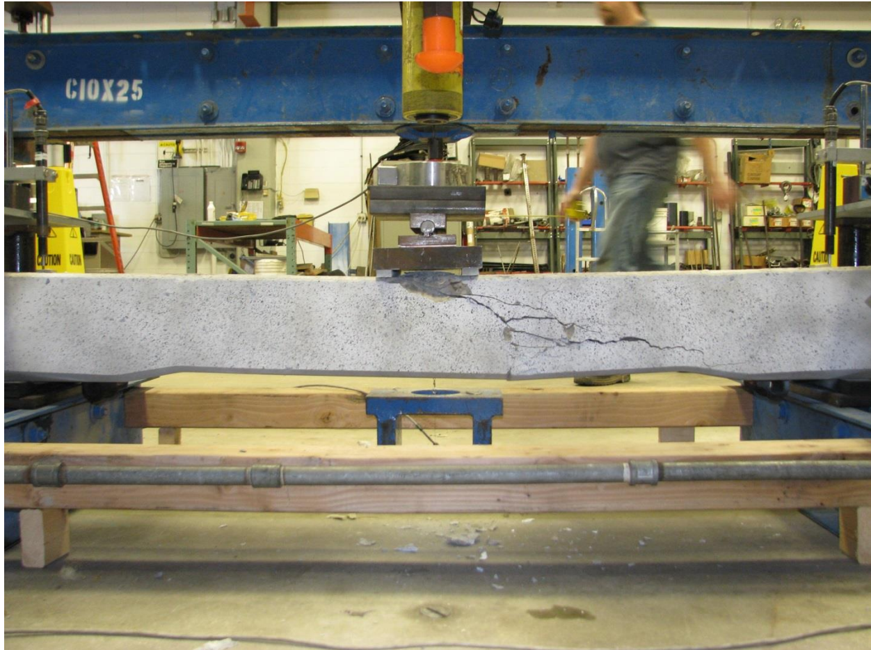
Figure 19. View of west face of New Tie after failure.
