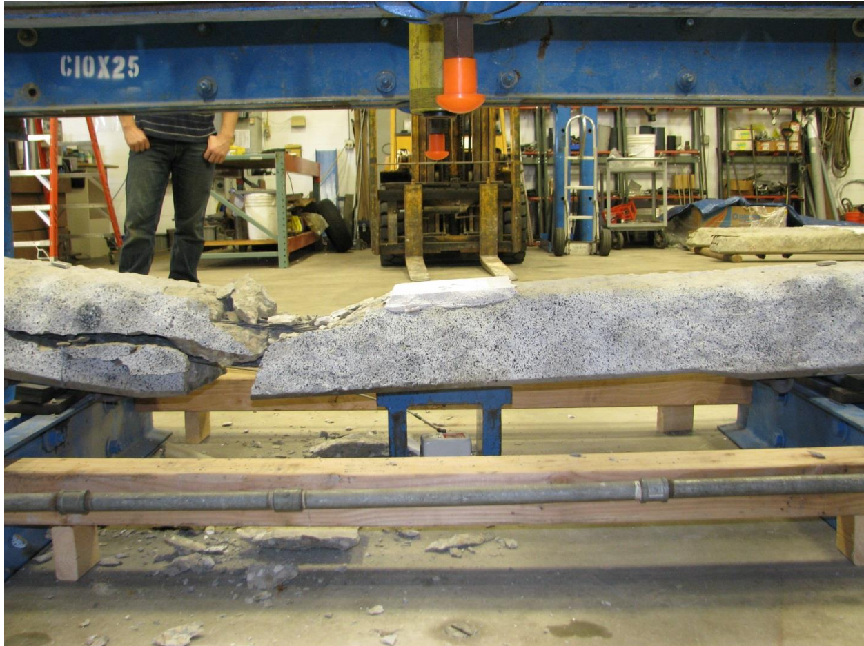
Figure 21. View of west face of tie N16 after failure.
