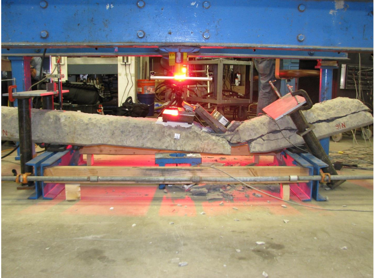
Figure 20. View of east face of tie N16 after failure.
