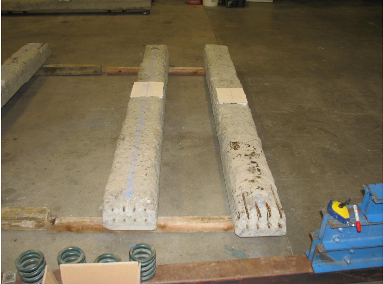
Figure 10. Hydrostone capping used at the loading area on used railroad ties N16 (left) and S4 (right).
