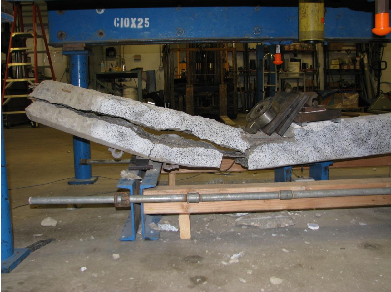
Figure 27. View of west face of tie N10 after failure.
