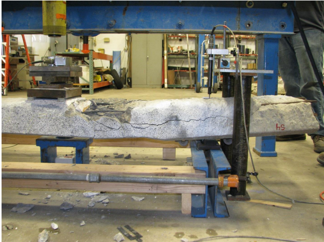
Figure 25. View of west face of tie S4 after failure.
