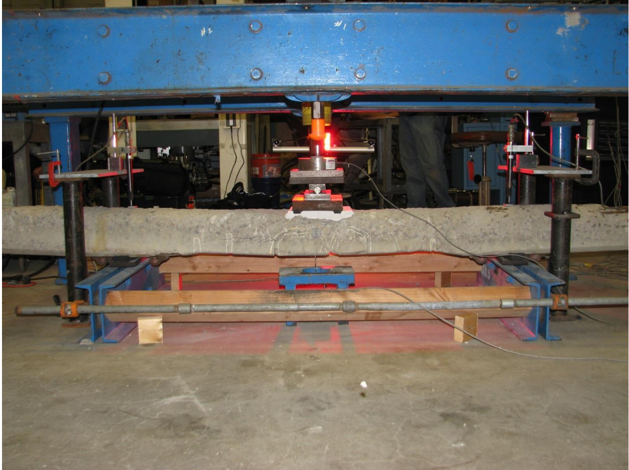
Figure 28. View of east face of tie S3 after failure.
