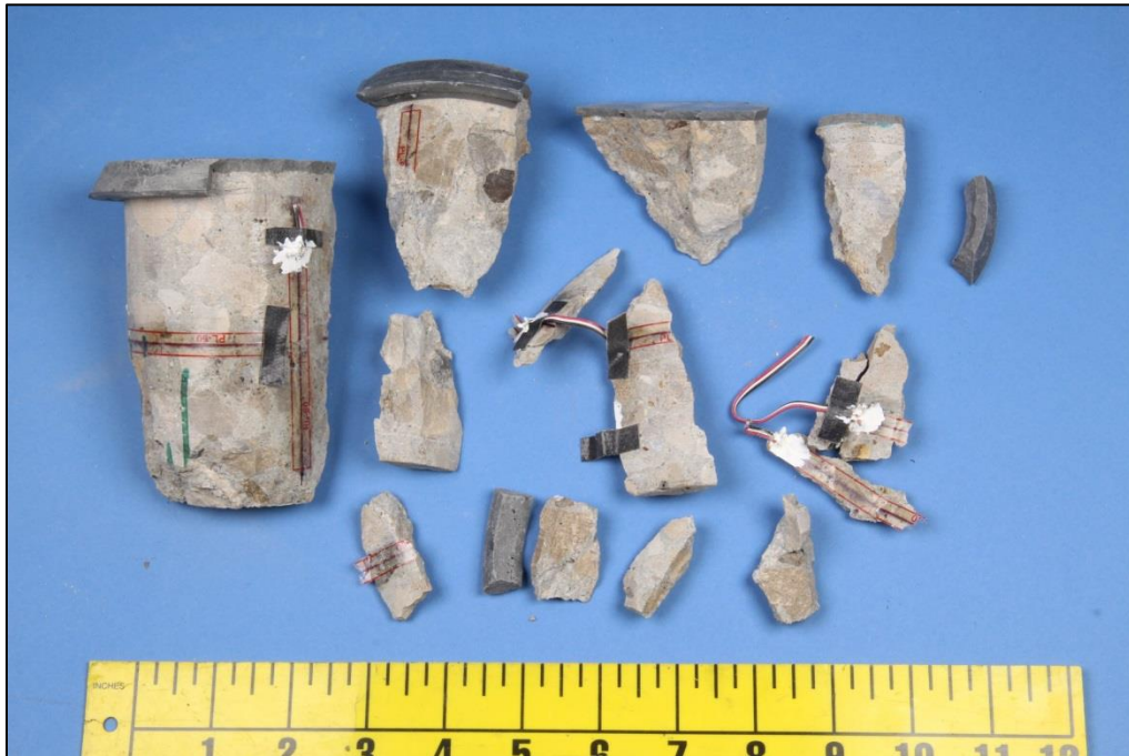
Figure 6. View of the compression test specimen from tie S3 shown after testing.
