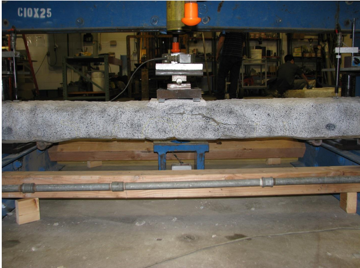
Figure 29. View of west face of tie S3 after failure.
