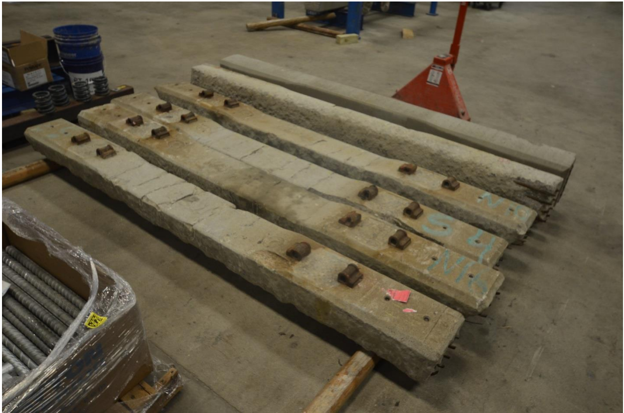
Figure 1. Overall view showing in service top face of as received railroad ties S3, N16, S4 and N10, from left to right. Tie S5 and new tie are seated on their side.
