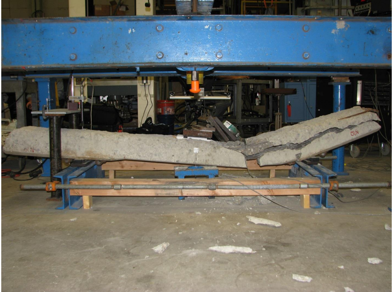
Figure 26. View of east face of tie N10 after failure.
