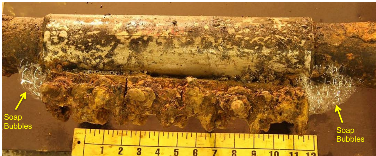
Figure 10. Photograph showing pipe segment "E" in area of the sleeve "S2" during pressure testing showing soap bubbles emitting from the ends of the sleeve. The soap bubbles show evidence of a leak.
