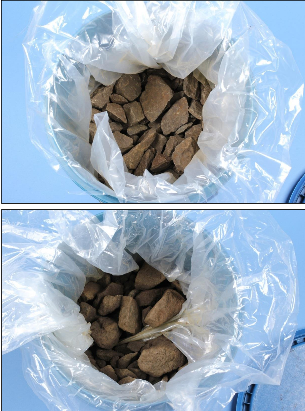
Figure 3. Overall views of the contents of the buckets labeled “clean ballast sample” (upper image) and “subgrade sample” (lower image).
