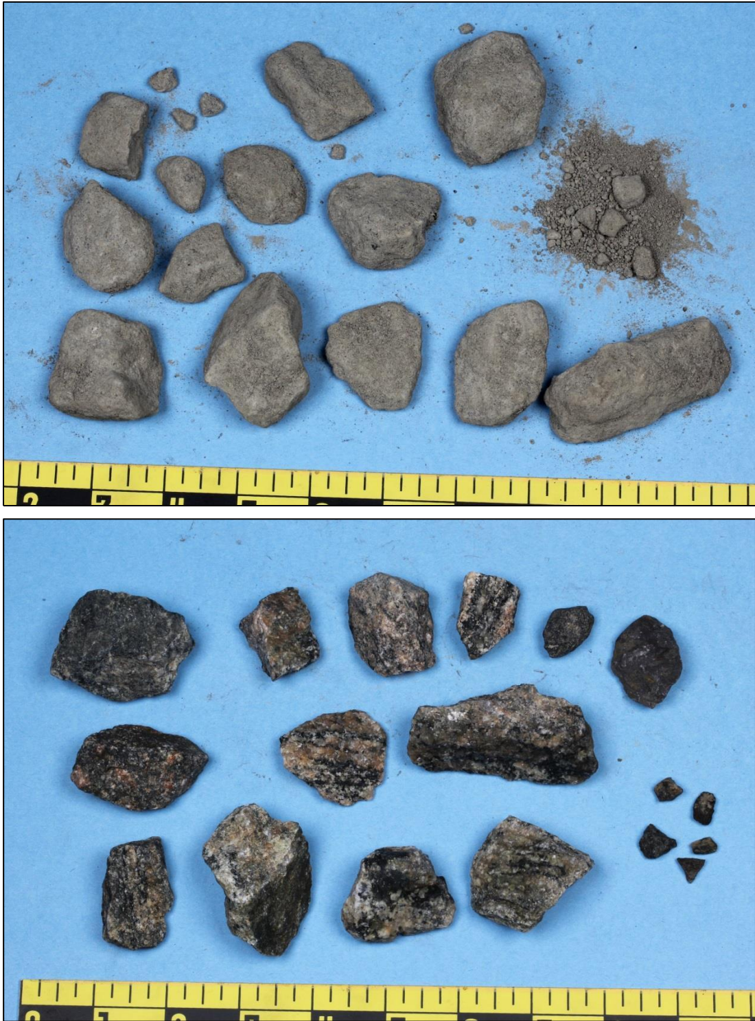
Figure 4. View of rocks from the fouled ballast sample after being dried (upper image) and after cleaning and drying (lower image).
