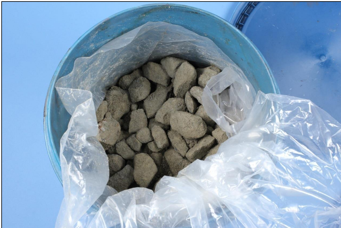
Figure 2. Overall view of the contents of the bucket labeled “fouled ballast sample”.
