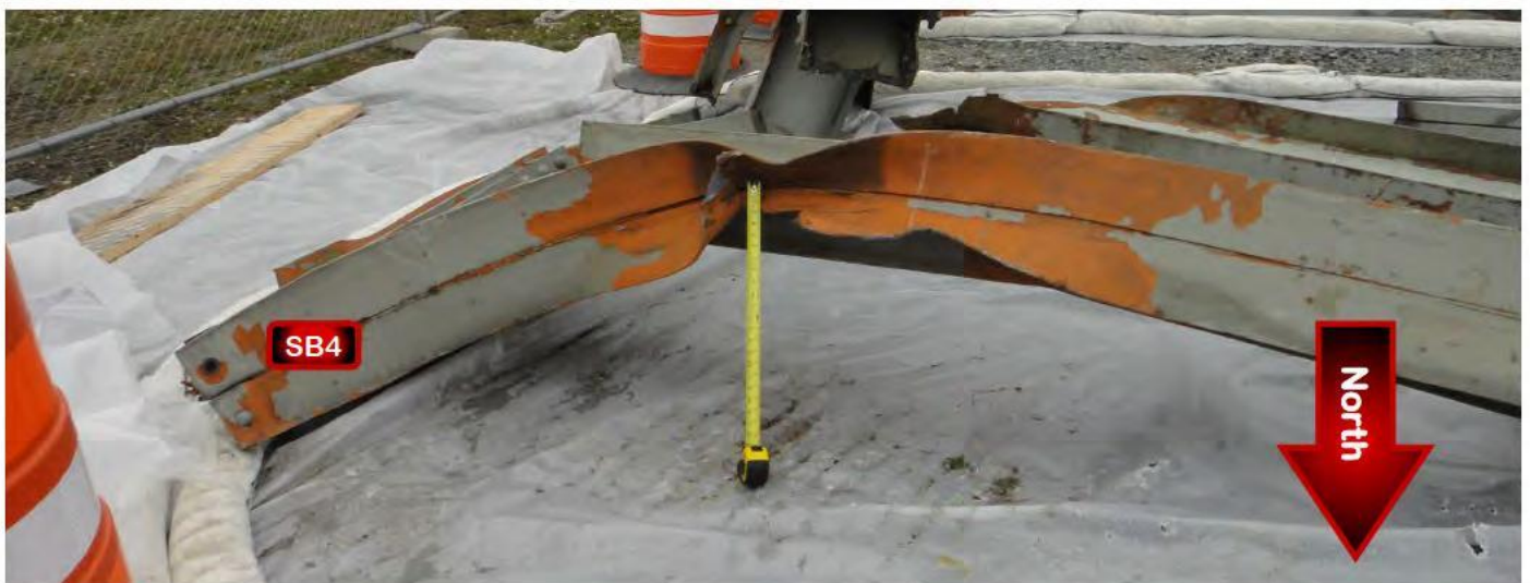
Figure 16. Impact damage to sway brace 4 above with extent of bowing depicted below.
