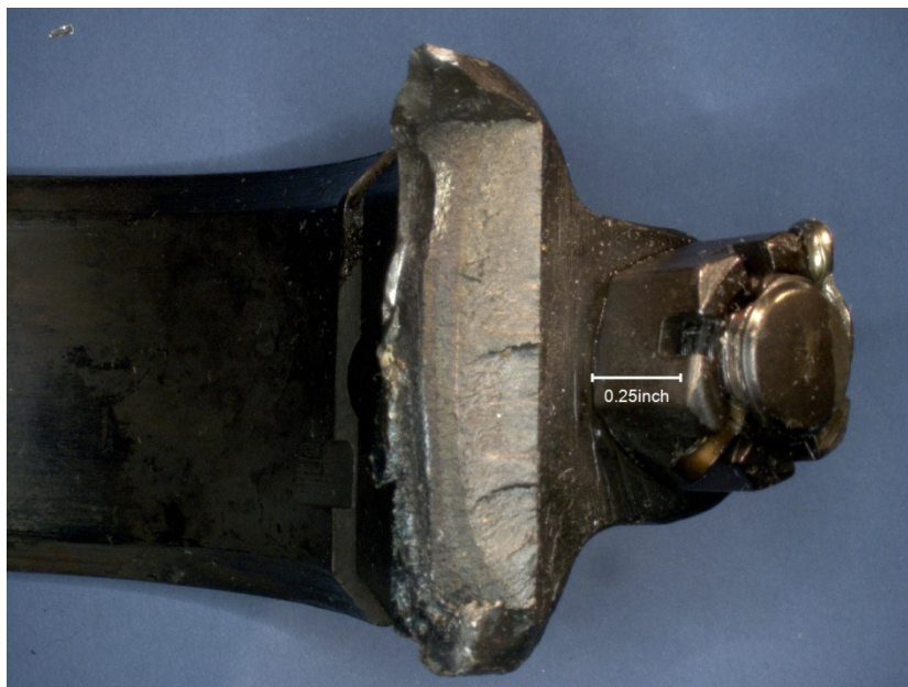
Figure 5: Mating fracture surface to the one shown in figure 3.
