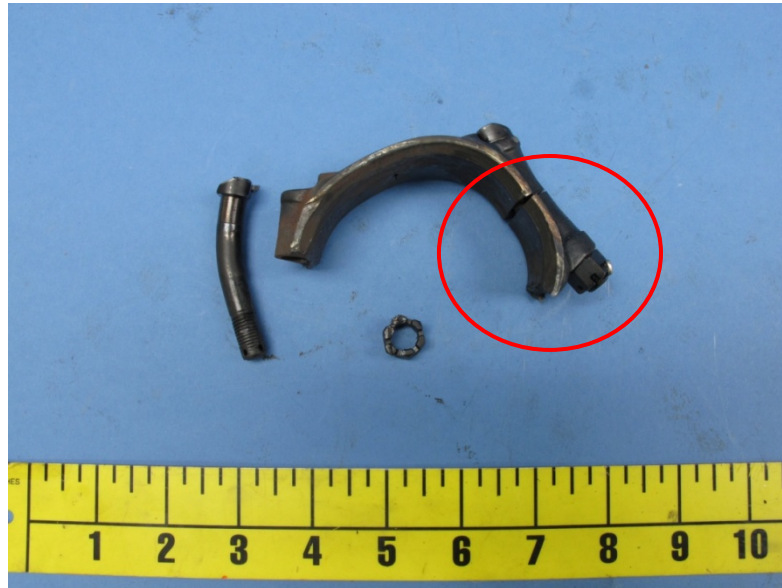
Figure 4: #2 piston rod bearing cap with portion of connecting rod attached (circled in the photo)
