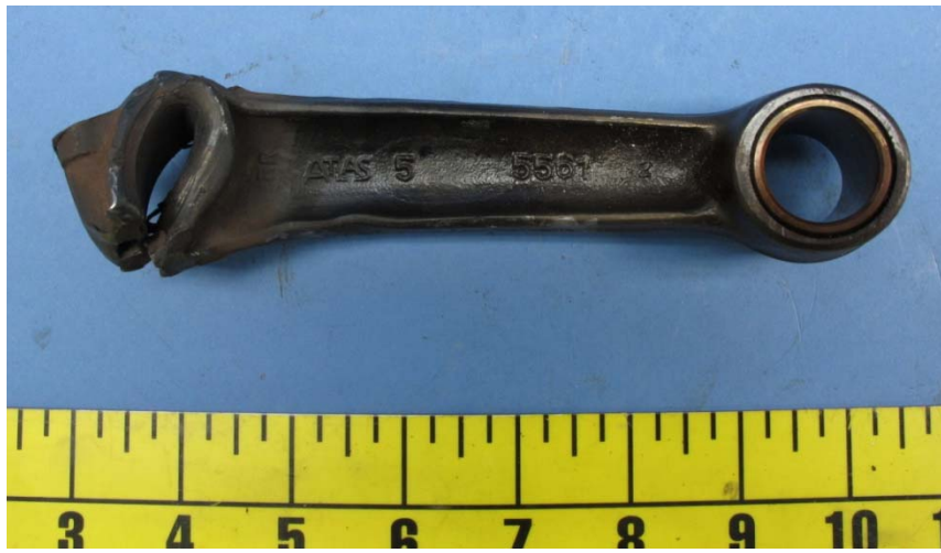
Figure 2: Damaged connecting rod assembly from the #2 cylinder
