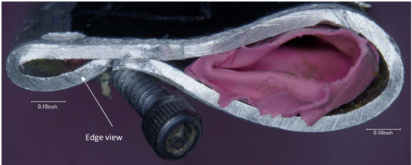
Figure 7 Edge view of the top of the forward control stick piece.
