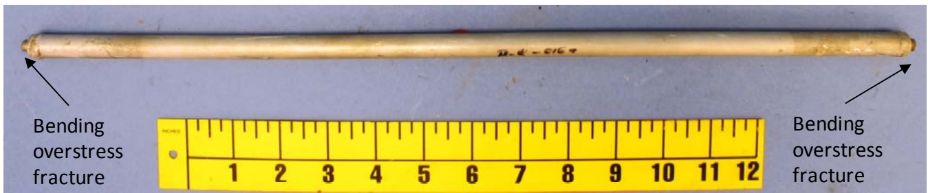
Figure 4 Eighteen-inch long control rod piece showing bending overstress fractures in the threads at each end.
