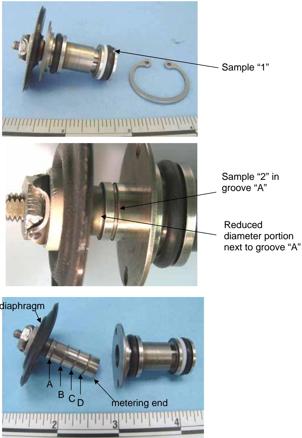
Figure 2. Photographs of the as-received spool portion that was inserted into the sleeve portion (top of page); spool partially removed from the sleeve portion showing a red particle that was attached to balance groove "A" (center of page); spool portion disassembled from the sleeve portion showing grooves labeled A" through "D" (bottom of page).
