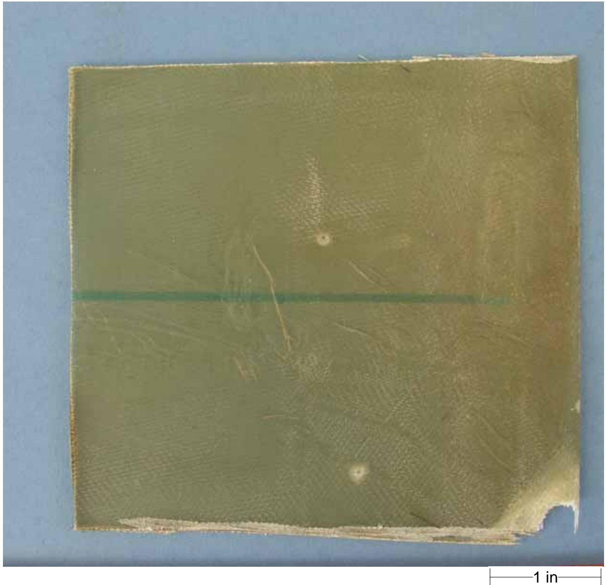
Figure 26. Photograph of the fiberglass wall portion from an exemplar collector can that was submitted by Carson Helicopter Services Incorporated. A piece from the lower right corner was fractured at the Safety Board Materials Laboratory for examination.
