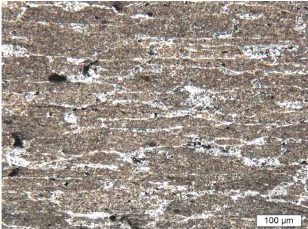
Figure 14. Longitudinal-radial section of the wall portion of the position adjusting screw. The microstructure shows an overheated aluminum alloy. Etched with Keller's reagent.
