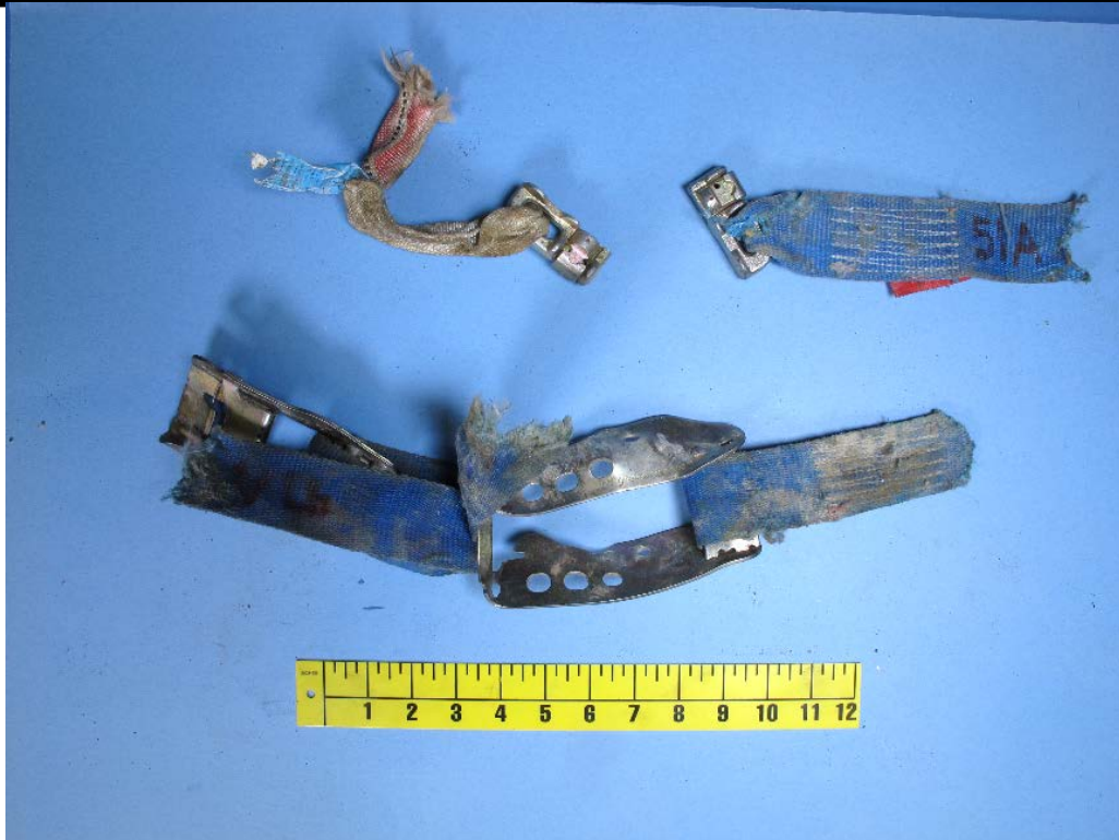
Figure 2. Image 2 of as-received tie-down strap segments.
