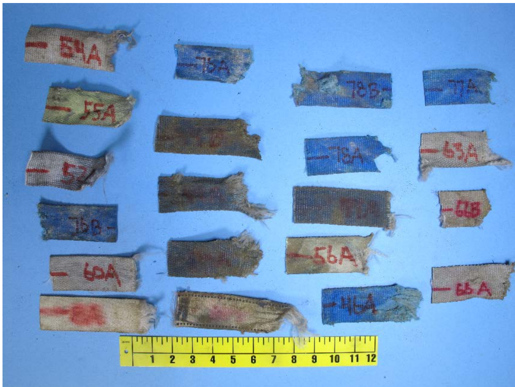
Figure 3. Image 3 of as-received tie-down strap segments.
