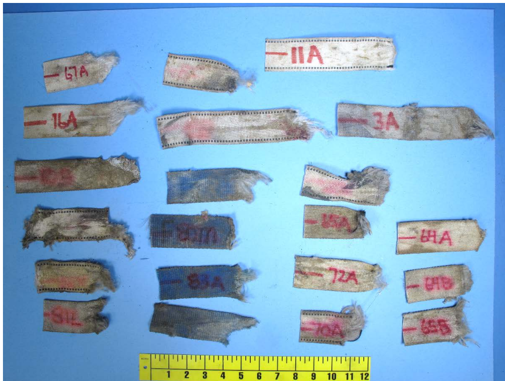
Figure 1. Image 1 of as-received tie-down strap segments.
