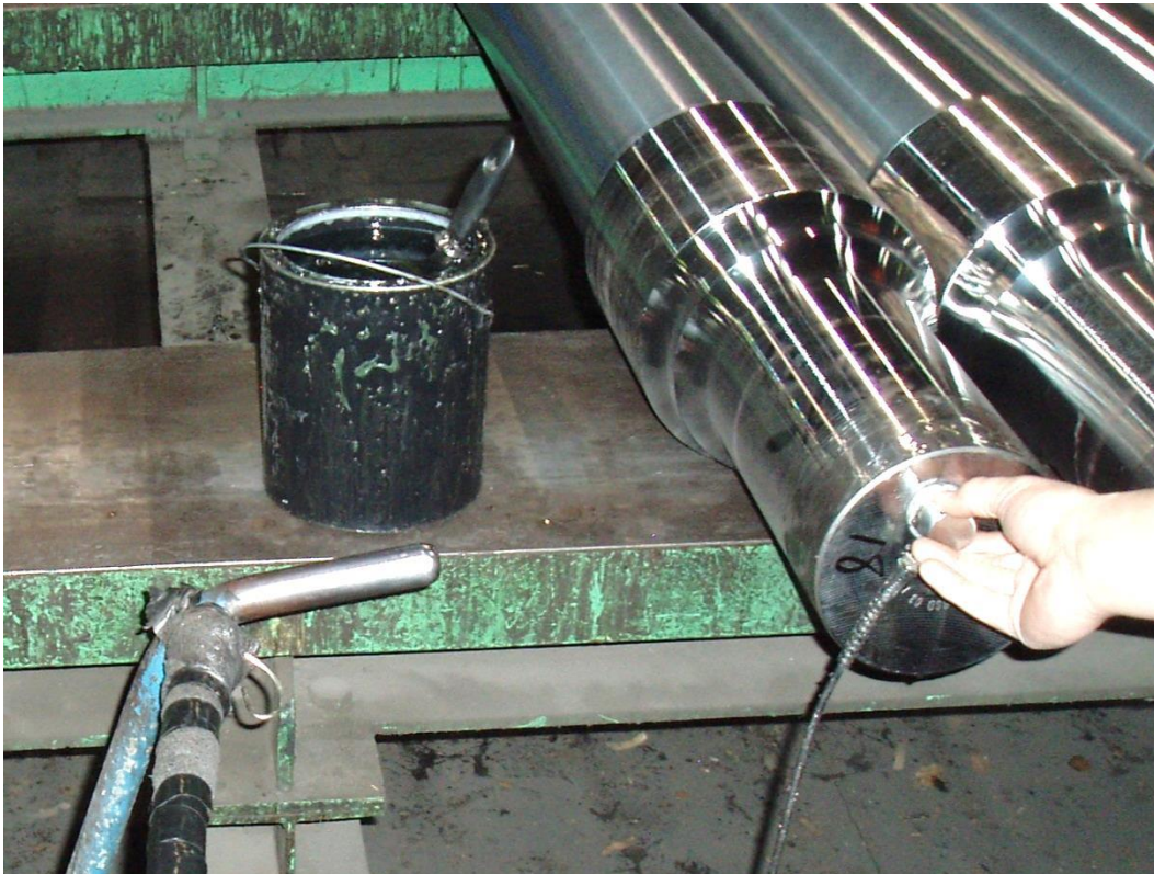
Figure 6 – Axial UT inspection of a finished axle.
