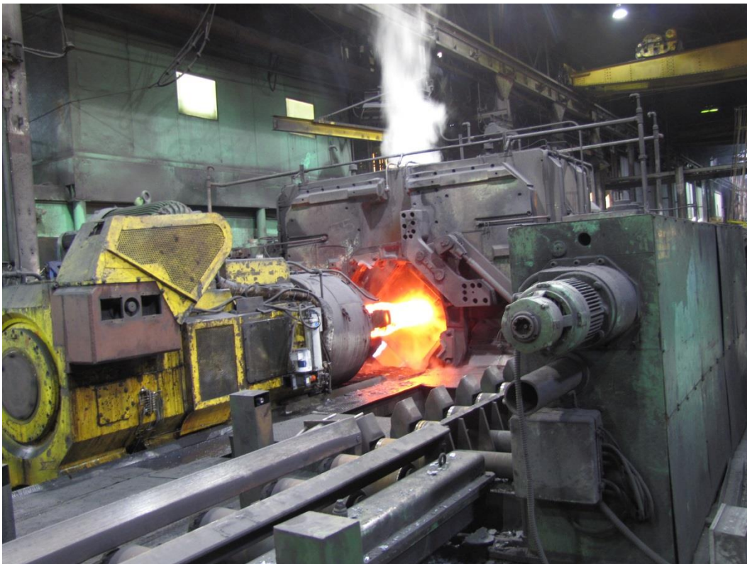
Figure 4 – Radial forging of a heated cut ingot, held by the “A” manipulator.
