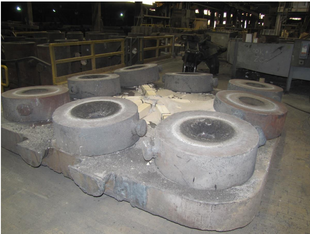
Figure 2 – The bottom of an ingot mold, after teeming and removal of the cylindrical molds.
