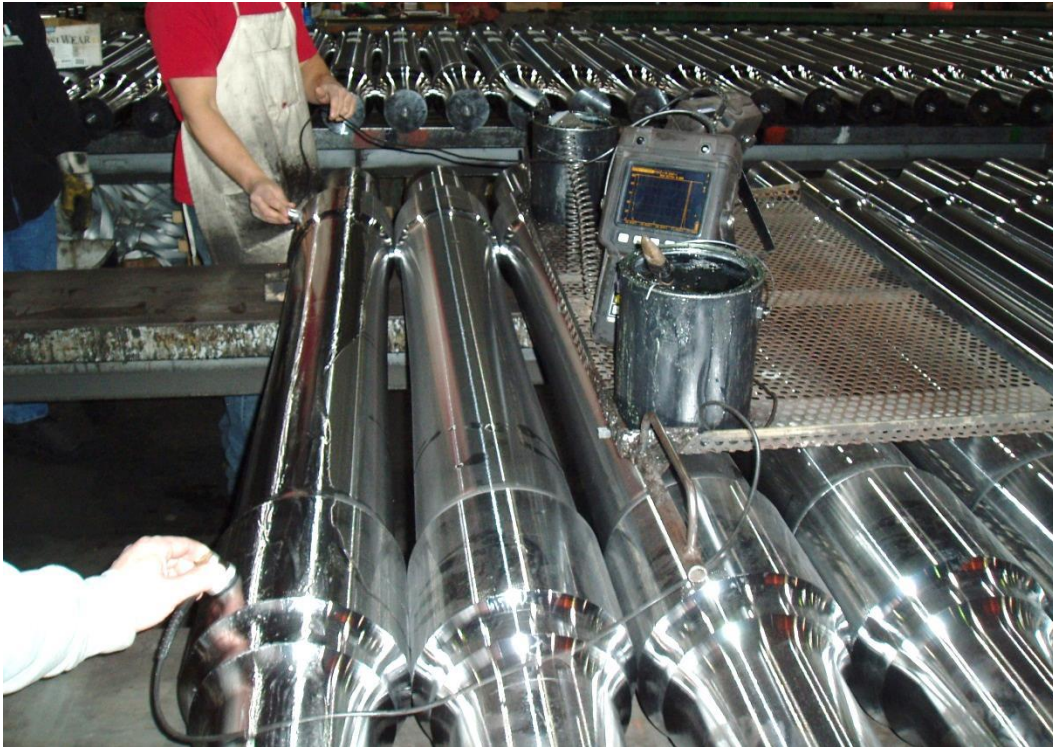
Figure 5 – Radial UT inspection of a finished axle.
