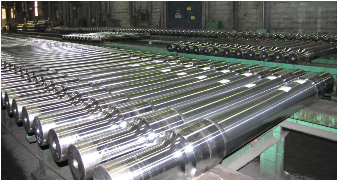
Figure 7 – Finished axles, after inspection identified with bar code labels.
