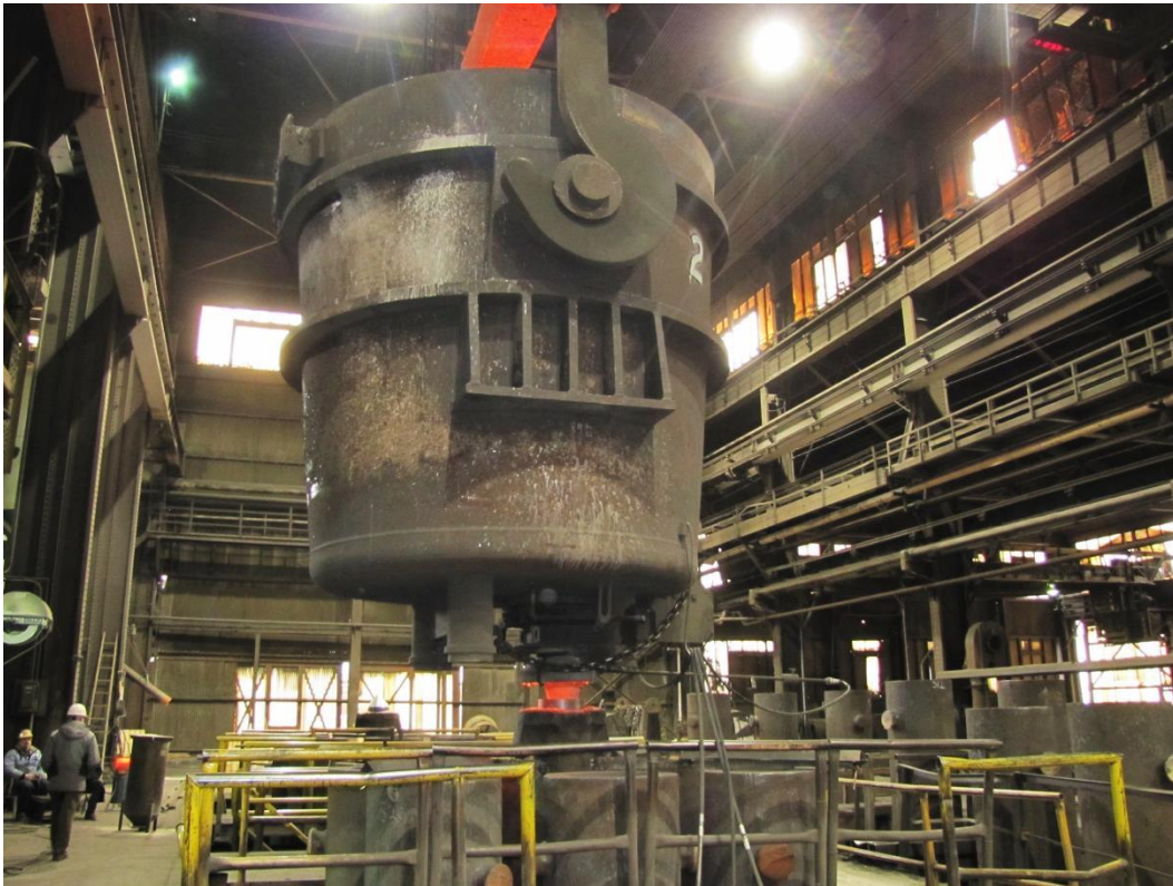
Figure 3 – A ladle positioned over the center trumpet after ingot teeming.
